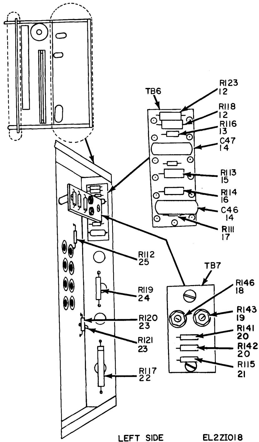
Figure 14. Generator, Pulse AN/UPM-15A, Chassis, Inside, Rear View (Sheet 2 of 2).
