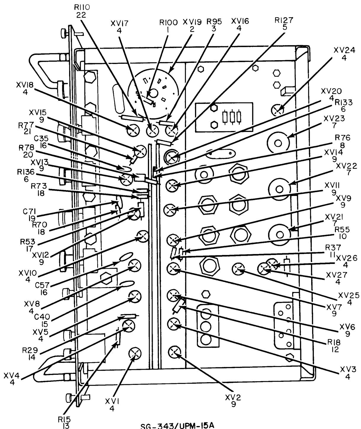
Figure 12. Generator, Pulse AN/UPM-15A, Chassis, Bottom View.
