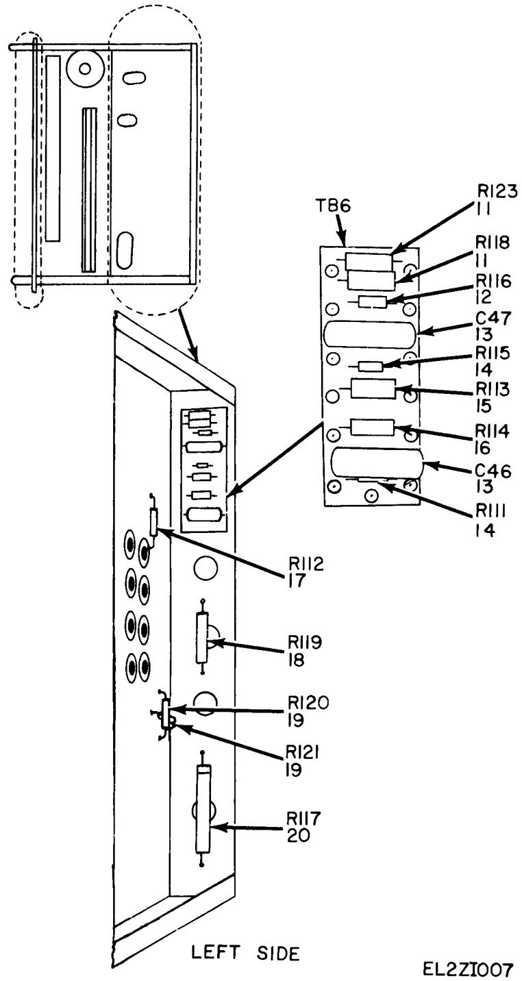
Figure 6. Generator, Pulse AN/UPM-15, Chassis, Inside Rear View (Sheet 2 of 2).
