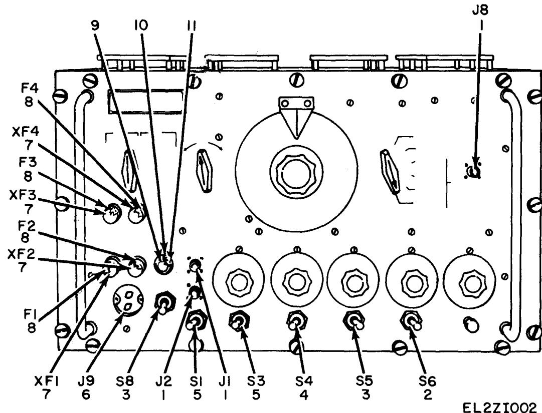
Figure 2. Generator, Pulse AN/UPM-15, Front Panel.
