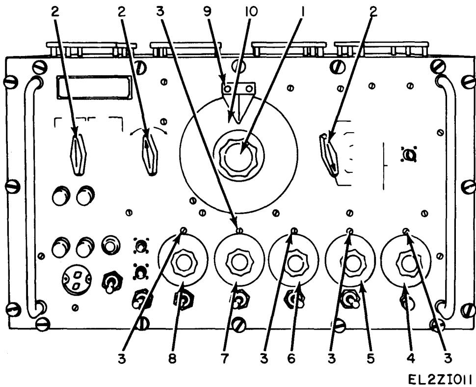
Figure 8. Generator, Pulse AN/UPM-15, Operating Controls.
