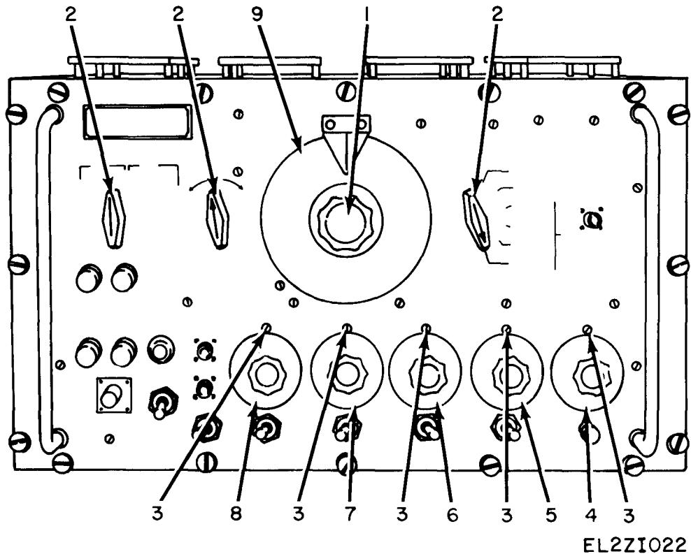
Figure 16. Generator, Pulse AN/UPM-15A, Operating Controls.
