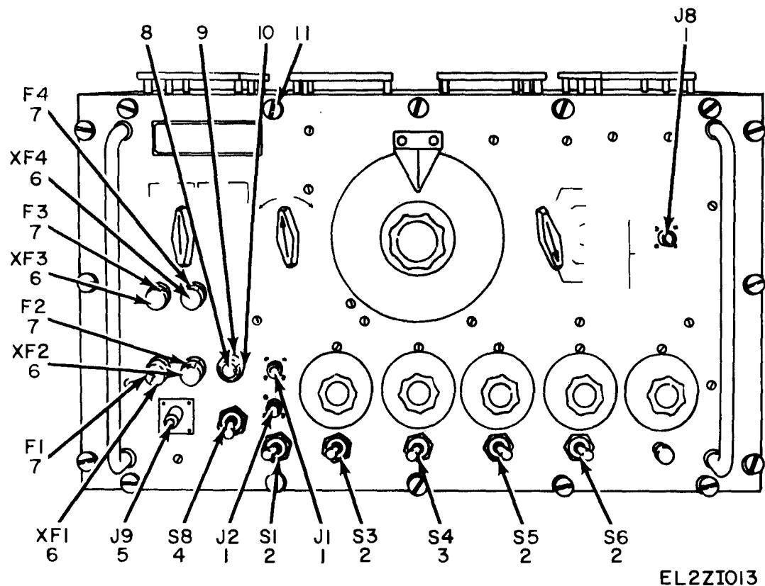
Figure 10. Generator, Pulse AN/UPM-15A, Front Panel.
