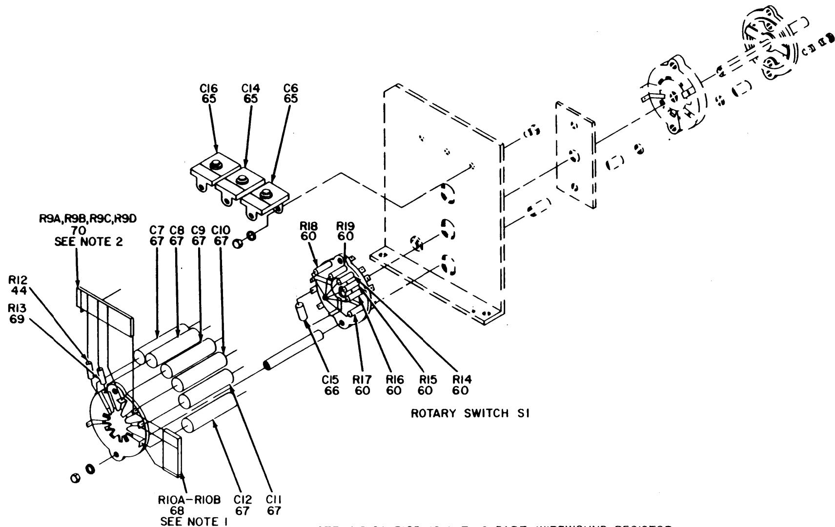
Figure 3. Voltmeter, Meter ME-30( )/U, ME-30C/U (Sheet 5 of 6).
