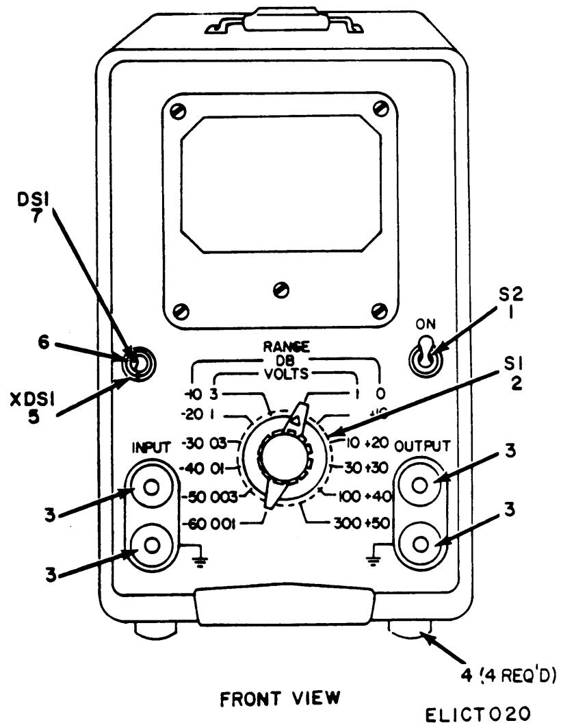
Figure 4. Voltmeter, Meter ME-30( )/U, ME-30E/U (Sheet 1 of 6)
