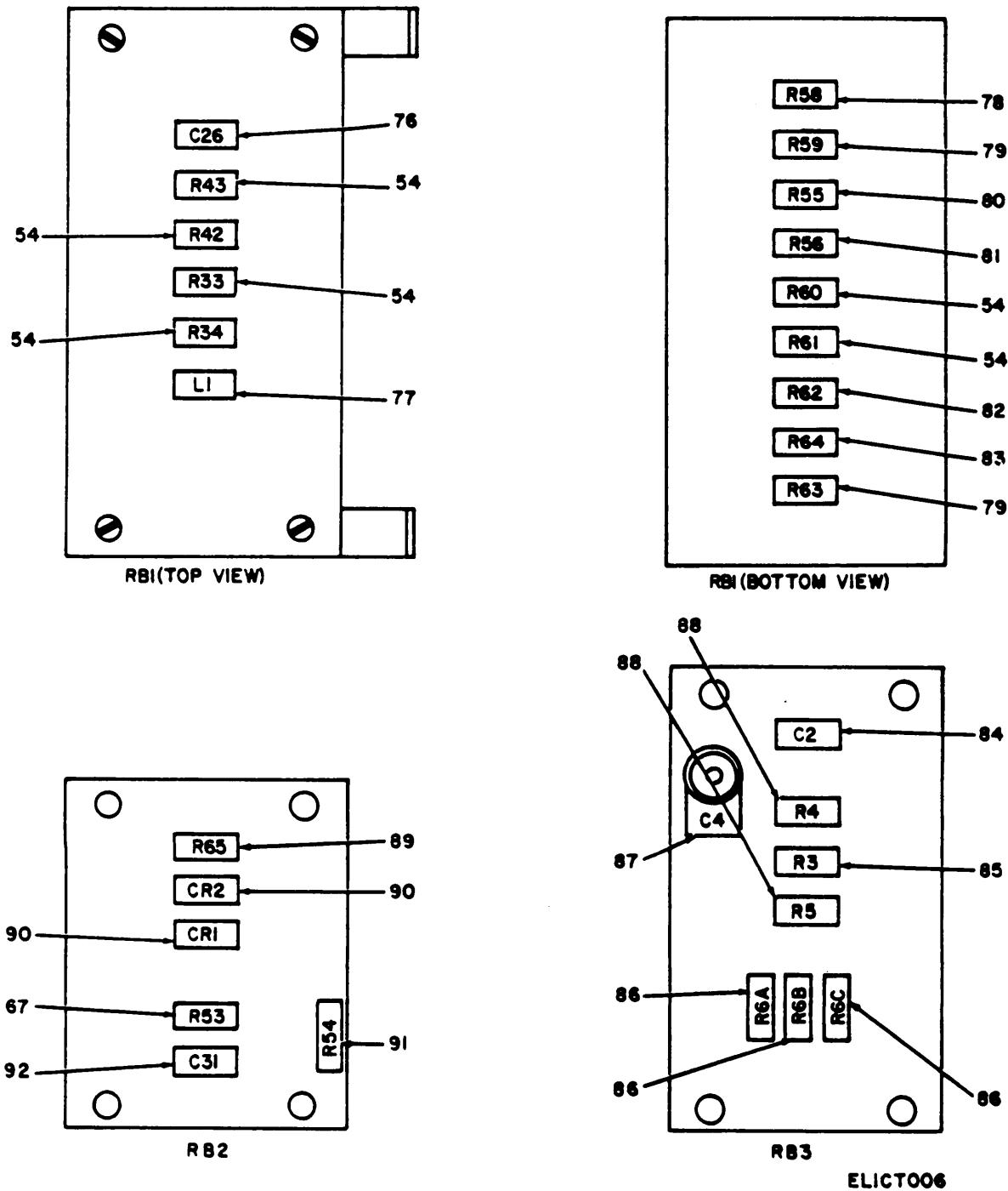
Figure 1. Voltmeter, Meter ME-30( )/U, ME-30A/U (Sheet 6 of 6)
