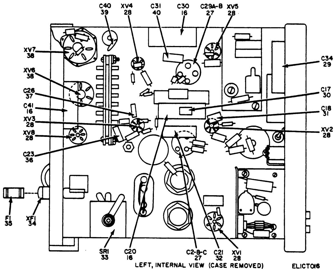
Figure 3. Voltmeter, Meter ME-30( )/U, ME-30C/U (Sheet 3 of 6)
