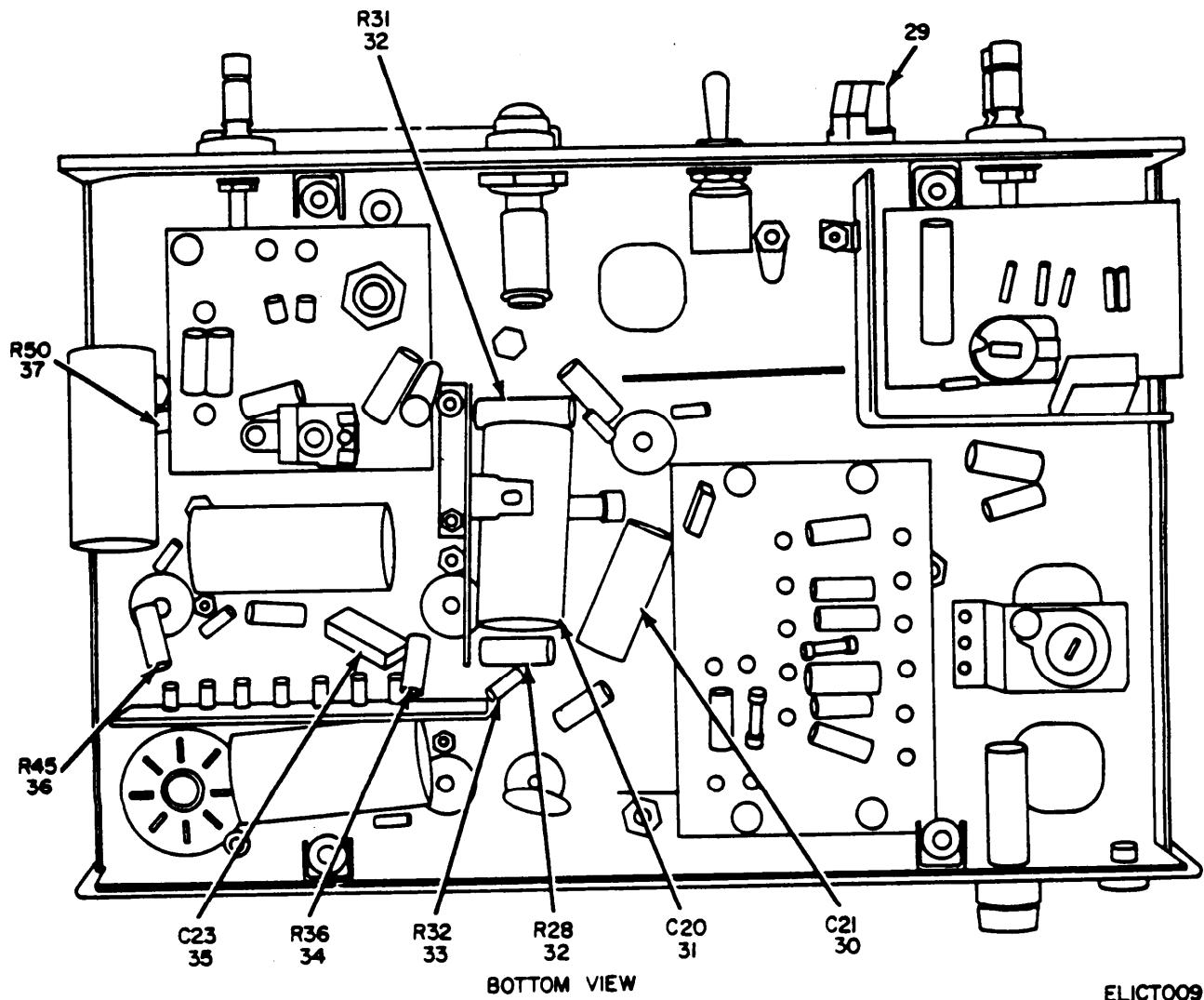
Figure 2. Voltmeter, Meter ME-30( )/U, ME-30B/U (Sheet 3 of 7)
