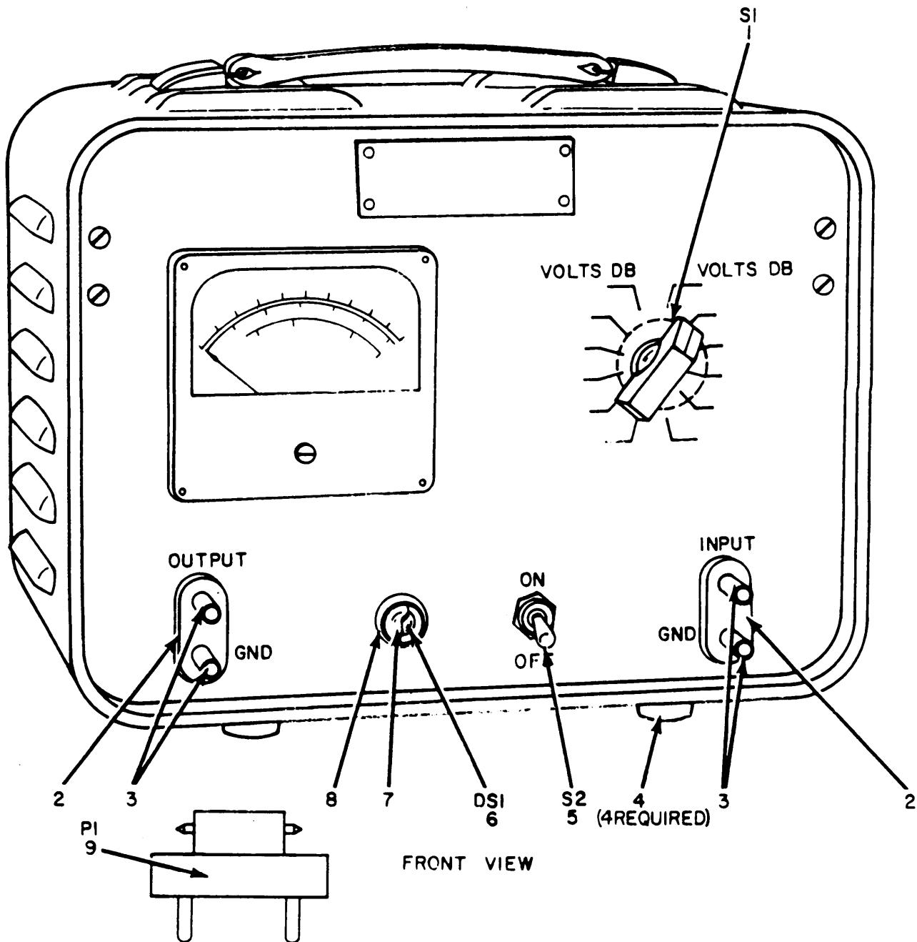
Figure 2. Voltmeter, Meter ME-30( )/U, ME-30B/U (Sheet 1 of 7).
