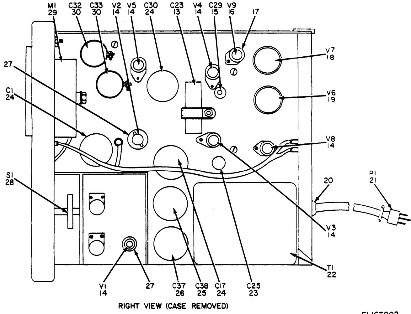
Figure 1. Voltmeter, Meter ME-30( )/U, ME-30A/U (Sheet 2 of 6)
