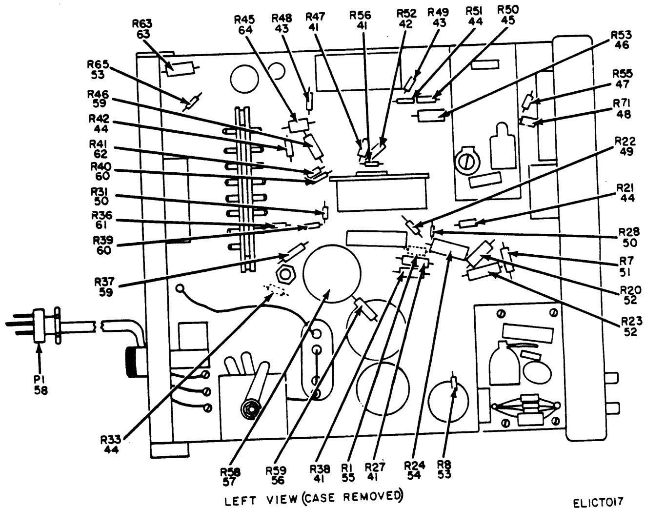
Figure 3. Voltmeter, Meter ME-30( )/U, ME-30C/U (Sheet 4 of 6).
