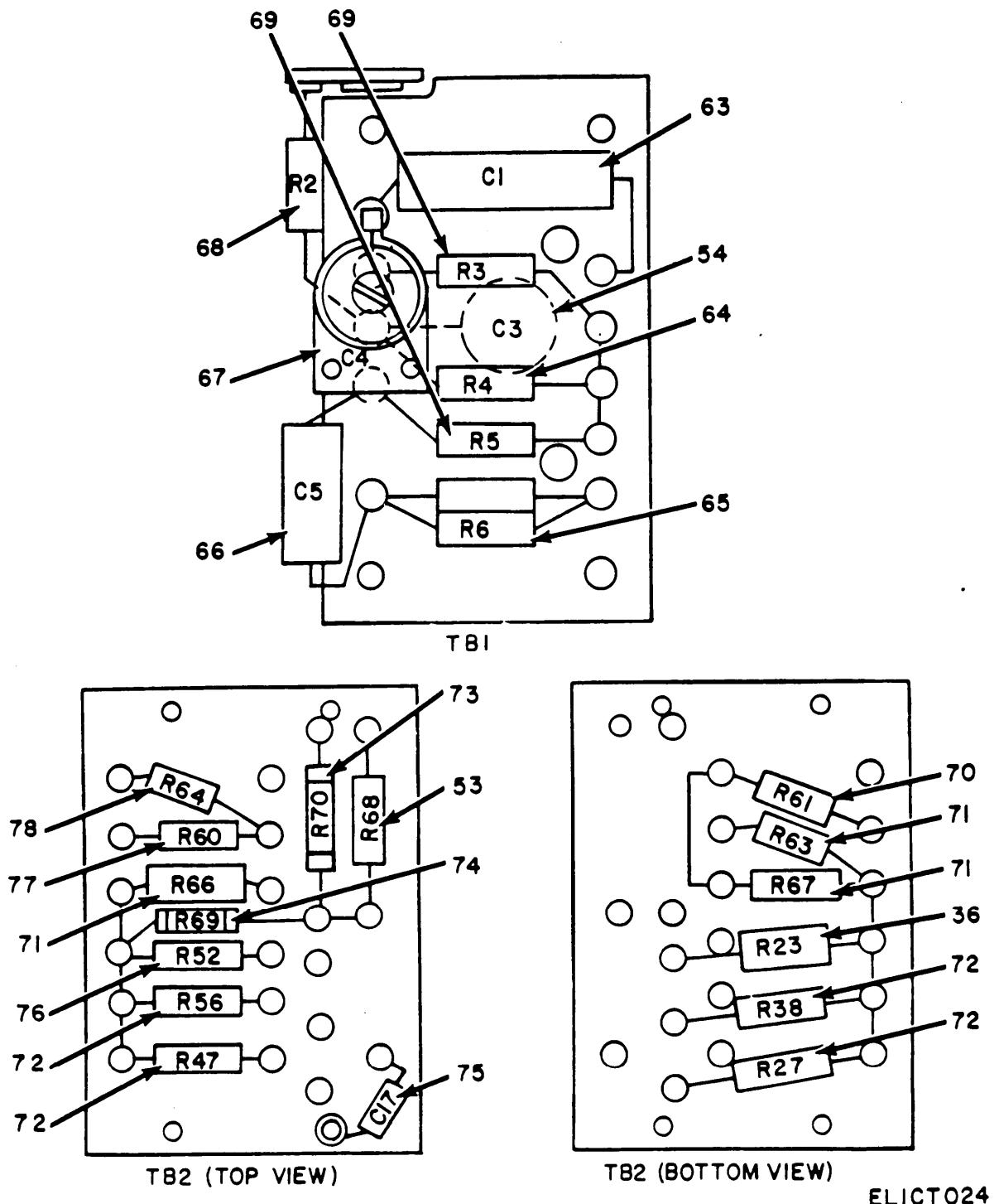
Figure 4. Voltmeter, Meter ME-30( )/U, ME-30E/U (Sheet 5 of 6).
