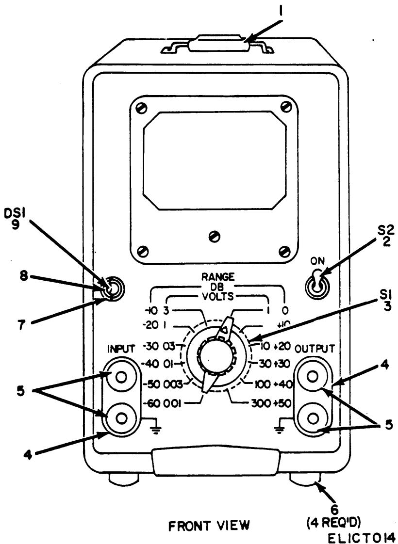
Figure 3. Voltmeter, Meter ME-30( )/U, ME-30C/U (Sheet 1 of 6)
