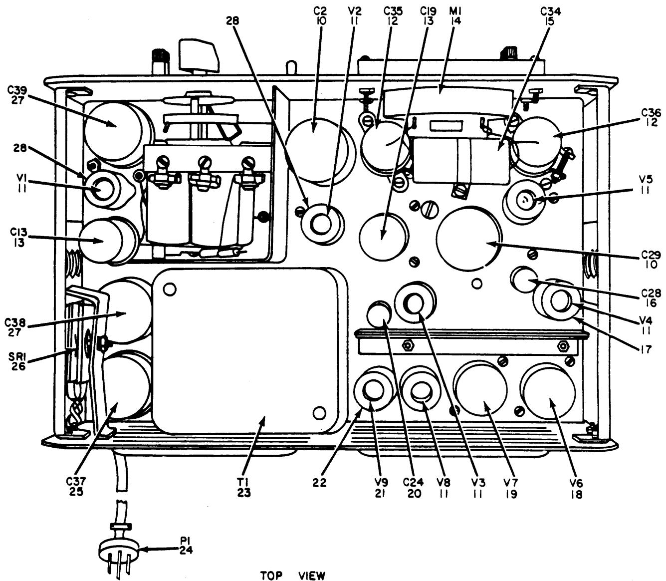
Figure 2. Voltmeter, Meter ME-30( )/U, ME-30B/U (Sheet 2 of 7).
