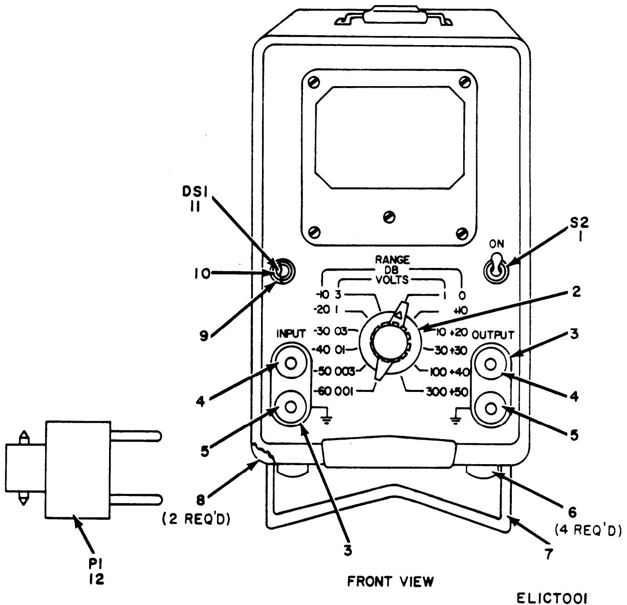
Figure 1. Voltmeter, Meter ME-30( )/U, ME-30A/U (Sheet 1 of 6).
