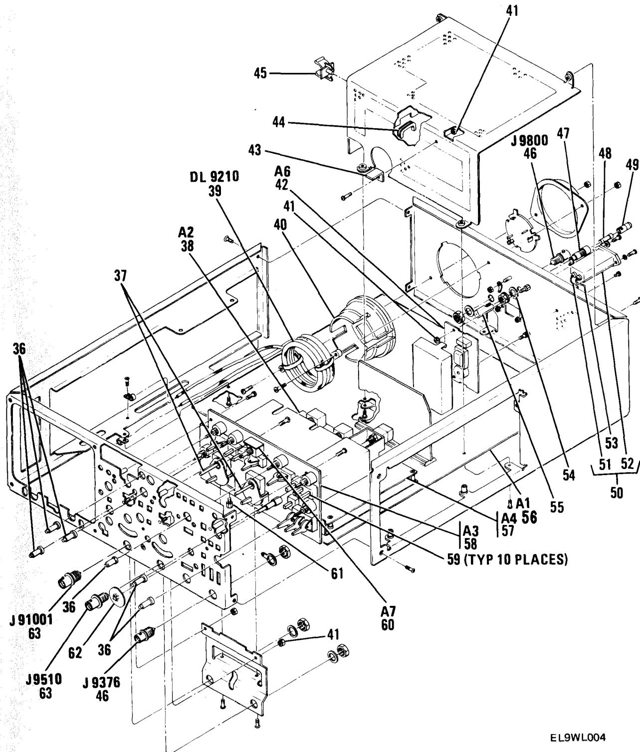
Figure 1. Oscilloscope AN/USM-488 Exploded View (Sheet 3 of 4)
