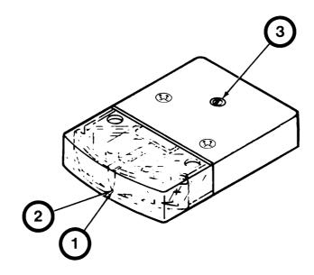
b. Connect power cable (1) to power input connector (2). Push in power switch (3). The power switch button should remain in and one of the decimal points should glow.
