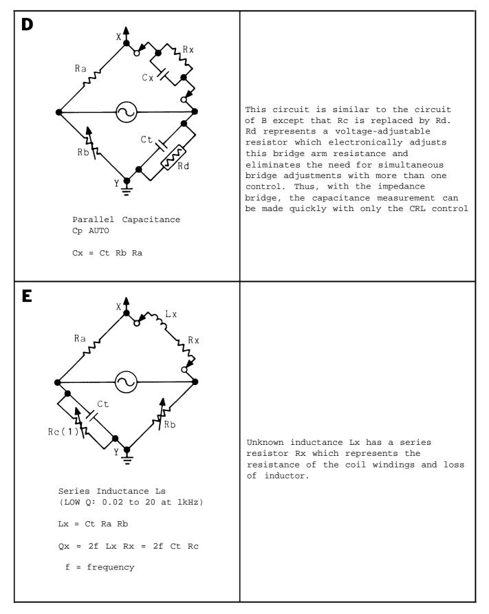
Figure 4-1. Bridge circuit configuration (Sheet 3 of 4).
