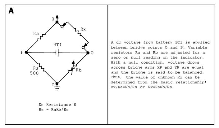
Figure 4-1. Bridge circuit configuration (Sheet 1 of 4).
