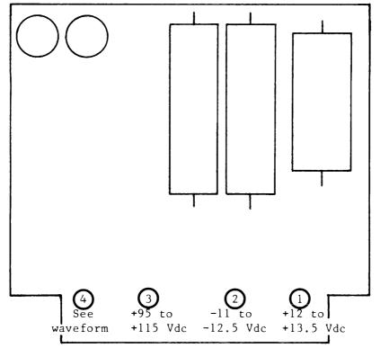
c. The following are correct test voltages and waveforms for the reference voltage assembly (A300), from the test point (TP) numbers:
