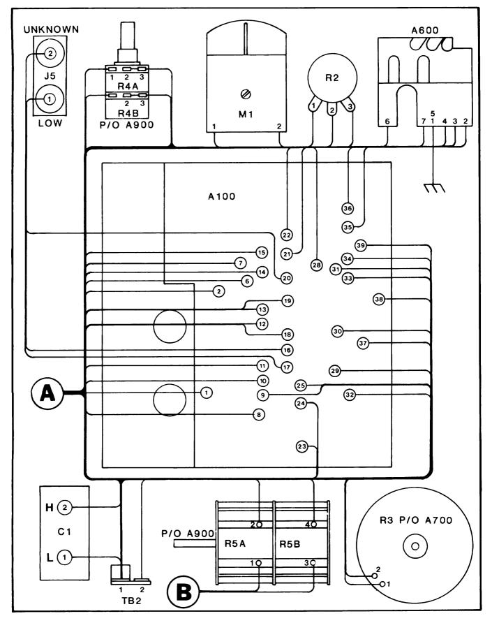
Figure 4-2. Impedance Bridge Wiring Diagram (Sheet 1 of 2).
