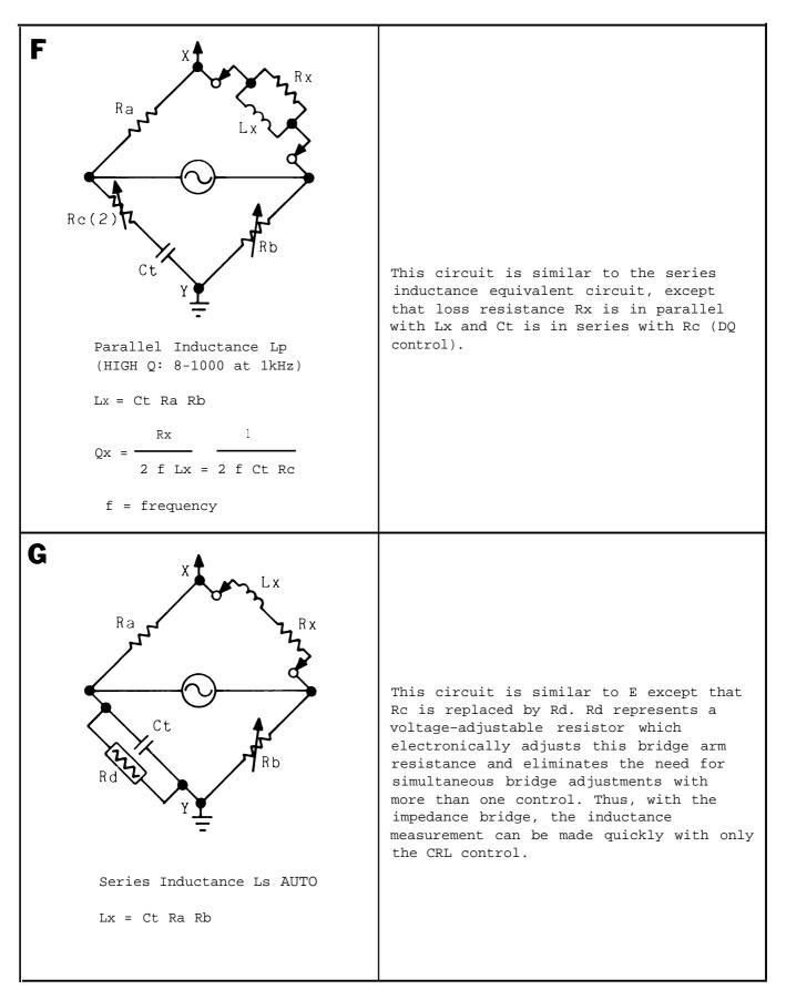
Figure 4-1. Bridge circuit configuration (Sheet 4 of 4).
