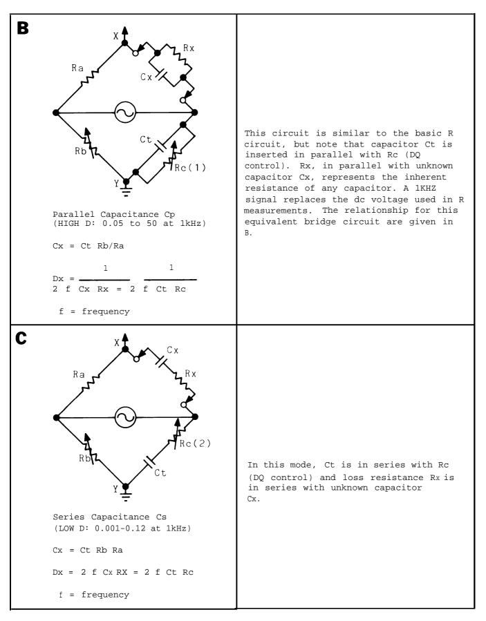
Figure 4-1. Bridge circuit configuration (Sheet 2 of 4).
