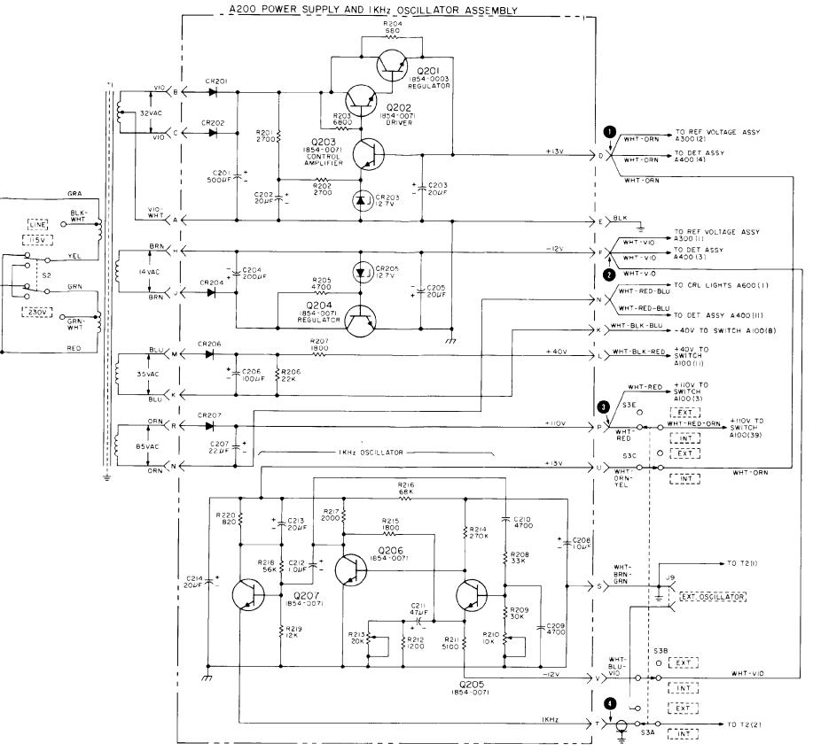
Power Supply and lKHz Oscillator Schematic Diagram FOLDOUT FO-3
