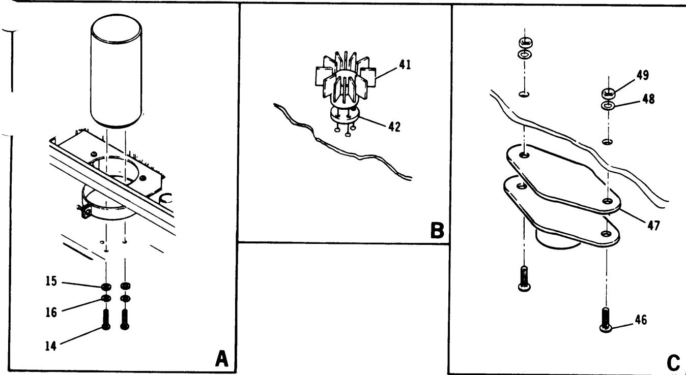
Figure 5. Main PCB Assembly (Sheet 3 of 4).
