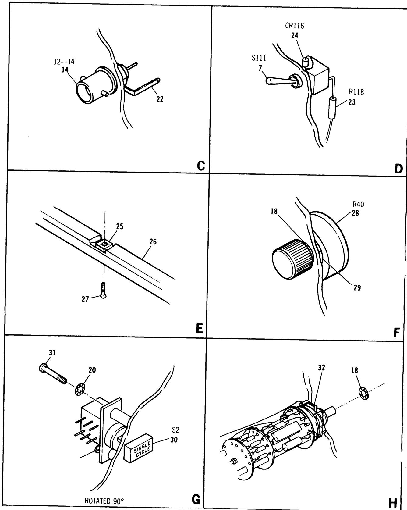
Figure 2. Front Panel Assembly (Sheet 2 of 2).
