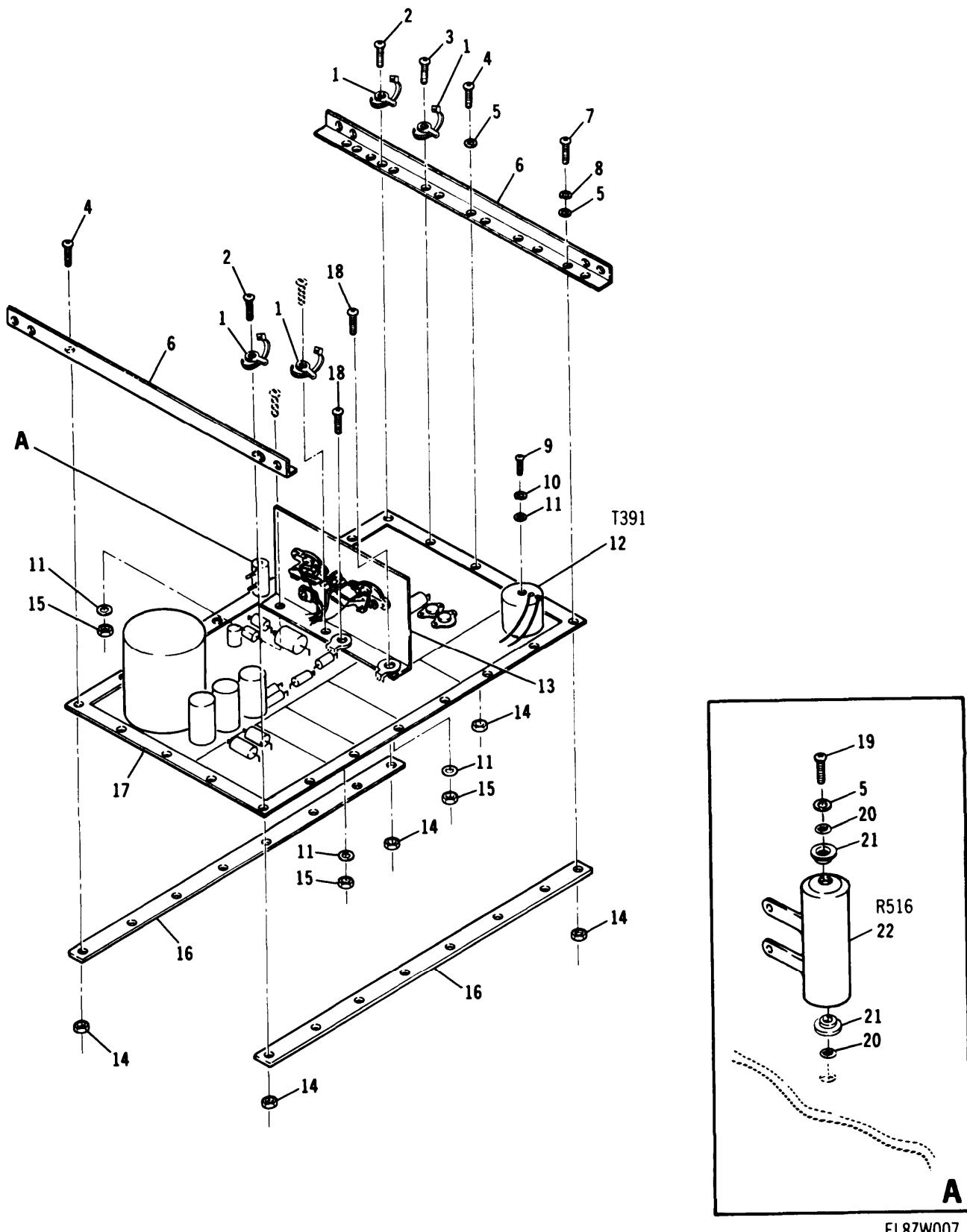
Figure 4. Chassis Subassembly.
