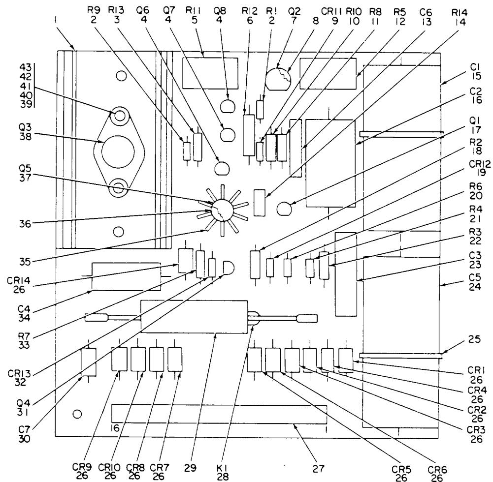
Figure 23. -25 +15 Volt Power Supply A5A1
