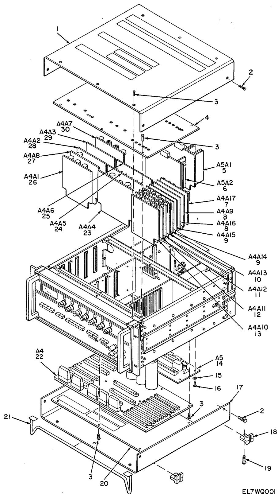
*Figure 1. Calibrator, Direct Current 0-1805/USM (Sheet 1 of 4).*
