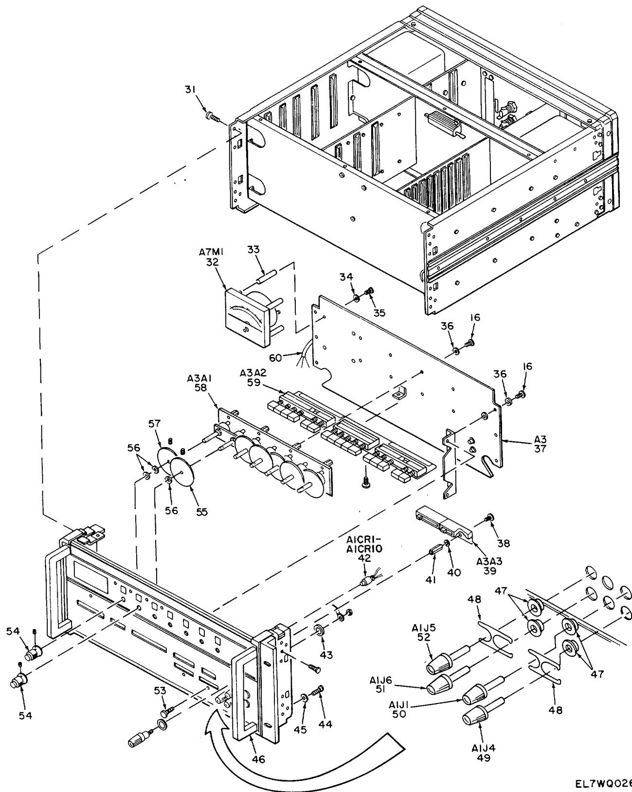
Figure 1. Calibrator, Direct Current 0-1805/USM (Sheet 2 of 4).
