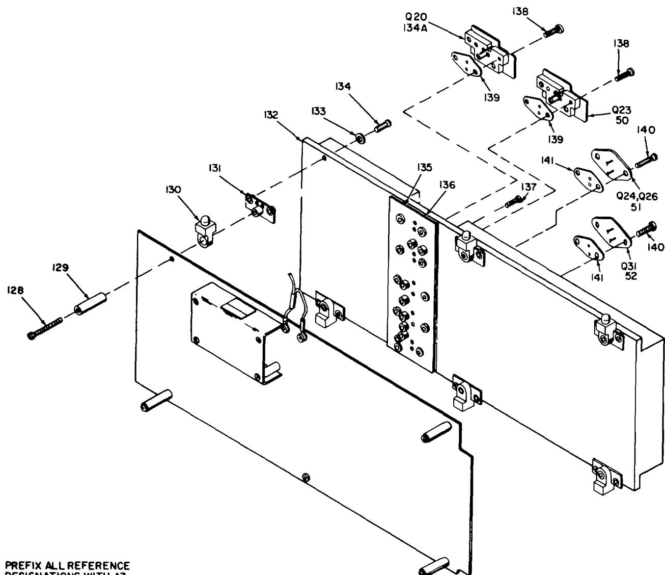
Figure 9. Power Amplifier Assembly A7 (Sheet 2 of 2).
