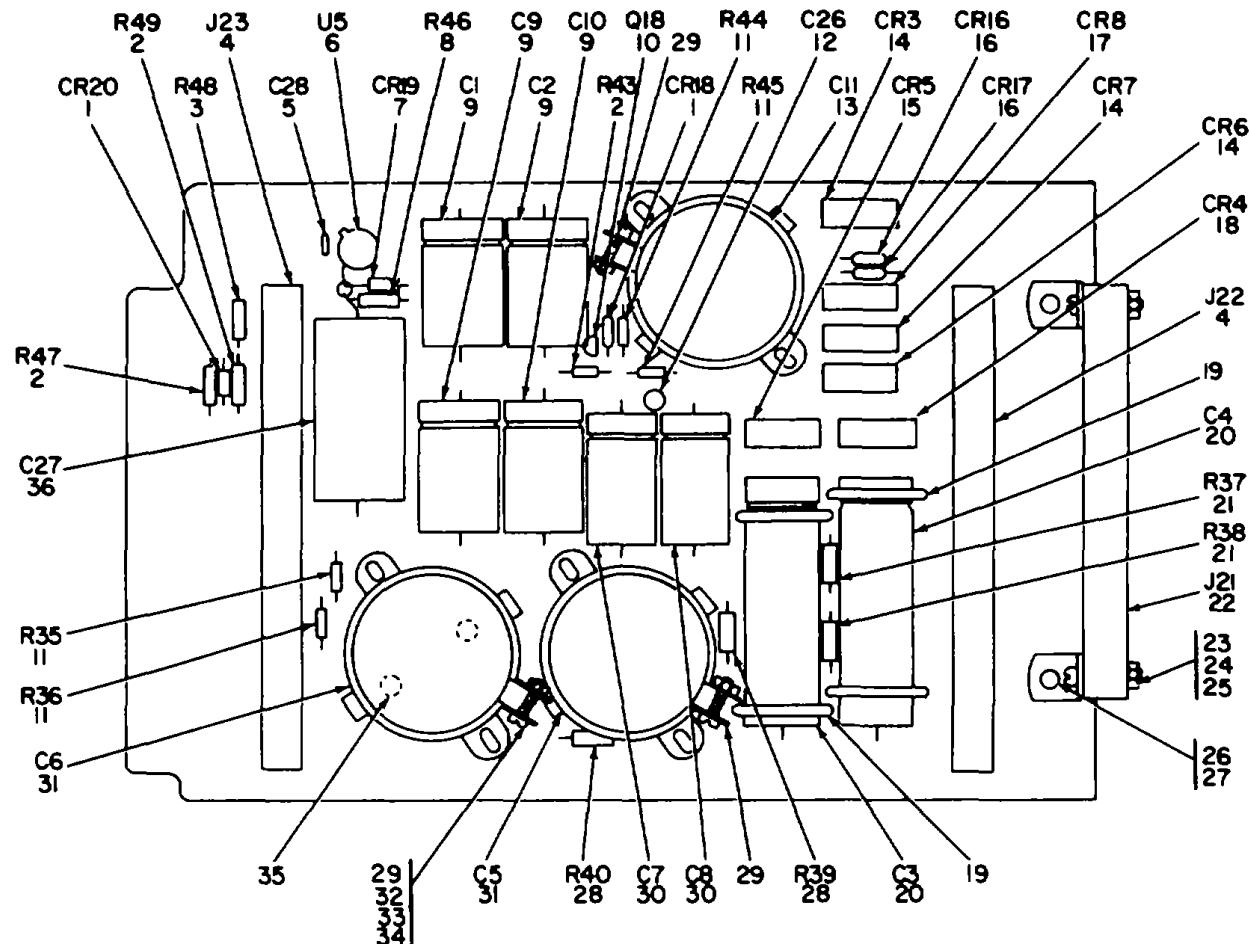
Figure 4. Power Supply Assembly A5.
