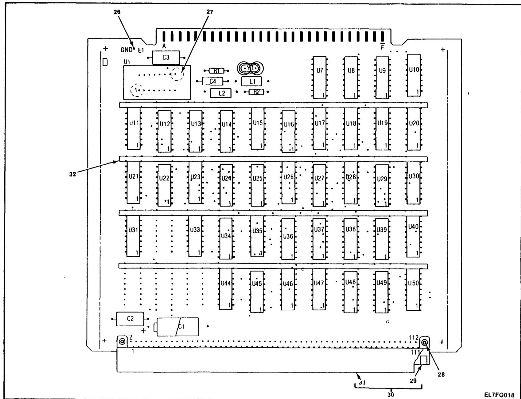
Figure 7. Circuit Card Assembly Pulse Generator (Sheet 1 of 2)
