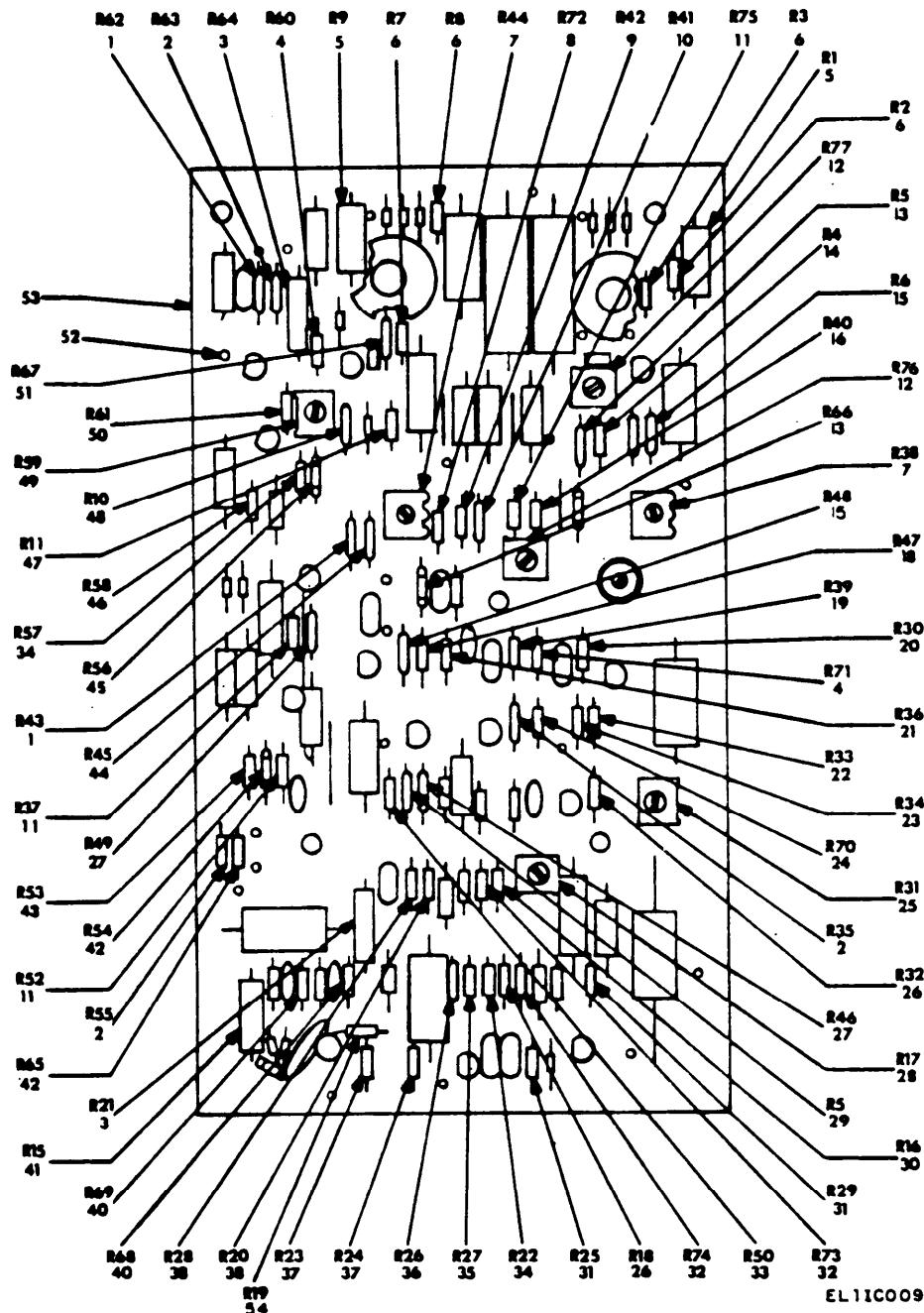
Figure 9. Circuit card assembly (main) (resistors).
