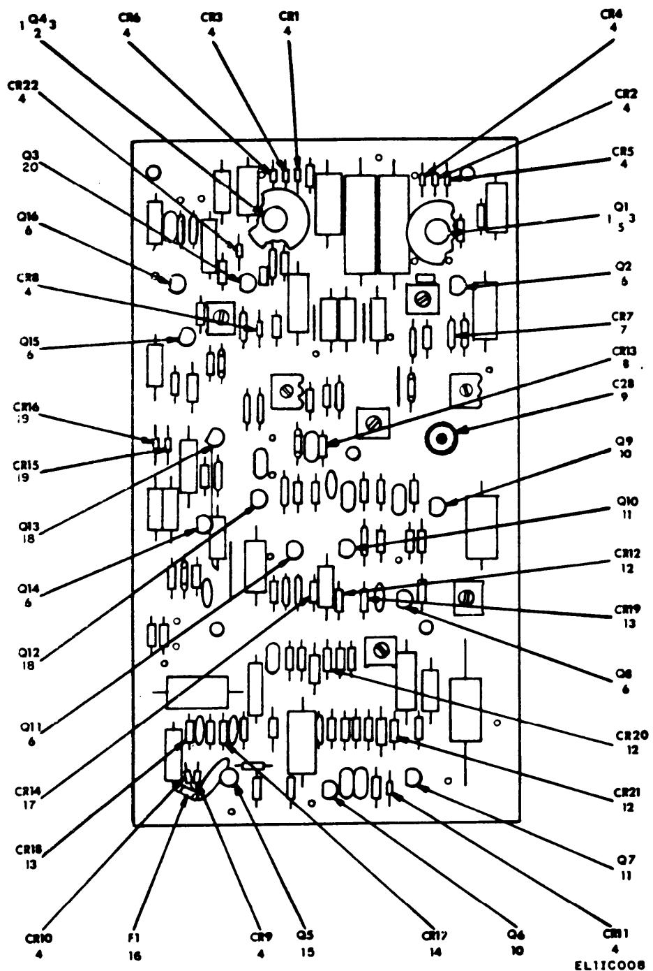
Figure 8. Circuit card assembly (main) (semiconductor).
