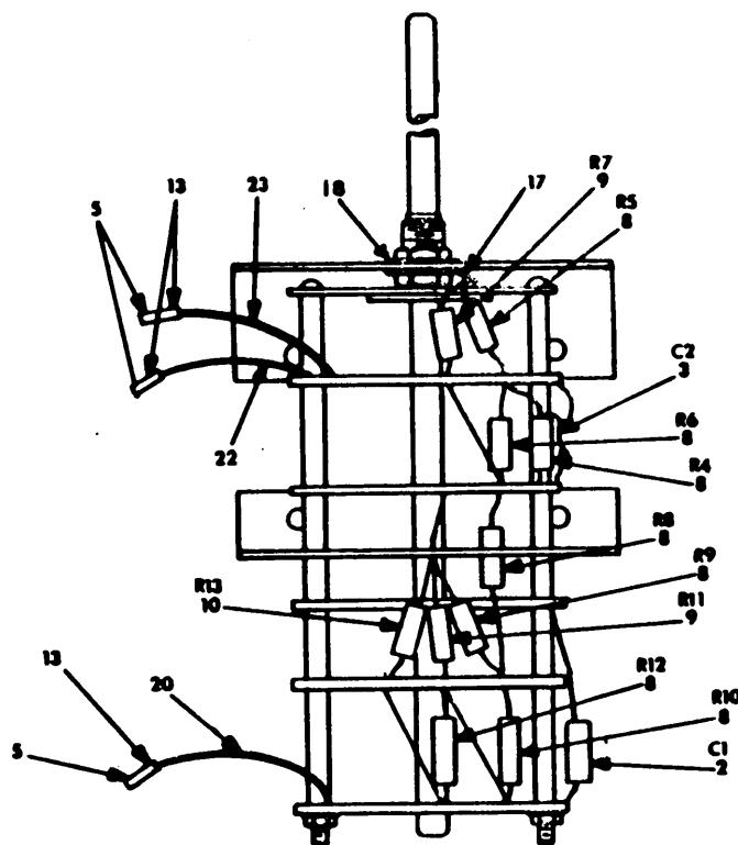
Figure 10. Attenuator assembly.
