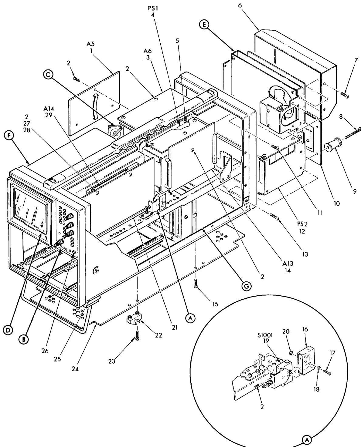
FIGURE 2 -1 , OSCILLOSCOPE OS-262/P/U /SHEET 1 OF 6/
