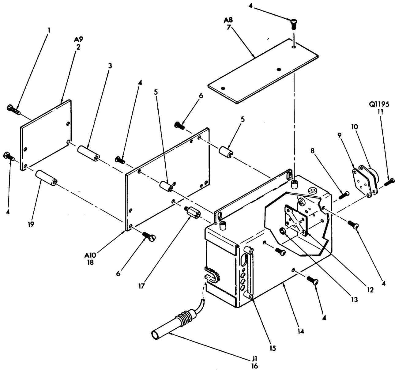
FIGURE 2-12. HIGH VOLTAGE POWER SUPPLY/PS1/
