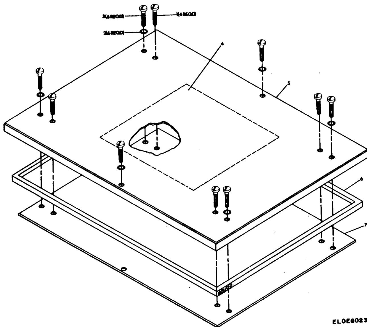
Figure 22. Cover Assembly (P/O A8).
