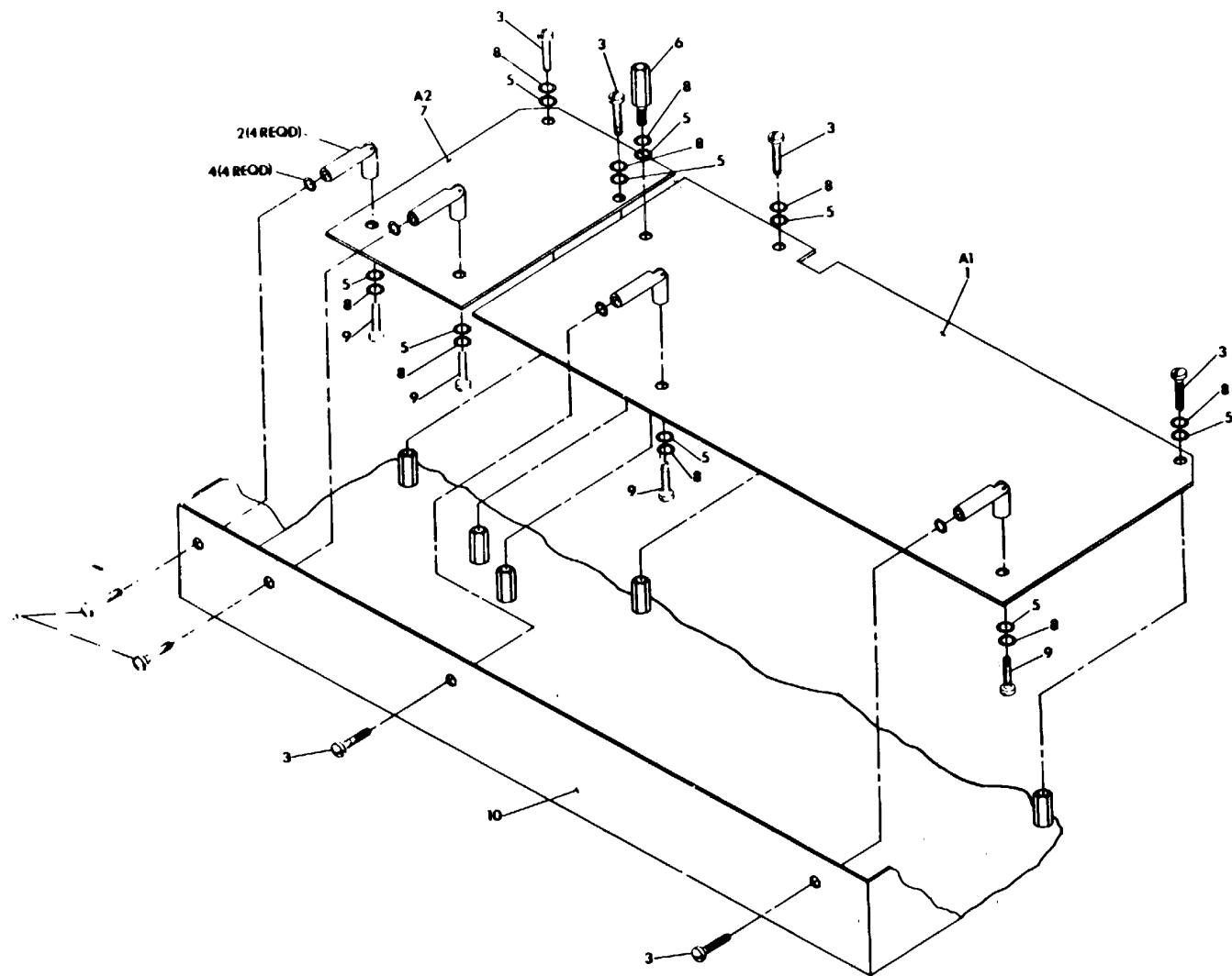
Figure 12. Circuit Card Hinge Assembly (P/O A9).
