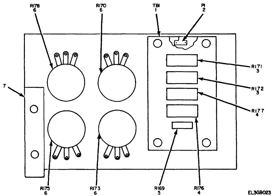
Figure 21. Resistor Board Assembly A2WI1A1.
