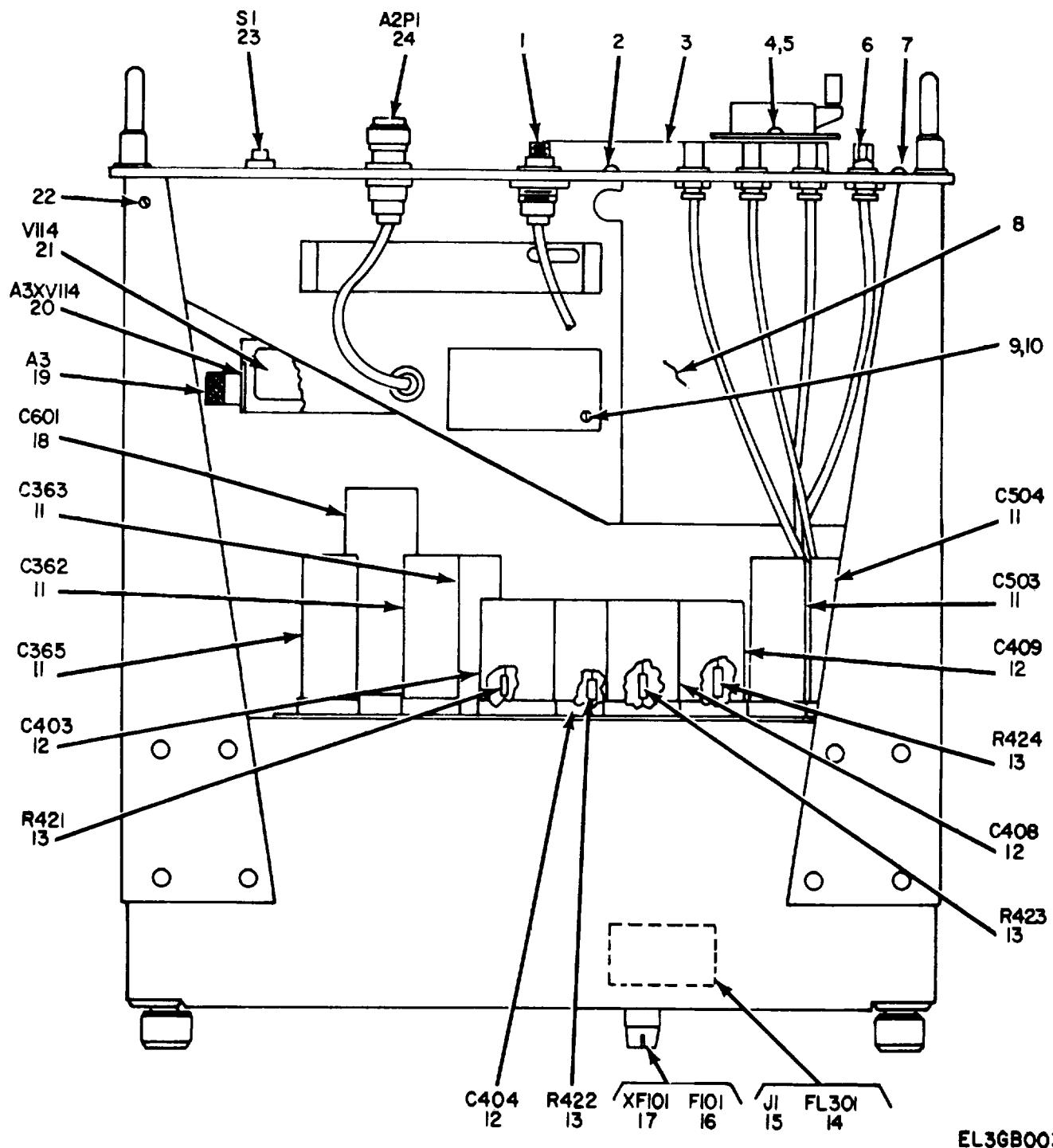
Figure 3. Signal Generator SG-756/URM, Bottom View, Cover Removed .
