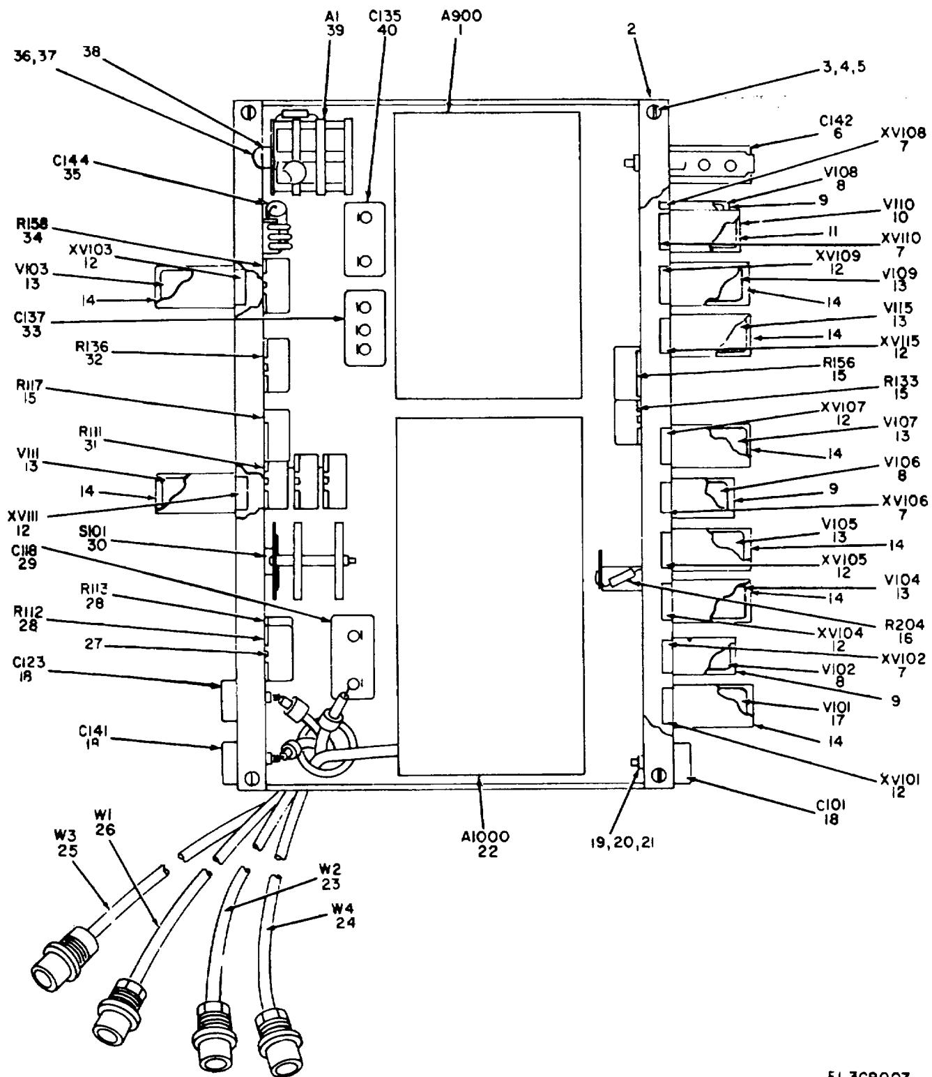
Figure 7. Pulser Assembly A1 .
