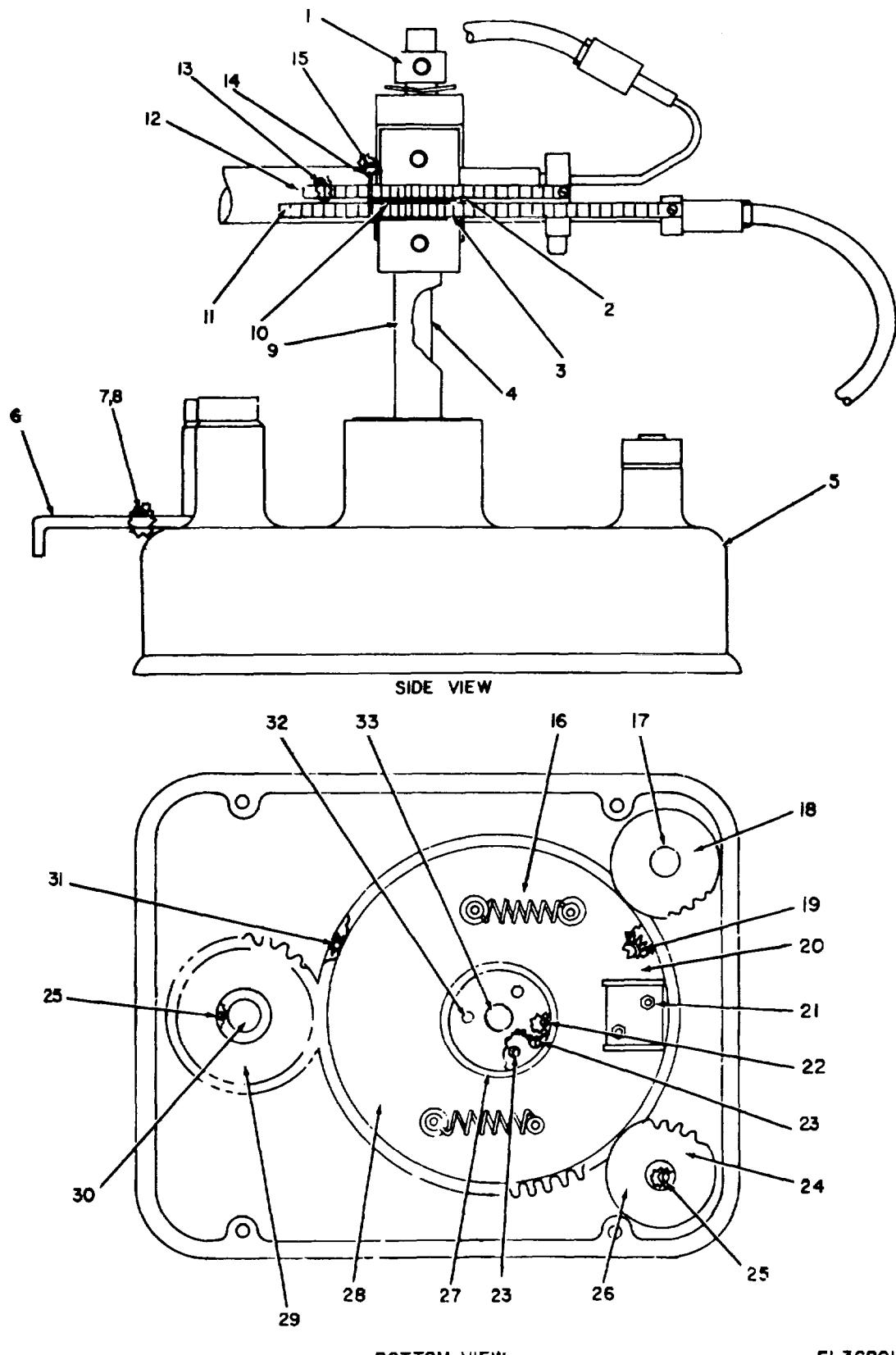
Figure 15. Drive Assembly A2A1 .
