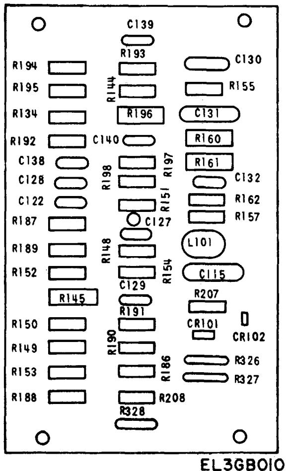
Figure 10. Circuit Card Assembly A1A900 (Sheet 1 of 2).
