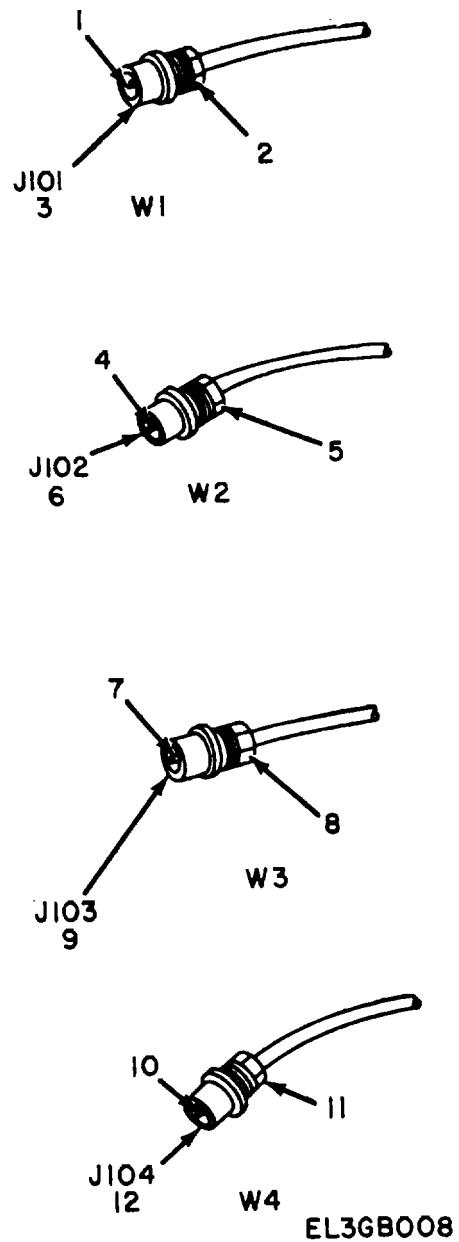
Figure 8. Cable Assemblies, Radio Frequency A1W1 Thru A1W4 .
