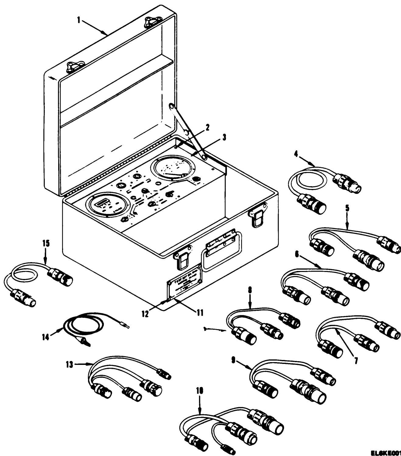
Figure 1. Test Set, Gyro Magnetic Compass AN/ASM-61
