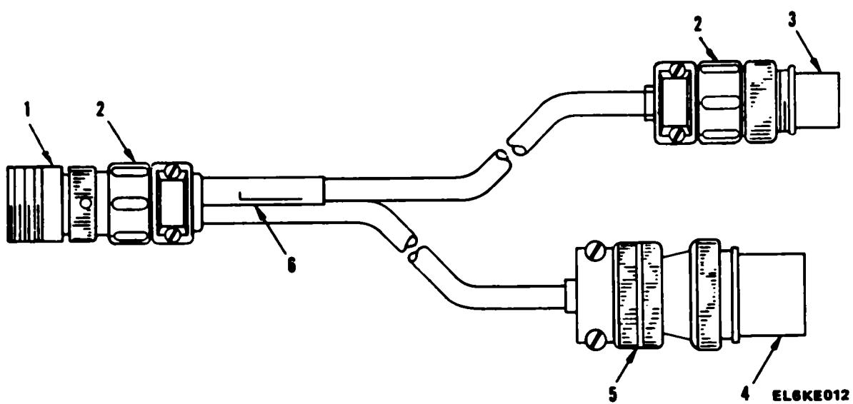
Figure 12. Electrical Lead Assembly CX- 11167/ASM-61
