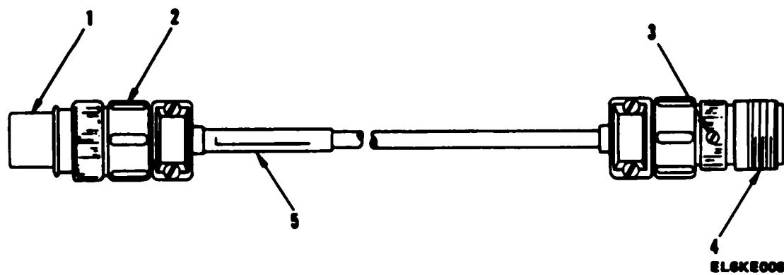
Figure 6. Special Cable Assembly, CX-11161/U
