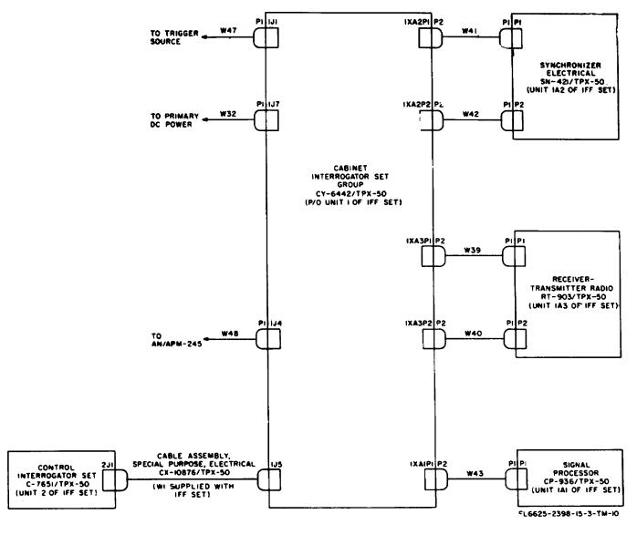
Figure 3-3. Connections of test cables to the IFF set.
