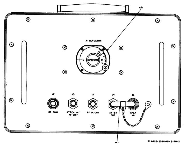
Figure 3-1. Hybrid attenuator A1, operating control, connectors and cable.
