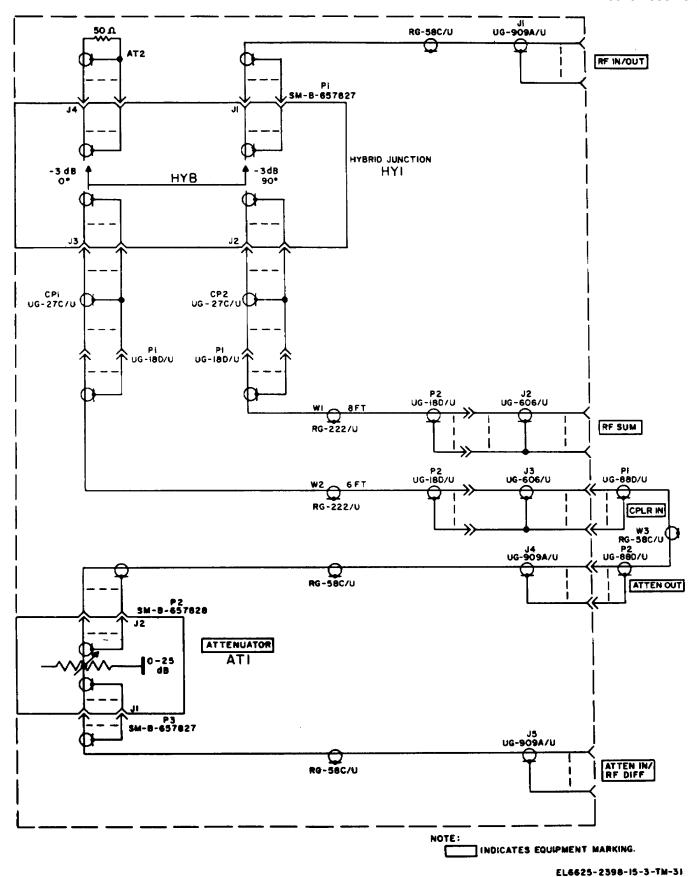
Figure 6-19. Hybrid Attenuator Assembly CN-1322/TPM-24(V), schematic diagram.
