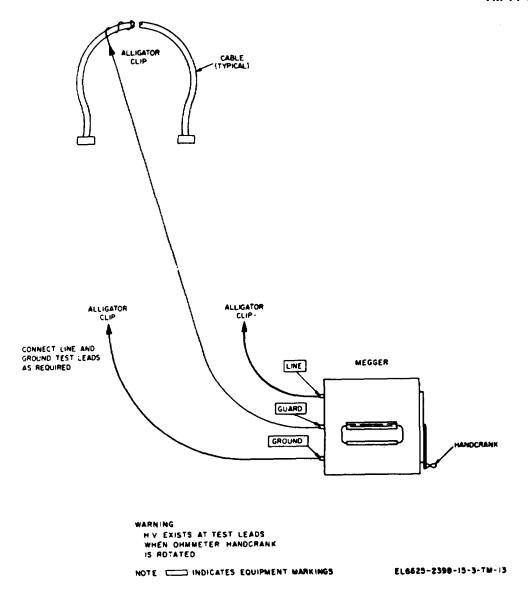
Figure 6-1. Cable megger test connections.
