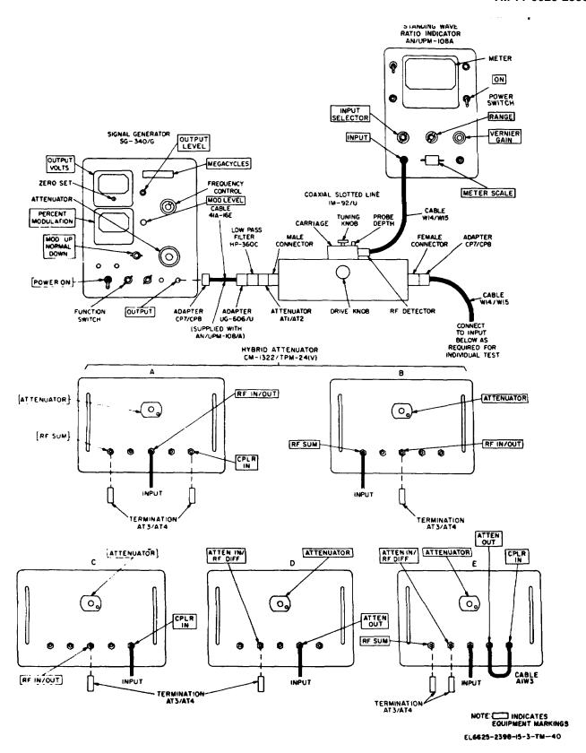
Figure 8-6. Hybrid Attenuator VSWR, test connections.
