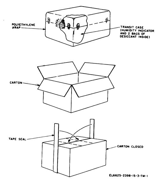
Figure 2-1. Packaging of Test Facilities Set AN/TPM-24(V)3.
