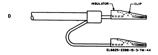
Figure 7-4. Assembly of alligator clips on cable W16.
