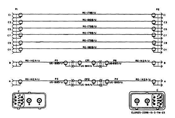
Figure 6-11. Cable W39, schematic diagram.
