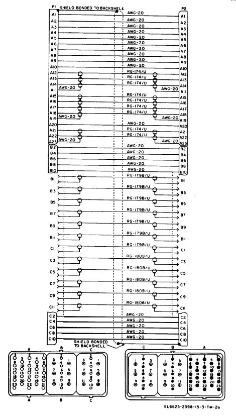
Figure 6-14. Cable W42, schematic diagram.
