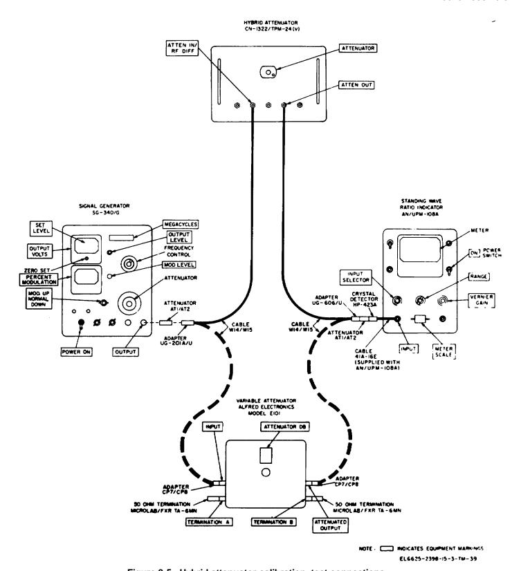
Figure 8-5. Hybrid attenuator calibration, test connections.
