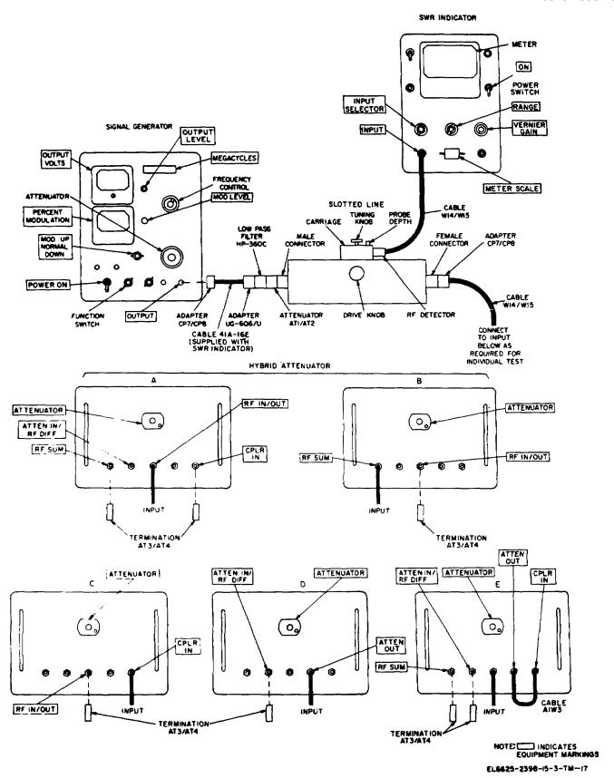
Figure 6-5. Hybrid attentuator VSWR, test connections
