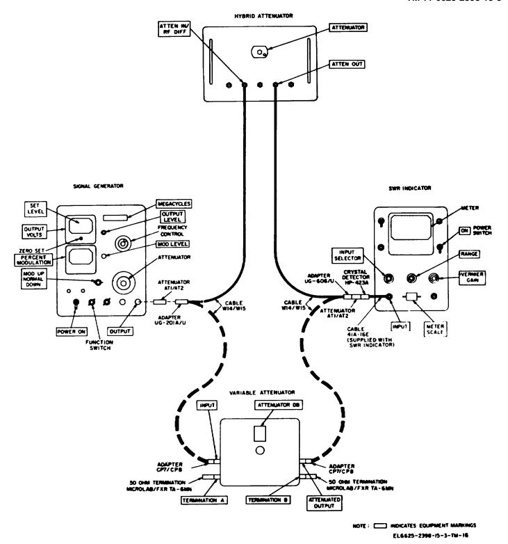
Figure 6-4. Hybrid attenuator ATTENUATOR dial, calibration connections.
