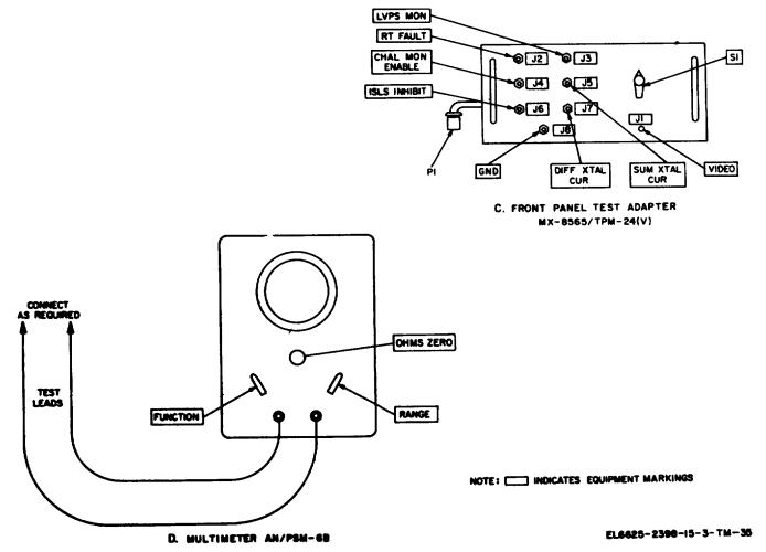
Figure 8-1. Cables, front panel test adapter and extender boards, continuity test conditions.
