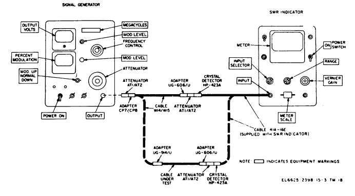
Figure 6-6. RF cable insertion losses, calibration connections.
