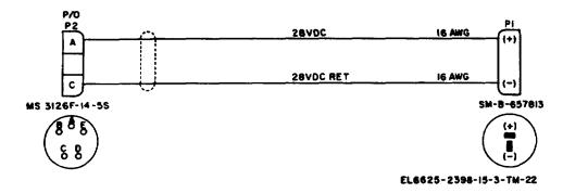
Figure 6-10. Cable W32, schematic diagram.
