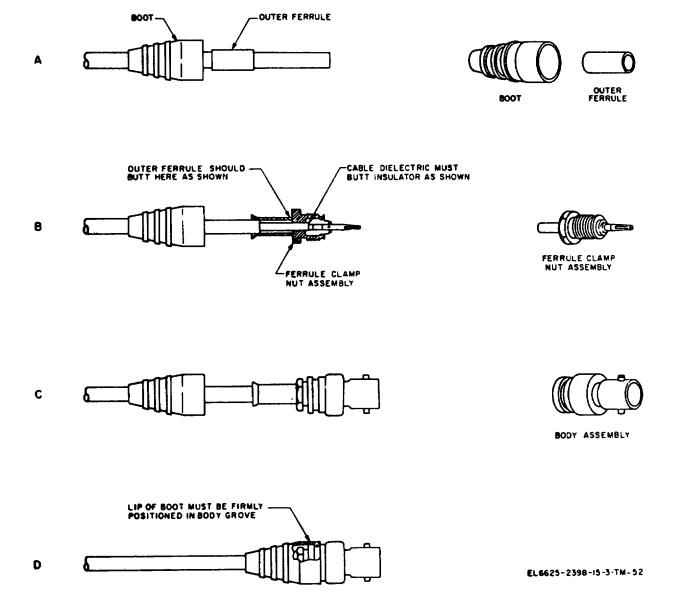
Figure 7-7. Assembly of connector W21P2.
