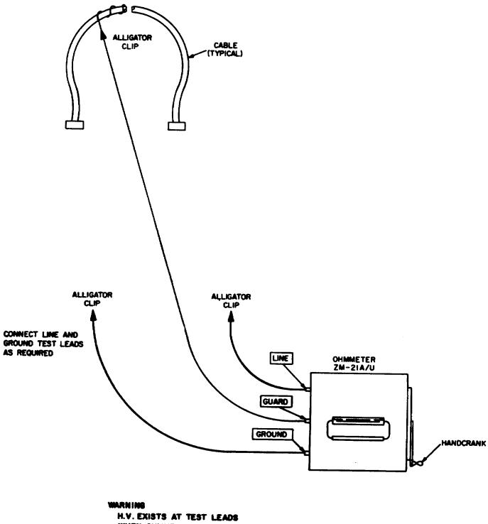
H.V. EXISTS AT TEST LEADS WHEN CHMMETER HANDCRANK IS ROTATED.
