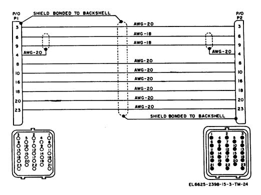
Figure 6-12. Cable W40, schematic diagram.
