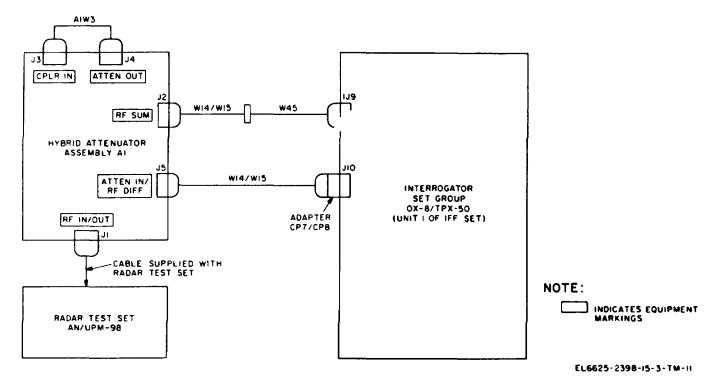
Figure 3-4. Typical hybrid attenuator receiver and transmitter test connections.
