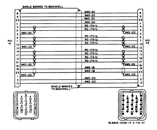
Figure 6-15. Cable W43, schematic diagram.
