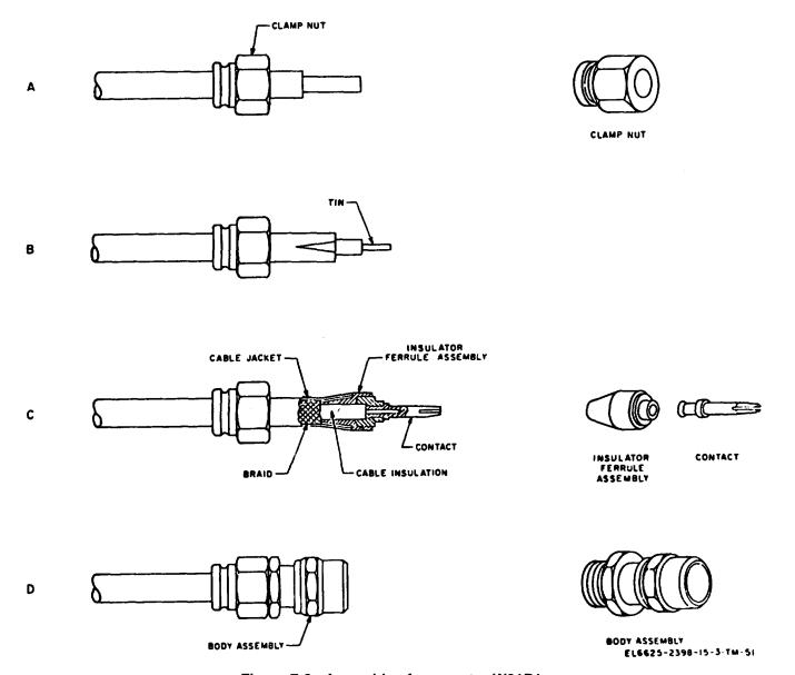
Figure 7-8. Assembly of connector W21P1.
