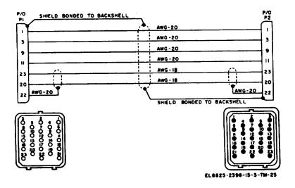
Figure 6-13. Cable W41, schematic diagram.
