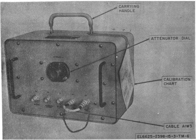
Figure 1-3. Hybrid Attenuator Assembly CN-1322/TPM-24(V).
