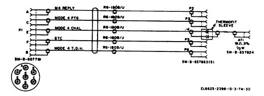
Figure 6-18. Cable W48, schematic diagram.
