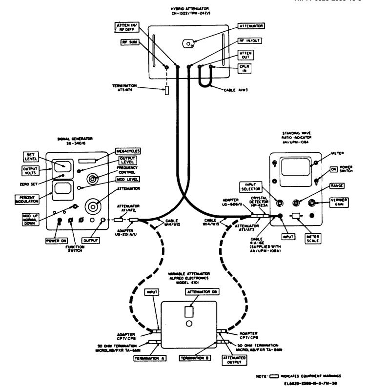
Figure 8-4. Hybrid Attenuator difference channel (between RF IN/OUT and ATTEN IN/RF DIFF connectors) insertion loss, test connections.
