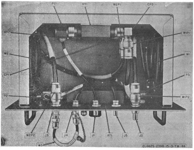
Figure 7-1. Part locations, hybrid attenuator A1.
