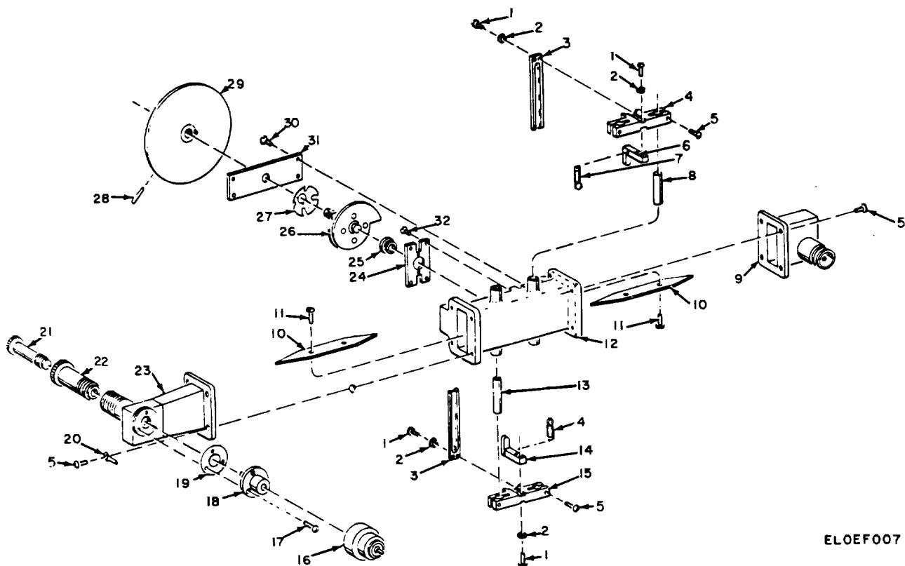
Figure 7. Waveguide Assembly.
