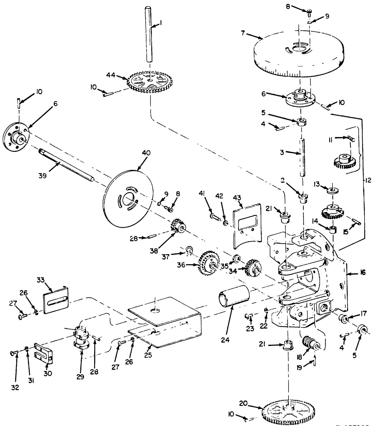
Figure 8. Tuning Drive Assembly.
