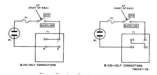
Figure 2. Transformer T1, primary connections.
