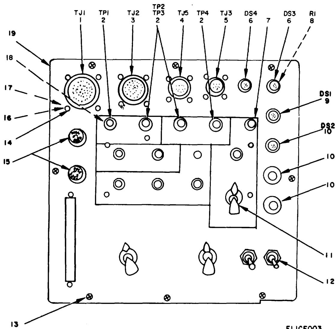
Figure 3. Test Set, Electronic System TS2676/ASM338, panel assembly.
