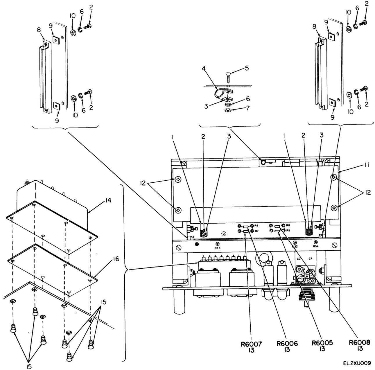
Figure 6. Battery Charger Subassembly, Top View, with Control Board Assembly and Cover in Place (Sheet 1 of 2)
