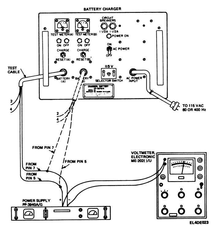
Figure 6-7. Charging voltage cutoff test.
