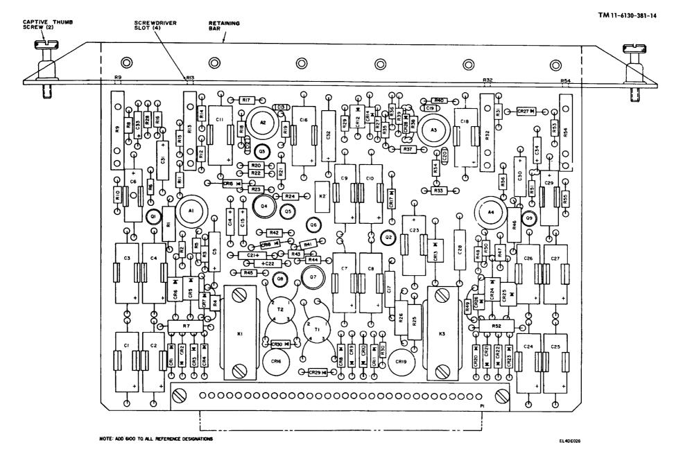
Figure FO 5. Control circuit card assembly, parts location diagram.
