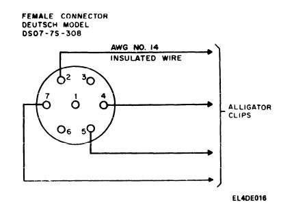
Figure 6-1. Test cable construction diagram.
