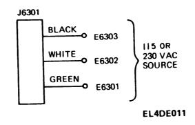
Figure 4-5. 230 vac conversion assembly, schematic diagram.
