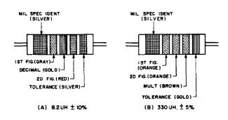
COLOR CODING FOR TUBULAR ENCAPSULATED R.F. CHOKES. AT A, AN EXAMPLE OF OF THE CODING FOR AN 8.2UH CHOKE IS GIVEN. AT B, THE COLOR BANDS FOR A 330 UH INDUCTOR ARE ILLUSTRATED.
