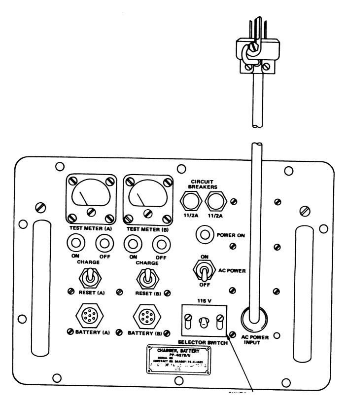
Figure 2-2. Battery charger, controls and indicators.
