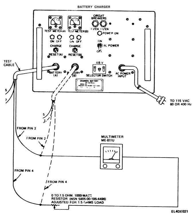
Figure 6-5. Changing c urrent test, 115 volts ac, 60 or 400 Hz.
