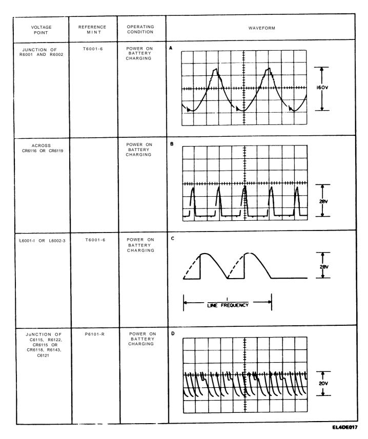
Figure 6-2 ① Waveforms, troubleshooting at genaral support (sheet 1 of 2).
