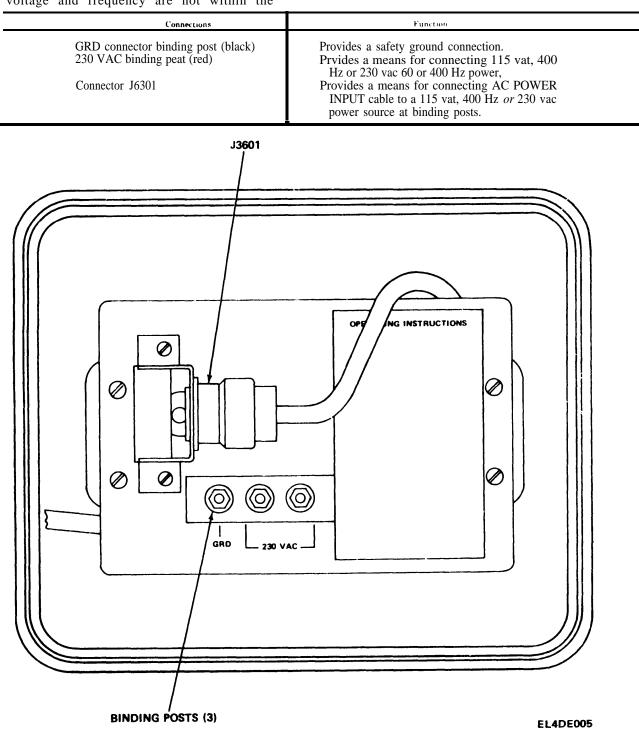
Figure 2-3. 230 vac conversion assembly, connections
