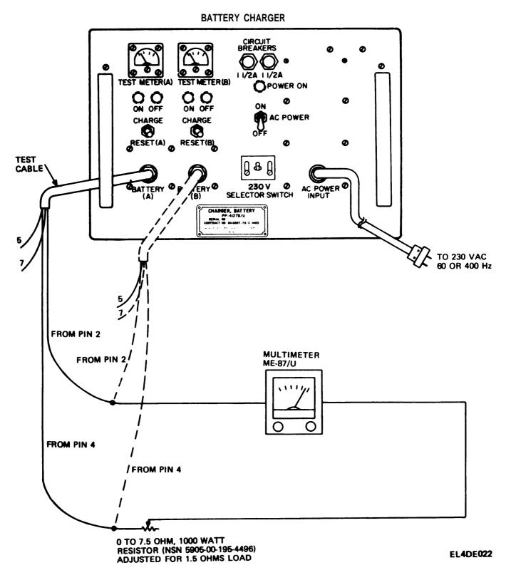
Figure 6-6. Charging current test, 290 volts ac, 60 or 400 Hz.
