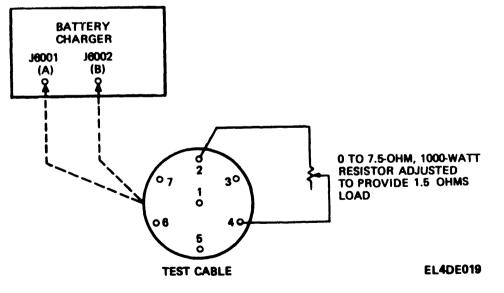
Figure 6-3. Test setup for adjusting battery charging current.
