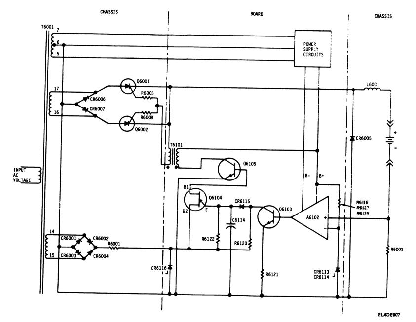
Figure 4-1. Basic ac phase-controlled current regulator, simplified schematic diagram.
