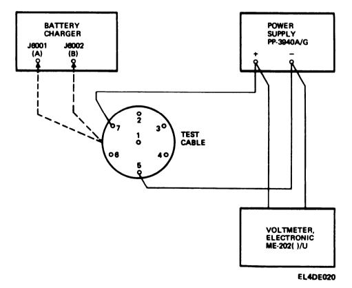
Figure 6-4. Test setup for adjusting charging voltage-sensing and cutoff circuit.
