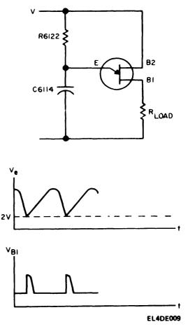
Figure 4-3. Basic UJT miltivibrator circuit.
