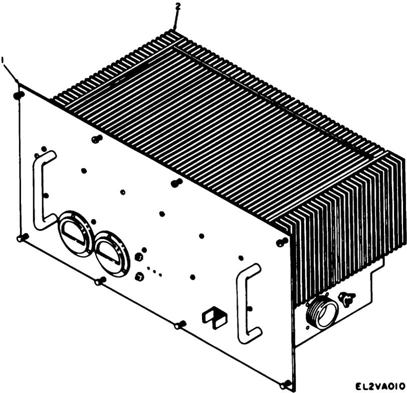
Figure 1. Power supply PP-6187/TSW
