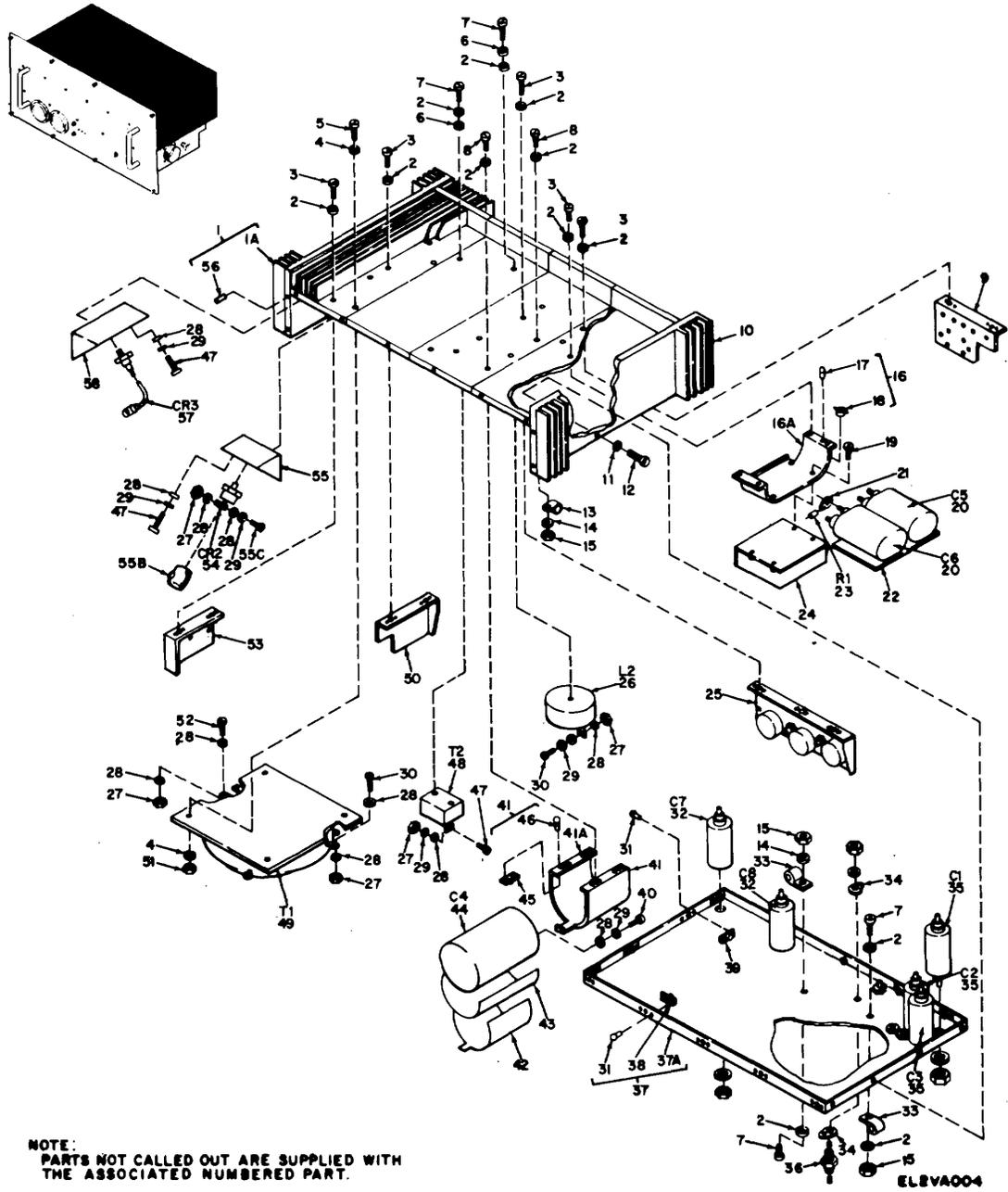
Figure 4. <sup>1</sup>Heatsink assembly, rectifier converter (sheet 1 of 2)
