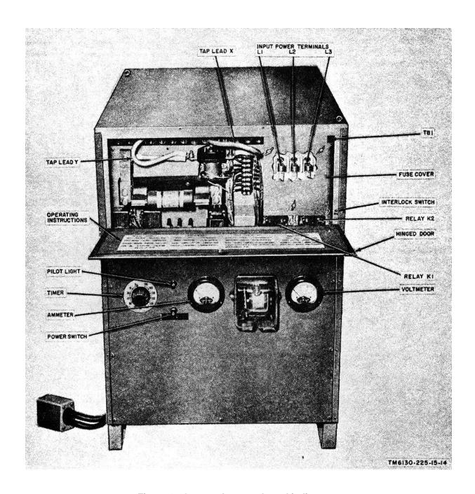
Figure 6. Operator's controls and indicators.
