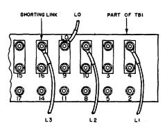
C. ARRANGEMENT OF SHORTING LINKS AND LEADS FOR 230 V 3 PHASE POWER INPUT
