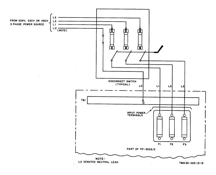
Figure 3. Power disconnect switch wiring.
