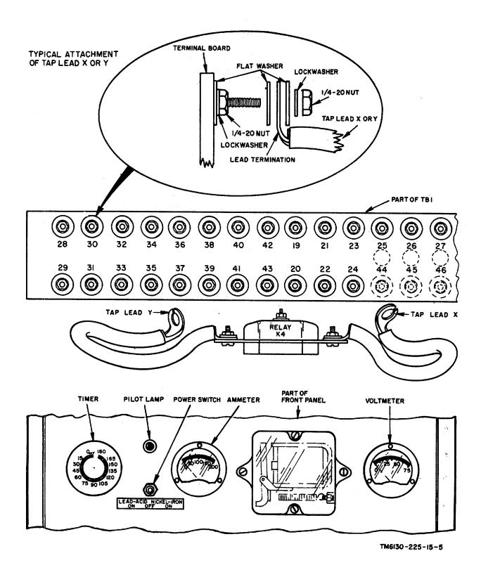
Figure 5. Terminal board tap lead connections and front panel controls and indicators.
