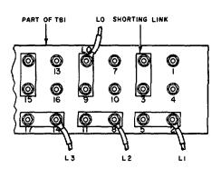
D. ARRANGEMENT OF SHORTING LINKS AND LEADS FOR 208 V 3 PHASE POWER INPUT TM6130-225-15-4
