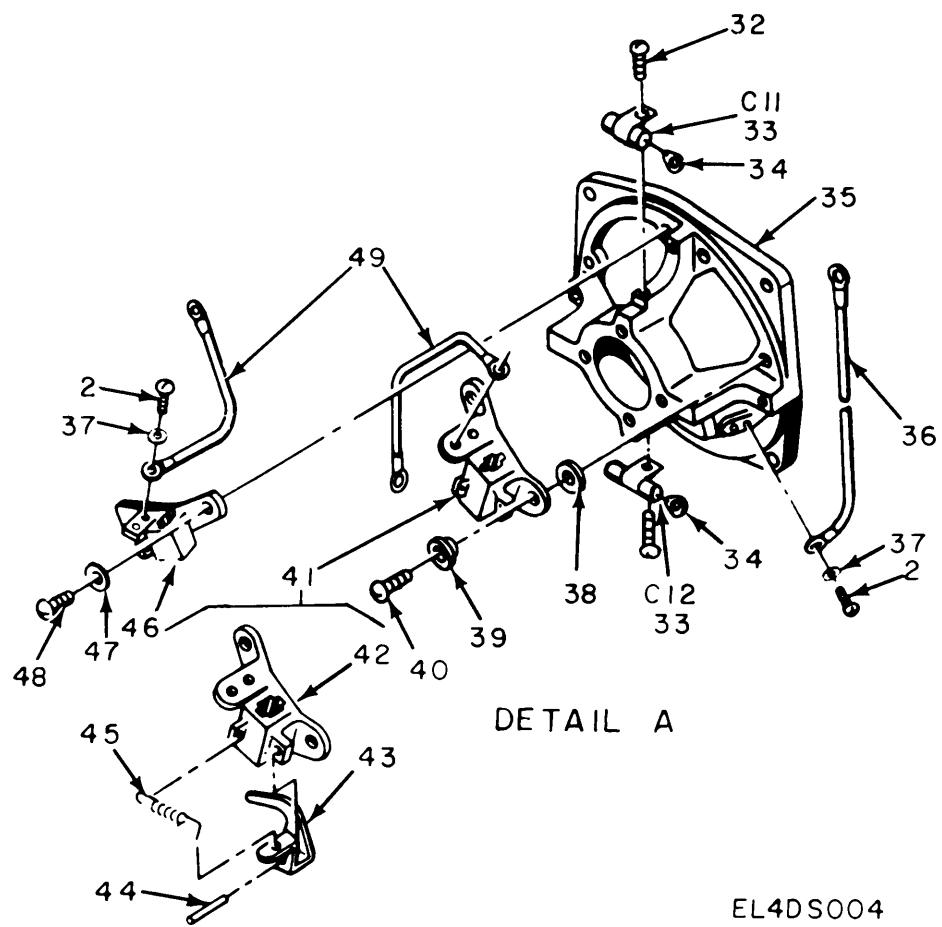
Figure 2. Motor-Generator PU-543C/A, Rotating Section (Sheet 2 of 2).
