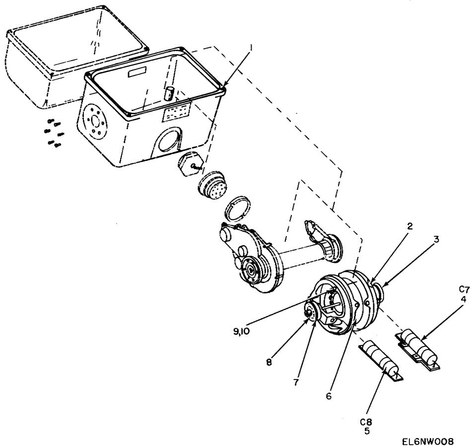
Figure 7. Generator Assembly.
