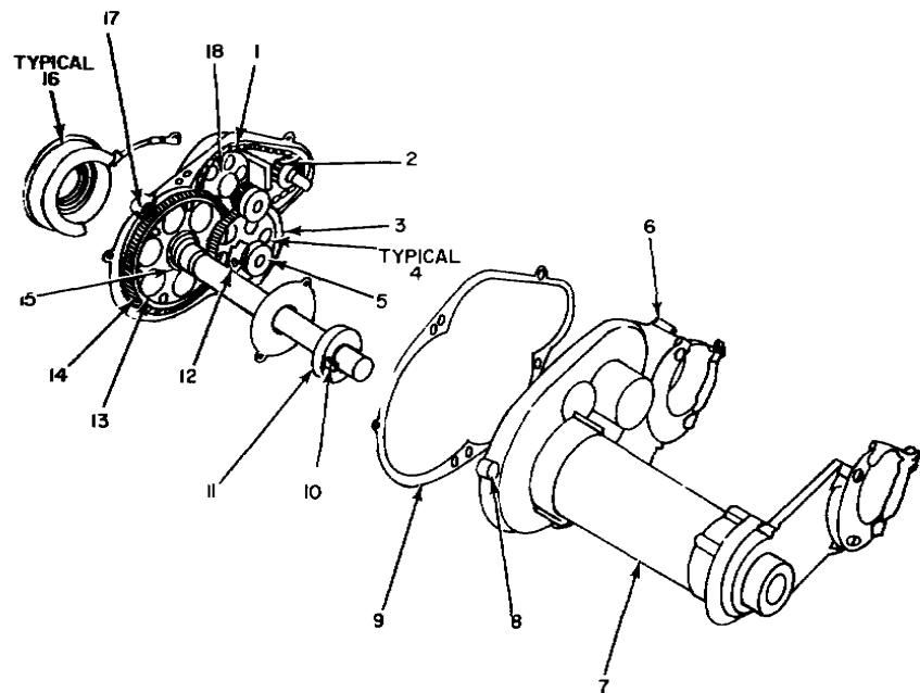
Figure 2. Gear Assembly, Speed Increaser.
