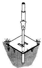
STEP 3 Secure the MAST BASE PLATE with the two MAST BASE STAKES.
