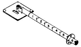
STEP (10) Assemble the 5 UPPER MAST SECTIONS AND join them to the masts on the ground.
