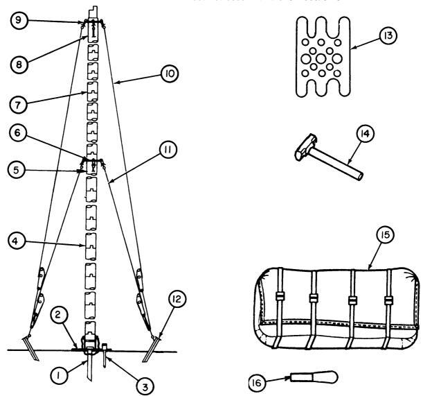
NOTE: Items used with the LOWER MAST SECTIONS and the LOWER GUYS are associated with Blue markings on components. Items used with the UPPER MAST SECTIONS and the UPPER GUYS are associated with Red markings on components.
