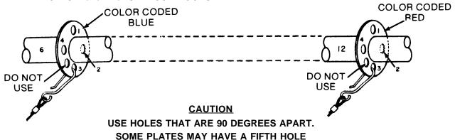
STEP 14 Attach each of the 4 GUY HOOKS (color code BLUE) to the proper hole on the LOWER GUY PLATE.
