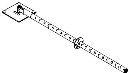
STEP (11) Slide the UPPER GUY PLATE (color code RED) onto the male end of the UPPER ADAPTER ASSEMBLY.
