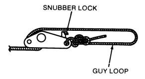
Remove the guy rope from the SNUBBER LOCK -
