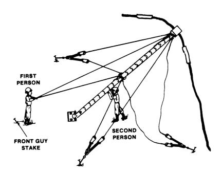
The **FIRST PERSON walks backwards** towards the FRONT GUY STAKE **pulling on the FRONT GUY ROPES** to assist in raising the MAST and in keeping the slight bow in the MAST.
