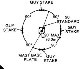
Position the movable short MAST on the MAST AND BASE ASSEMBLY so it lays on the MAST BASE PLATE in the direction the mast will be assembled.
