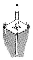
STEP 4 PLACE a short STANDARD (20') over the short MAST of the MAST AND BASE
