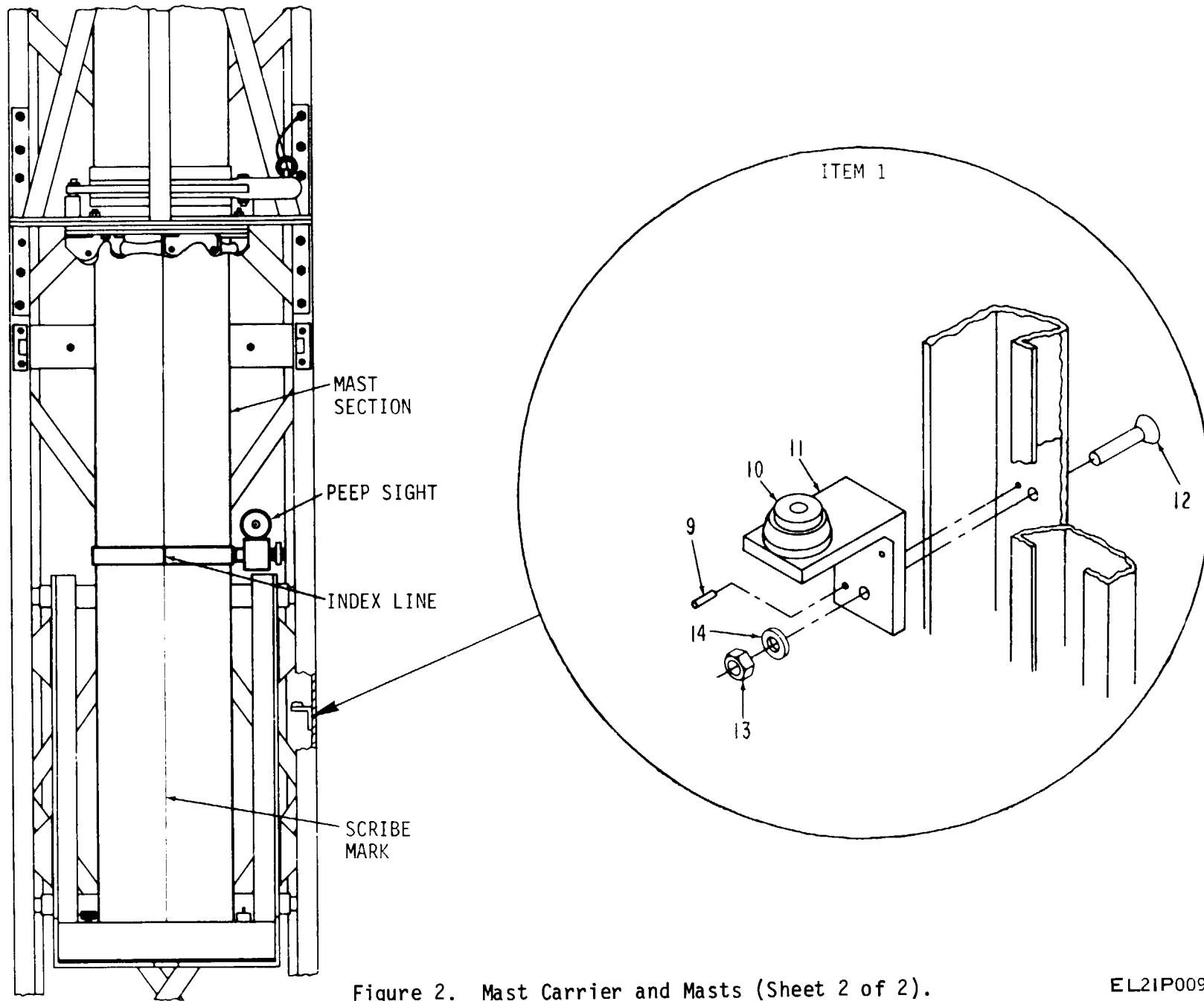
Figure 2. Mast Carrier and Masts (Sheet 2 of 2).
