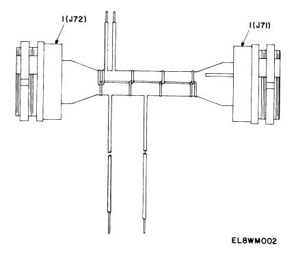
Figure 2. Wiring harness assembly SM-D-951293.
