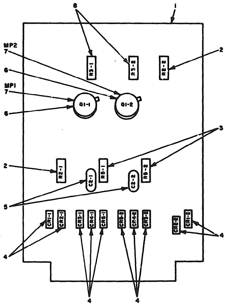
Figure 9. Circuit card assembly (5 GD logic gate) 398-6538-4.
