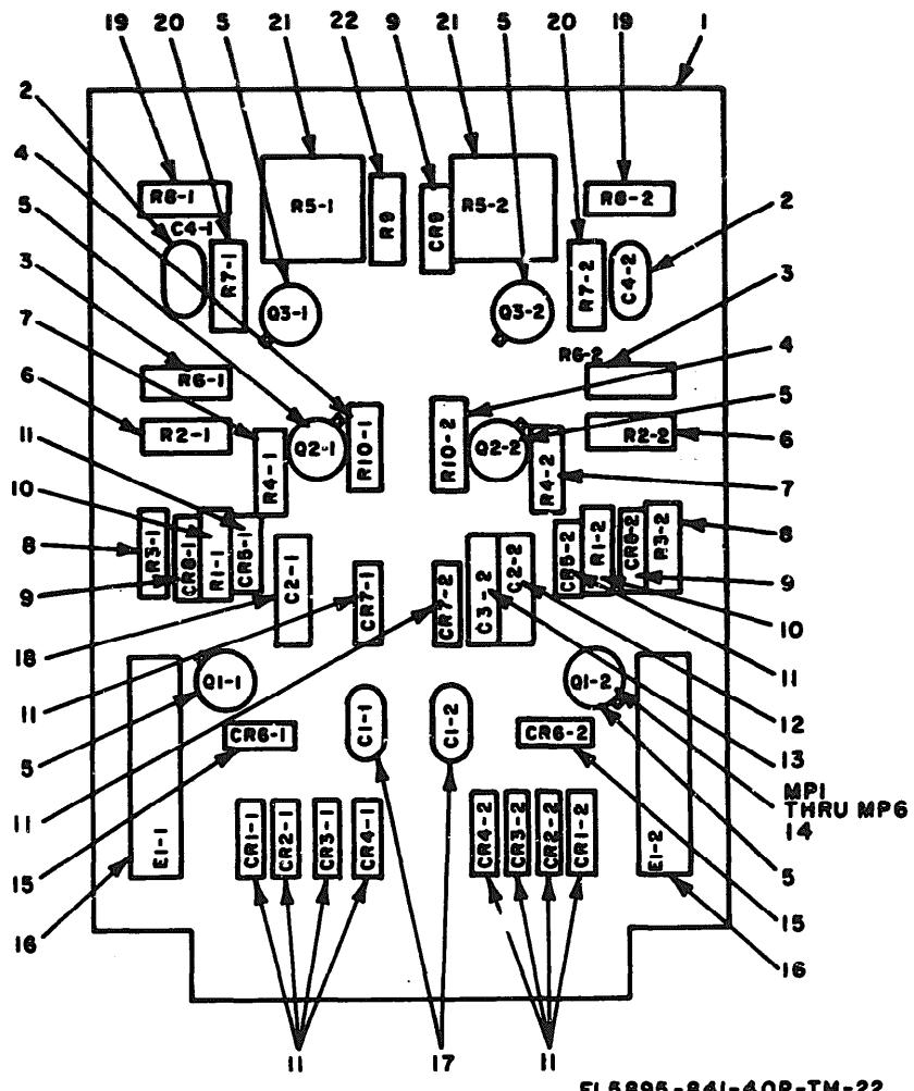
Figure 22. Circuit Card Assembly (SSS1 single-shot) 398-6607-11203.
