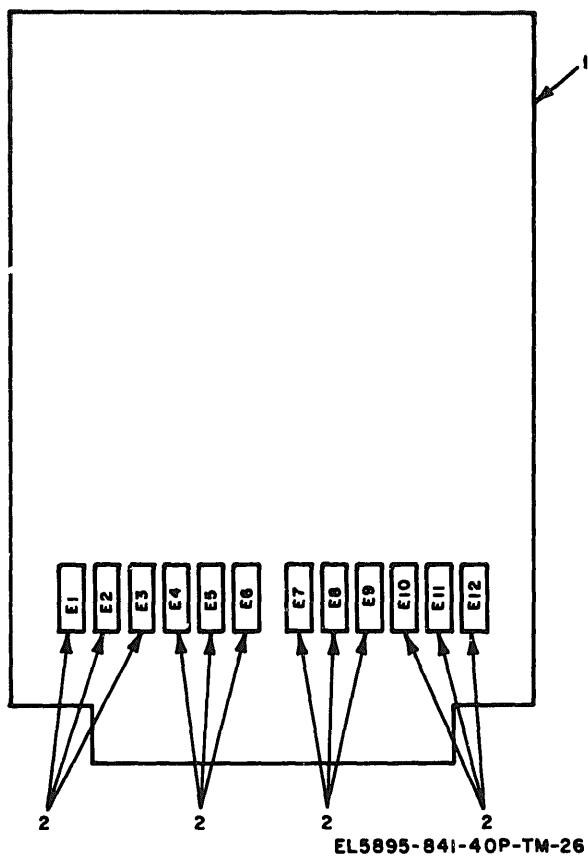
Figure 26. Circuit card assembly (IRBCA resistor board) 398-4490-3.
