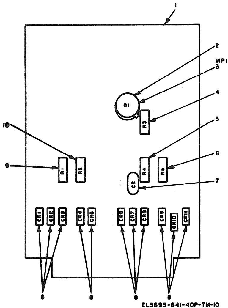
Figure 10. Circuit Card Assembly (11GC logic gate) 398-6539-3.
