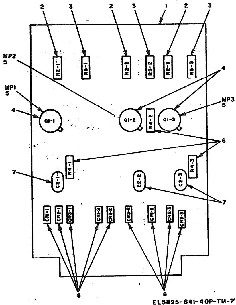
Figure 7. Circuit card assembly (3 GD logic gate) 398-6535-4.
