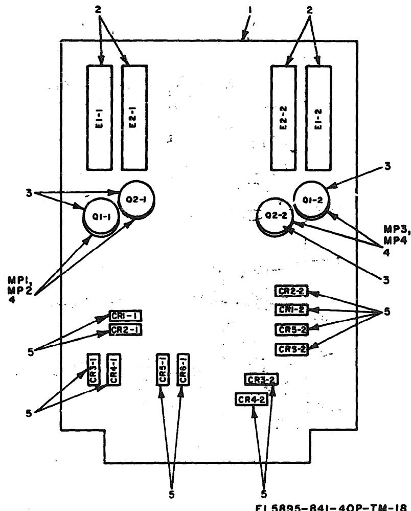
Figure 18. Circuit Card Assembly (4FD flip-flop) 398-6550-4.
