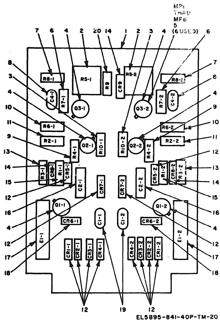
Figure 20. Circuit Card Assembly (SSS1 single-shot) 398-6607-10101.
