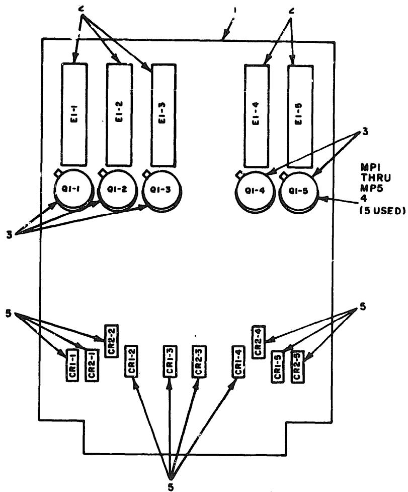
Figure 13. Circuit Card Assembly (52GC logic gate) 398-6546-3.
