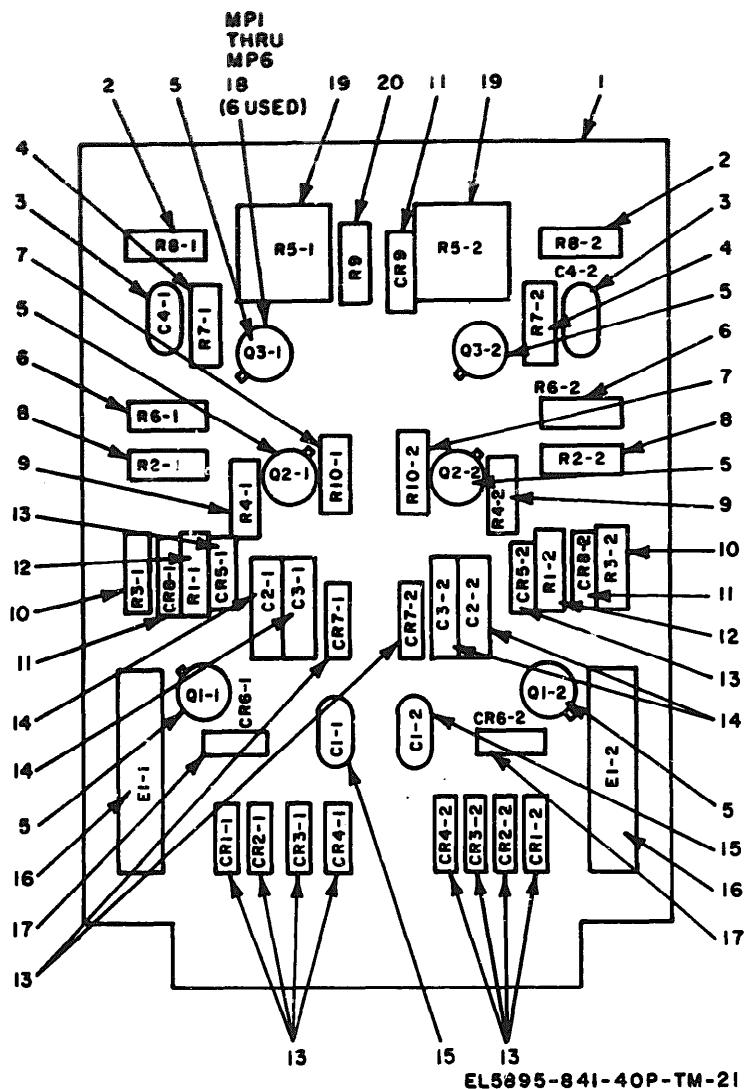
Figure 21. Circuit Card Assembly (SSS1 single-shot) 398-6607-10303.
