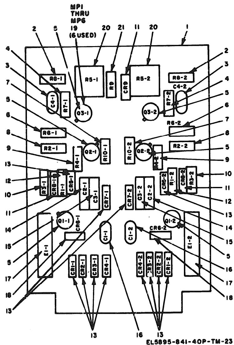
Figure 23. Circuit Card Assembly (SSS1 single-shot) 398-6607-11818.
