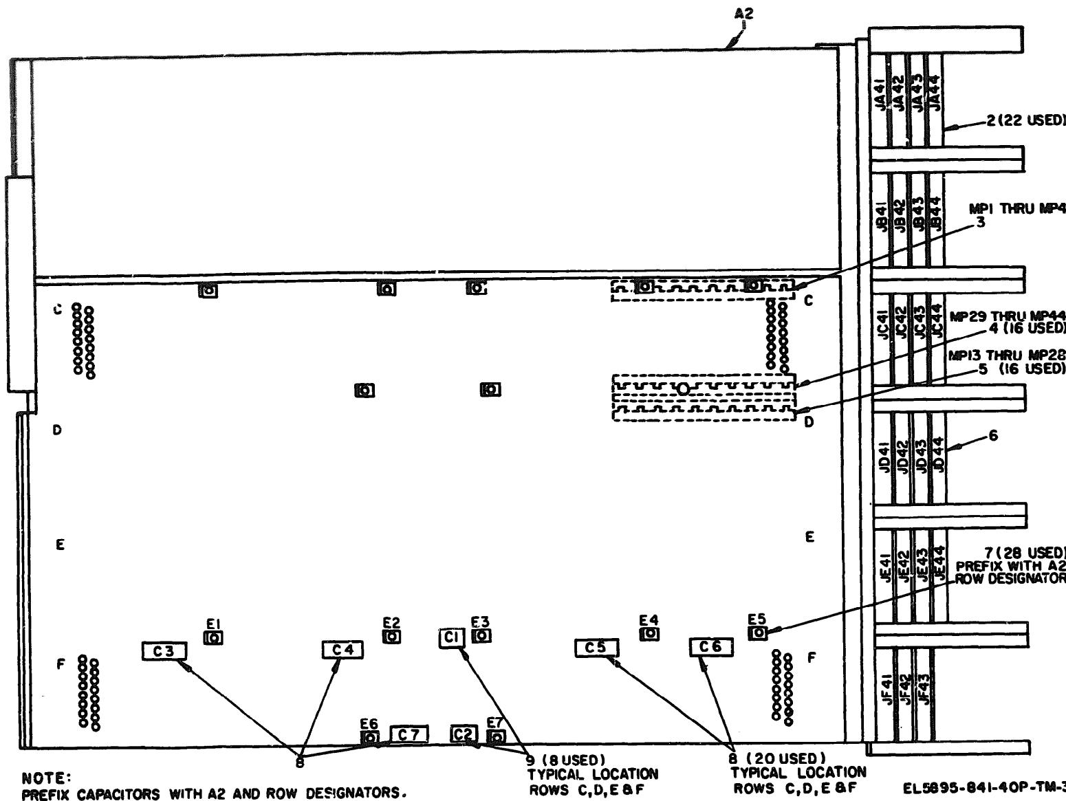
Figure 3. Functional assembly, drum 398-7517-2.
