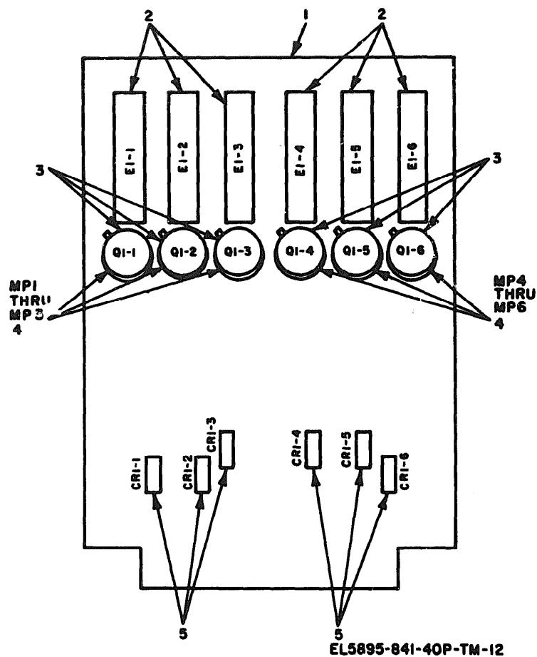
Figure 12. Circuit Card Assembly (1GC logic inverter) 398-6545-3.
