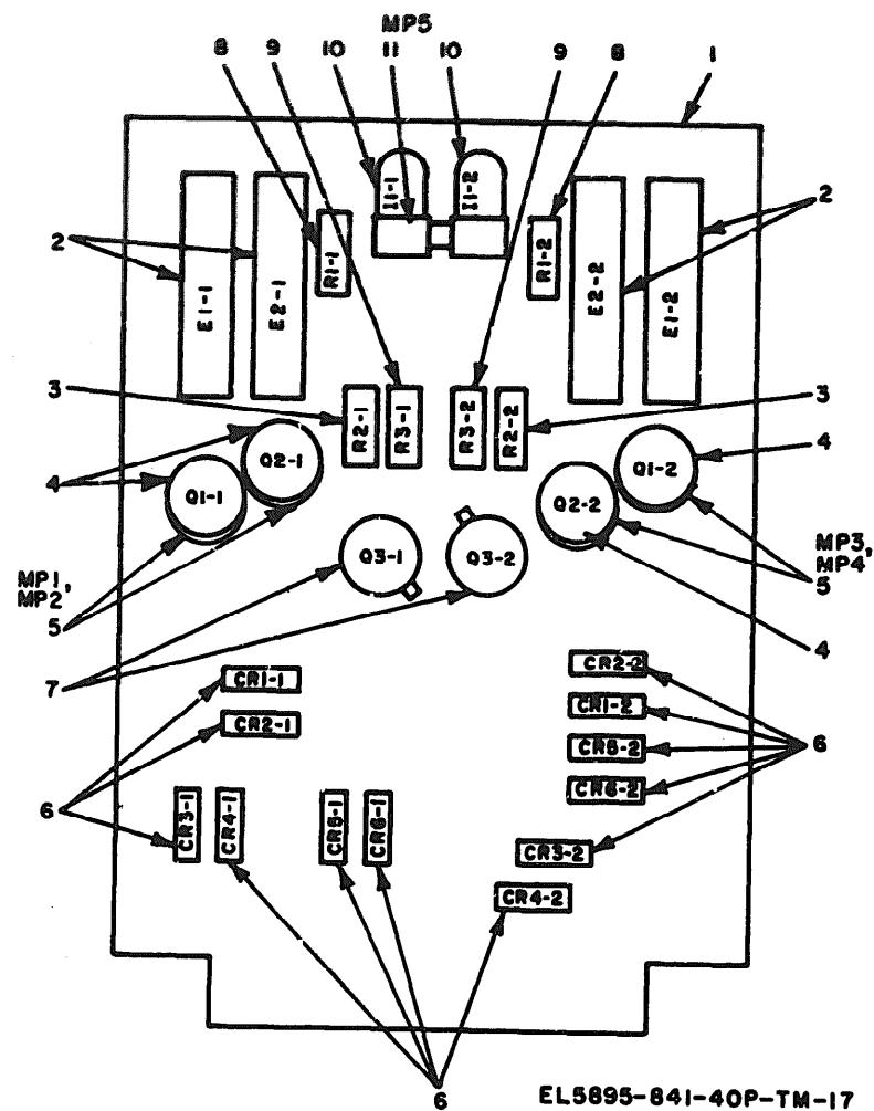
Figure 17. Circuit Card Assembly (4FC flip-flop) 398-6550-3.
