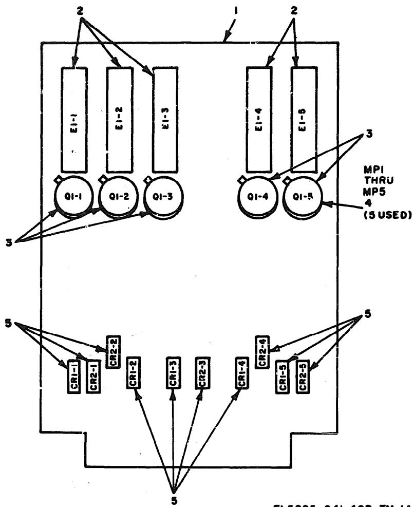
Figure 14. Circuit Card Assembly (52GD logic gate) 398-6546-4.
