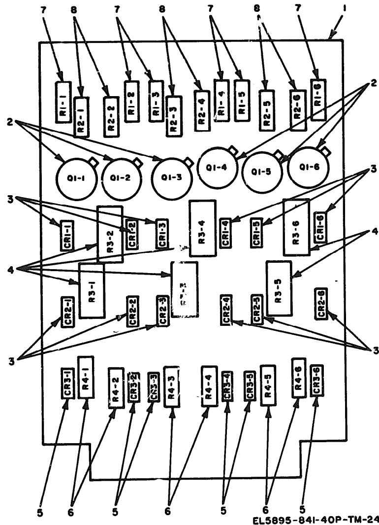
Figure 24. Circuit Card Assembly (IMLDA lamp driver) 398-6820-1.
