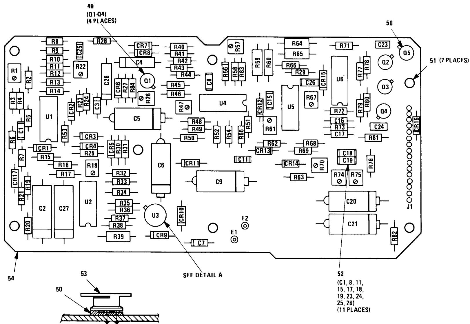
Figure 15. Power Supply Board No. 1 Circuit Card Assembly
