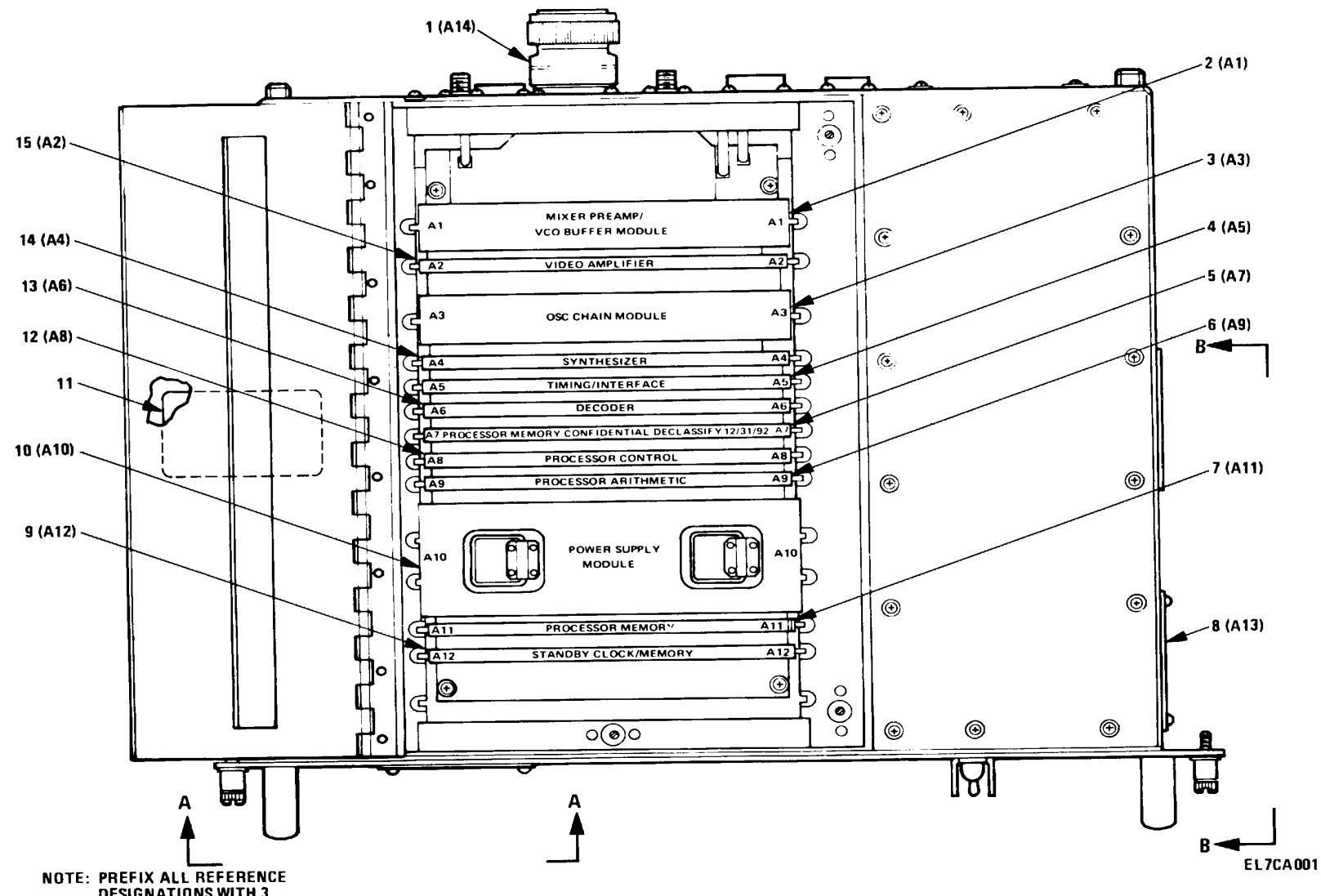
*Figure 1. Modem, Digital Data MD-1094/G (3) (Sheet 1 of 2)*
