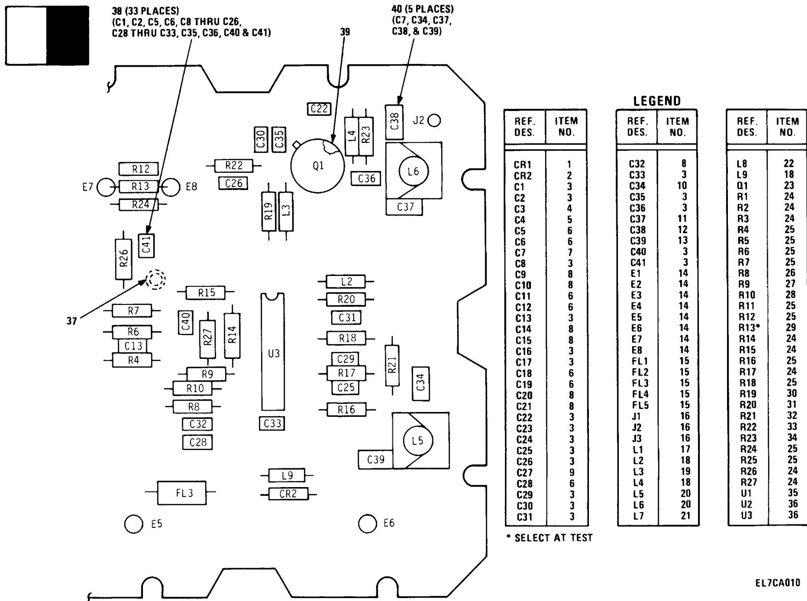
Figure 5. VCO Buffer Circuit Card Assembly (3A1A3), (Sheet 2 of 2)
