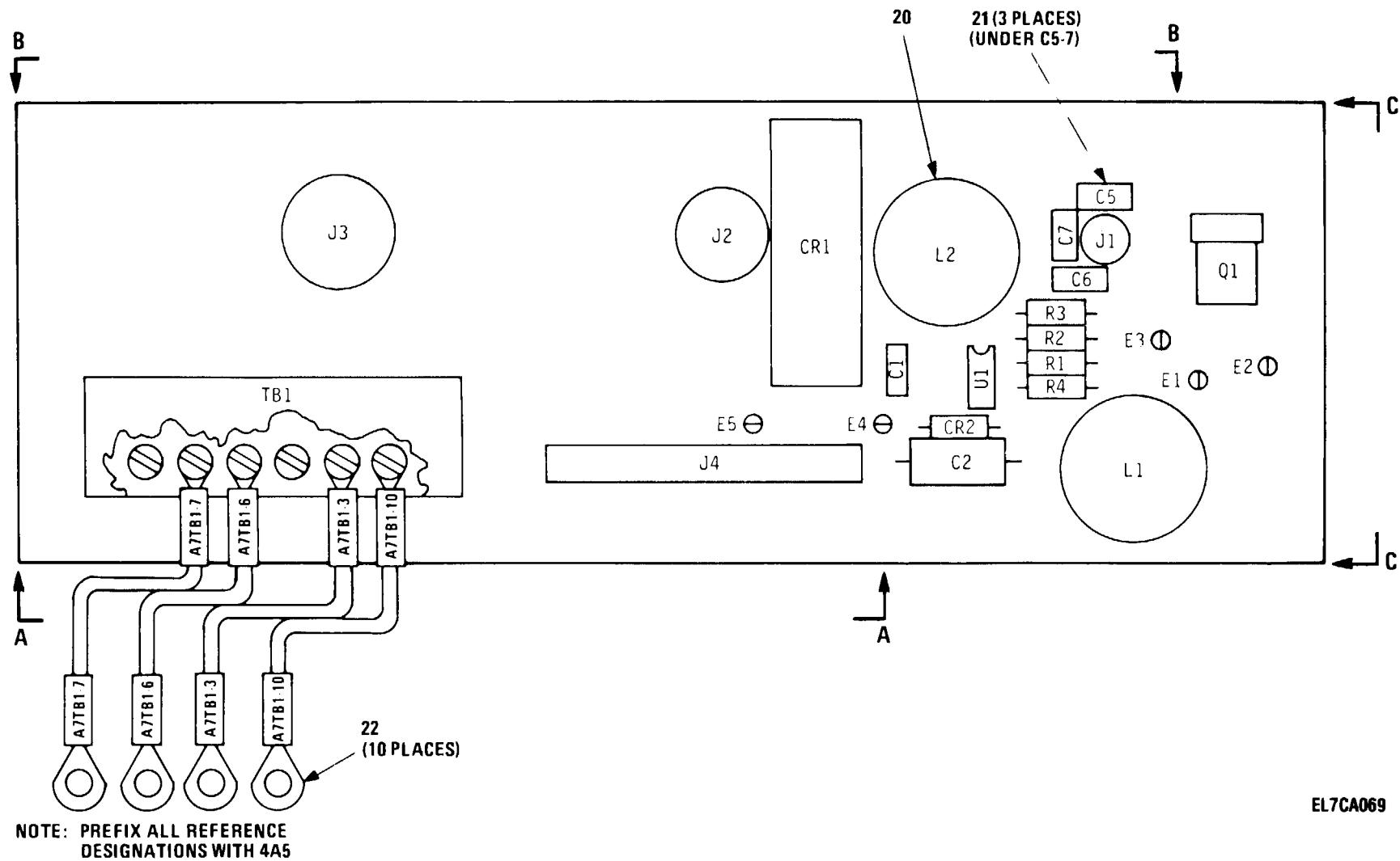
Figure 37. Interface Circuit Card Assembly (4A5) (Sheet 1 of 3)
