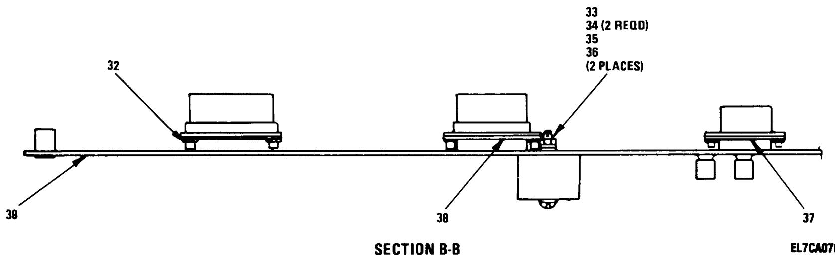
Figure 37. Interface Circuit Card Assembly (4A5) (Sheet 2 of 3)
