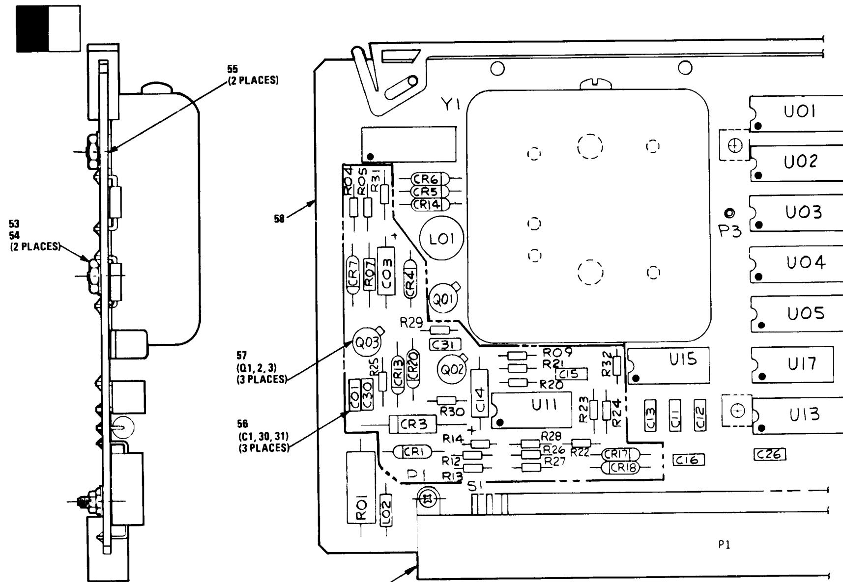
Figure 17. Standby Clock Memory Circuit Card Assembly (3A12A2)
