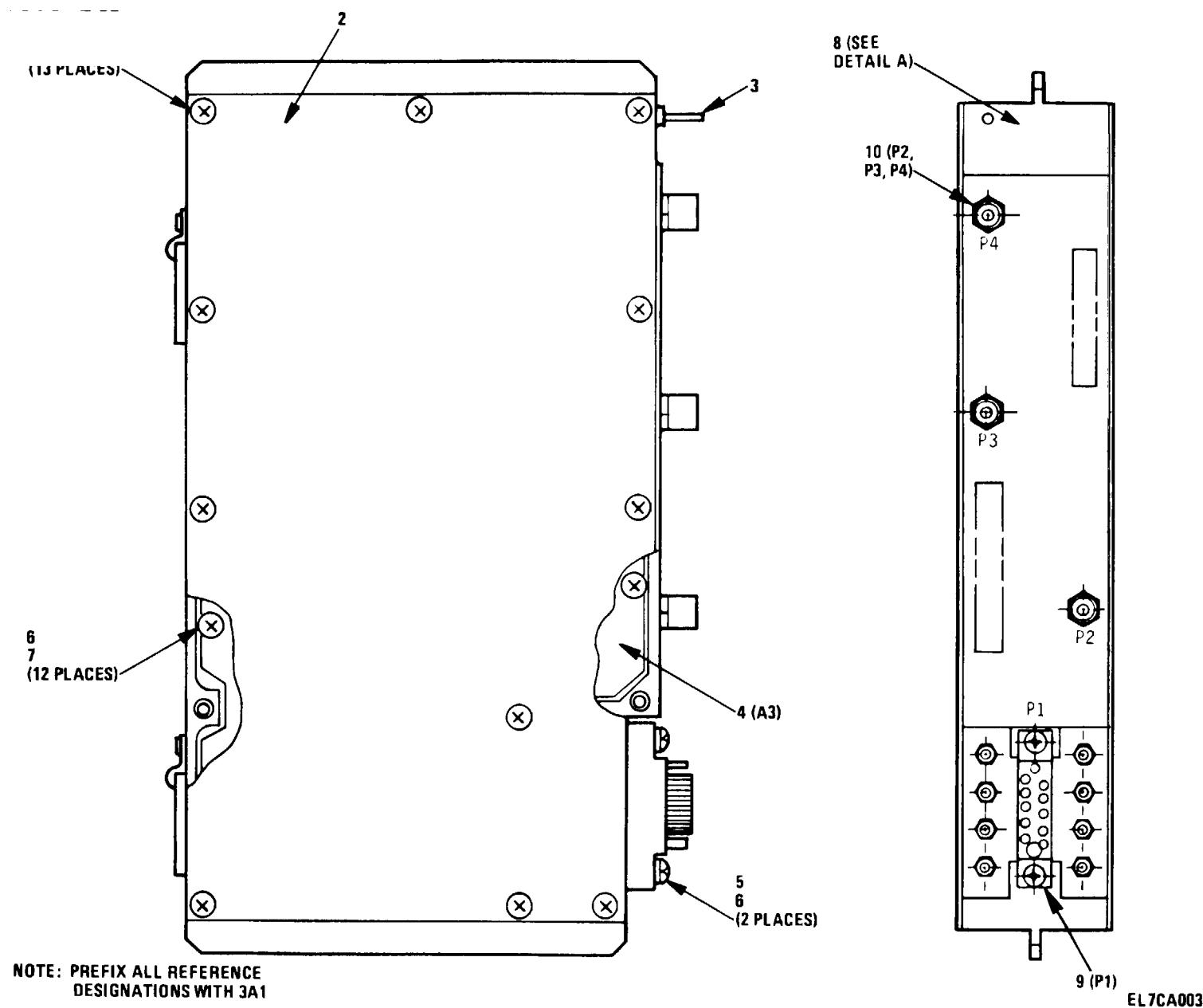
Figure 2. Mixer Preamp/VCO Buffer Module (3A1) (Sheet 1 of 3)
