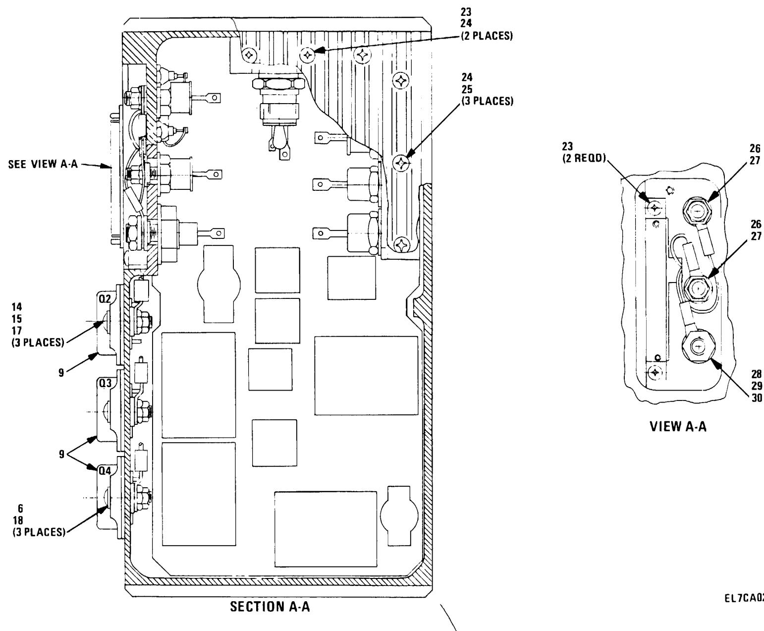
Figure 12.. Power Supply Module (3A10) (Sheet 2 of 4)
