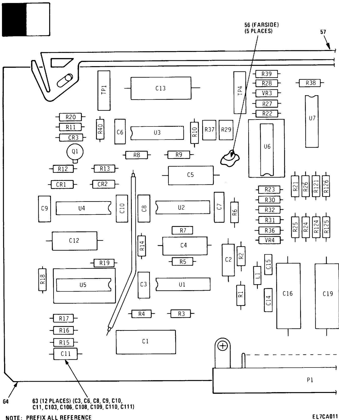
Figure 6. Video Amplifier Circuit Card Assembly (3A2) (Sheet 1 of 3)
