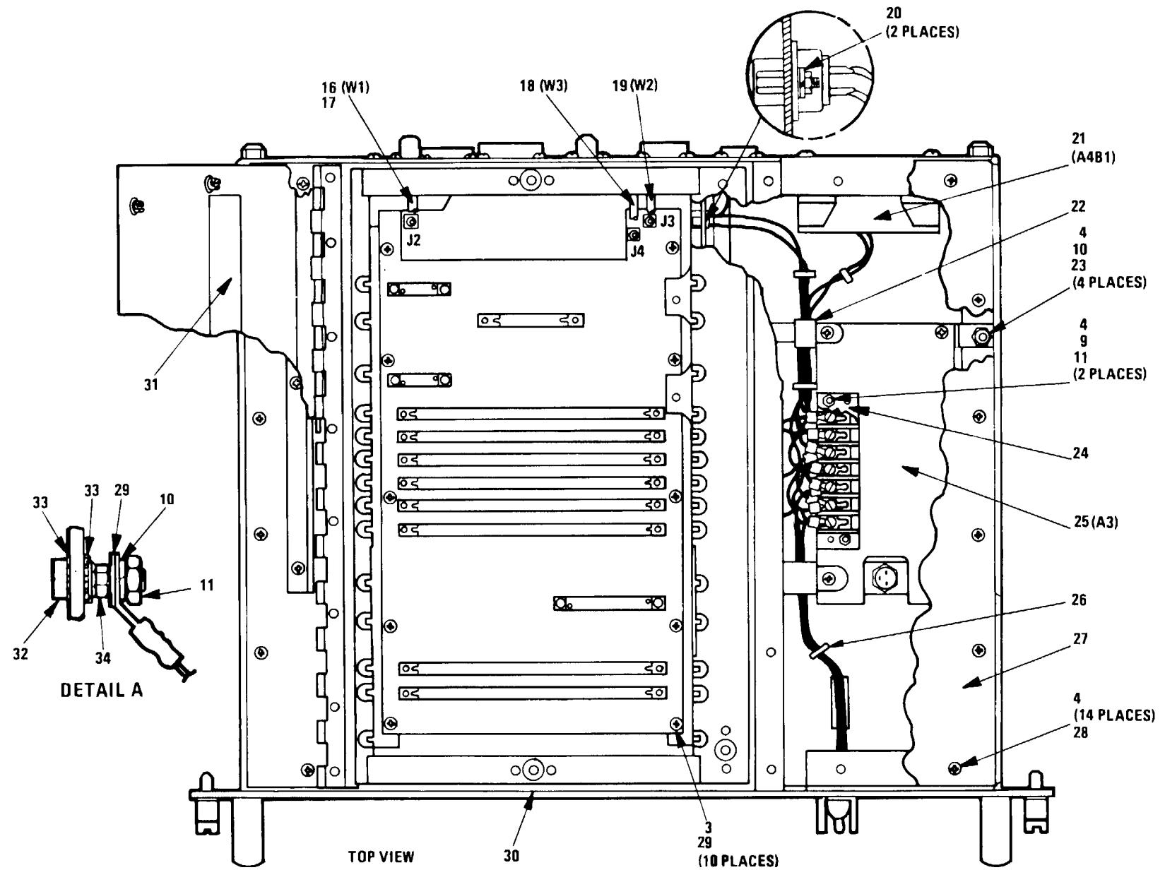
Figure 19. Chassis Assembly (3A13) (Sheet 2 of 2)
