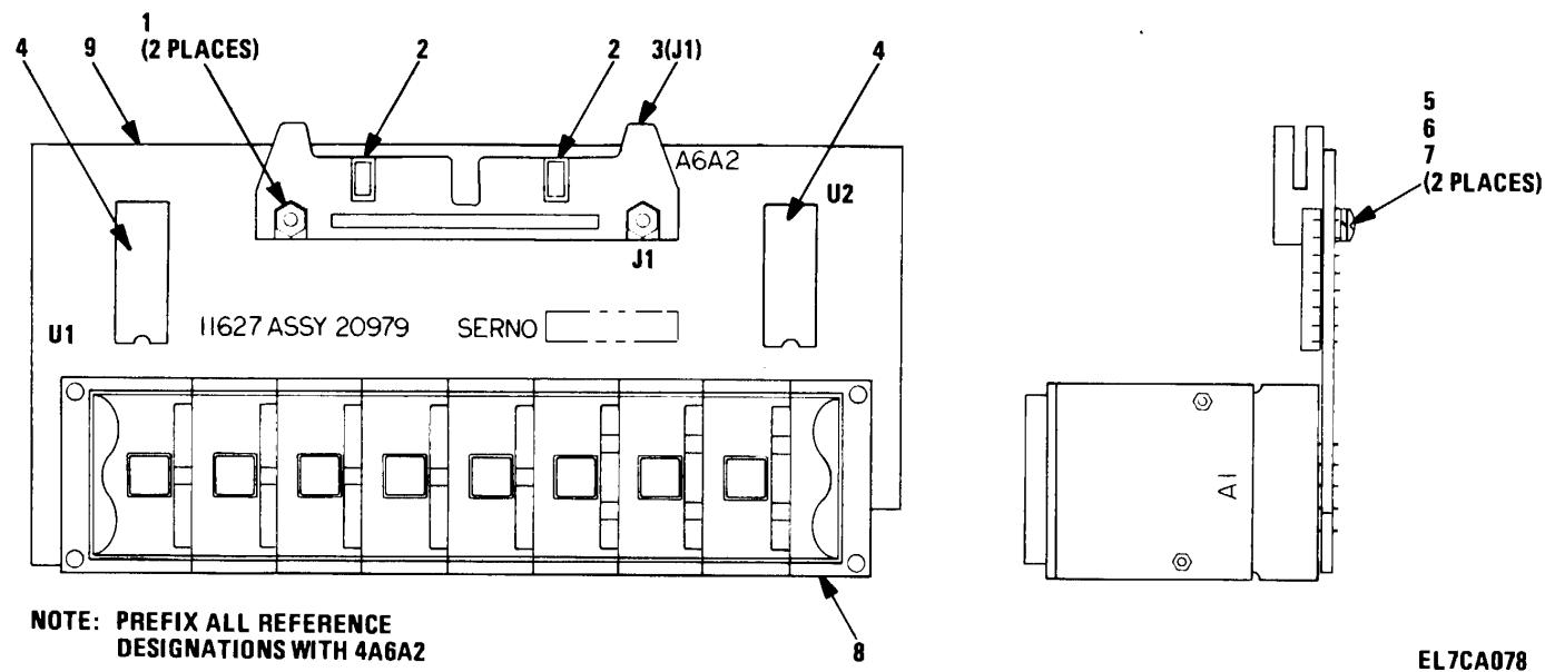
Figure 41. Front Panel Circuit Card Assembly (4A6A2)
