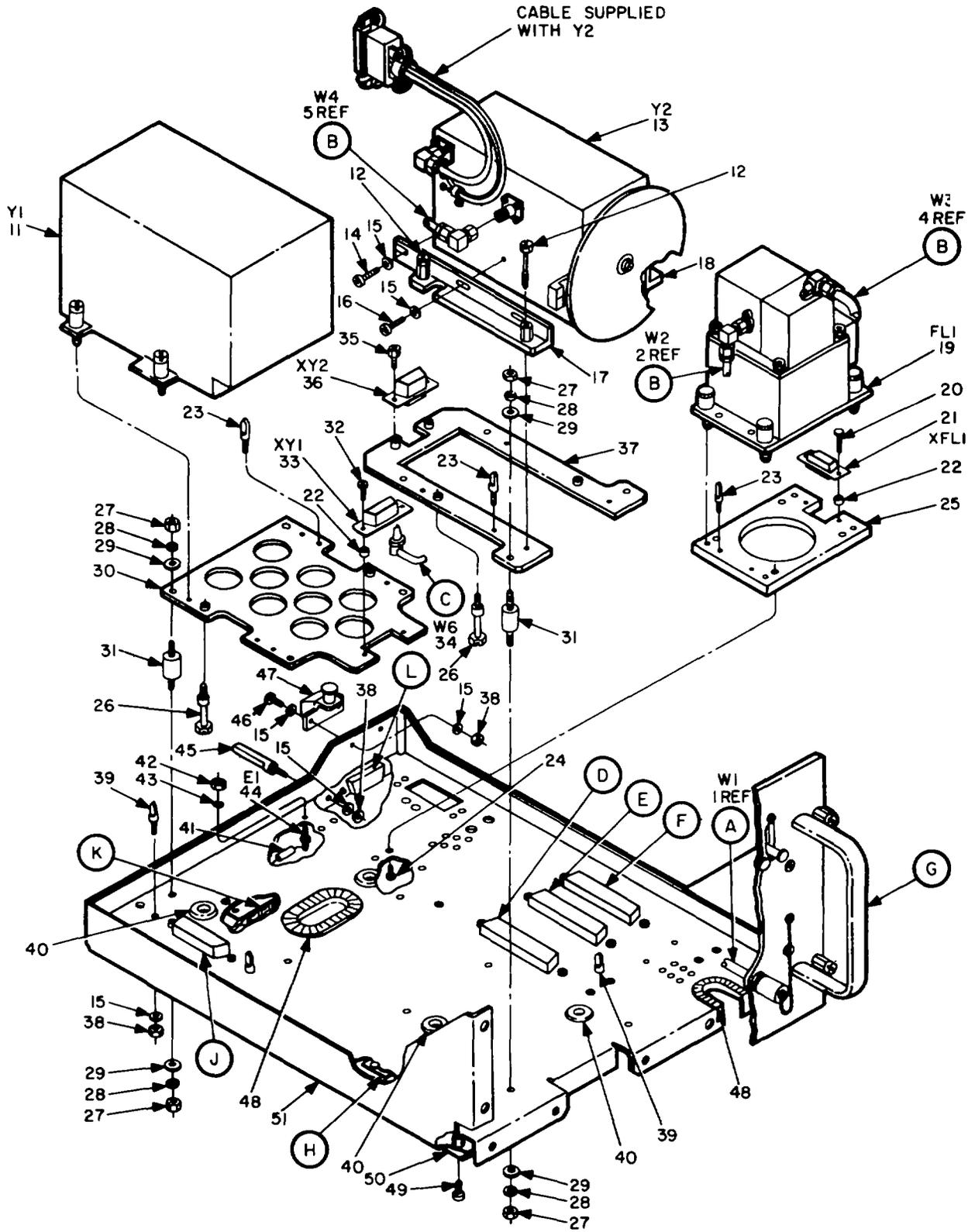
Figure 2. Electronic Frequency Synthesizer 0-1678/TSC (Sheet 2 of 6).
