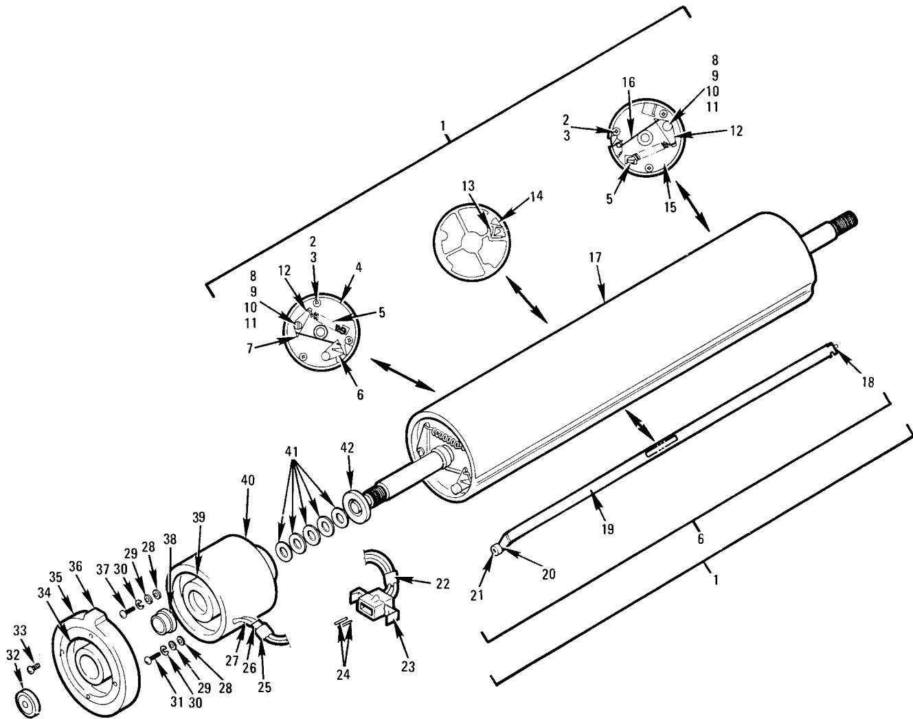
FIGURE 14. DRUM DRIVE ASSEMBLY
