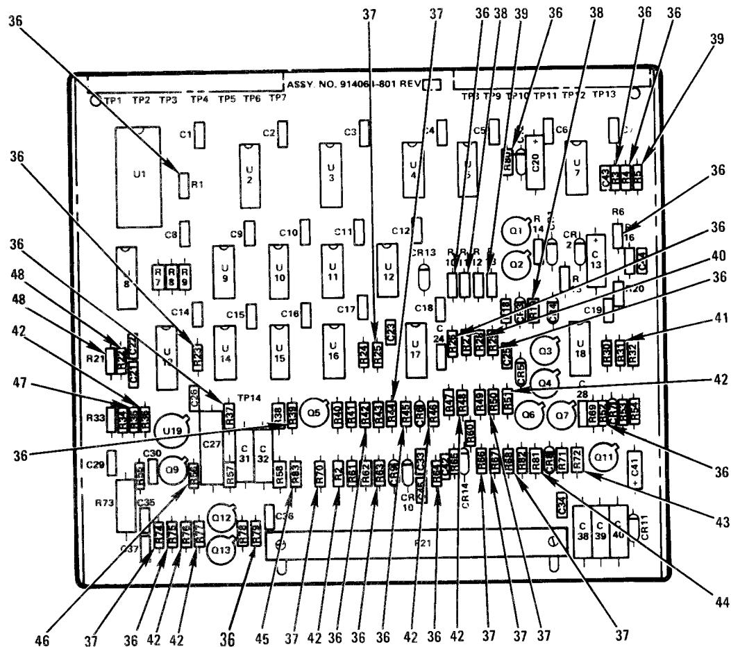
FIGURE 22. BASEBAND SERVO CIRCUIT CARD (3 of 4)
