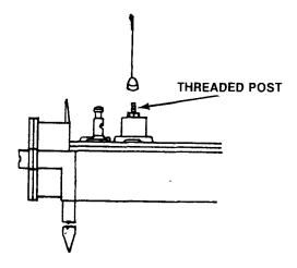
• Screw detector antenna onto threaded post top of detector.
