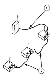
Field wire 1 is run to first detector in Hot-Loop group. Other lengths of field wire 2 connect other detectors with each other in "Parallel".
