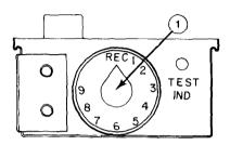
ŽWhen in wire mode be sure REC-TEST switch on wire link is set to REC position.
