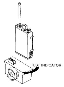
(2) Set TEST switch through positions 1 thru 9 and observe flashing indicator.
