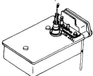
4 **DETECTOR.** (10 each) Small, light-weight, battery powered. Detects ground vibrations (personnel) or magnetic (vehicle) intrusions. Sends message to receiver by RF or wire transmission. Adapts to different environments, Has self-test features. Detector antenna screws into top of unit. Two ground holding stakes screw into bottom of each dSector.
