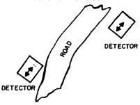
Ž Push detector into hole so that holding stakes are firmly implanted into ground. DO NOT STEP ON DETECTOR.
