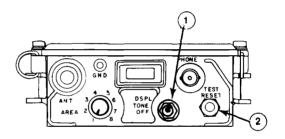
To erase memory, press TEST RESET button (2) on receiver.
