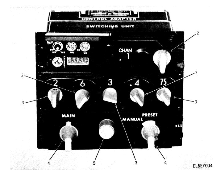
Figure 3. Switching Unit (1A1).
