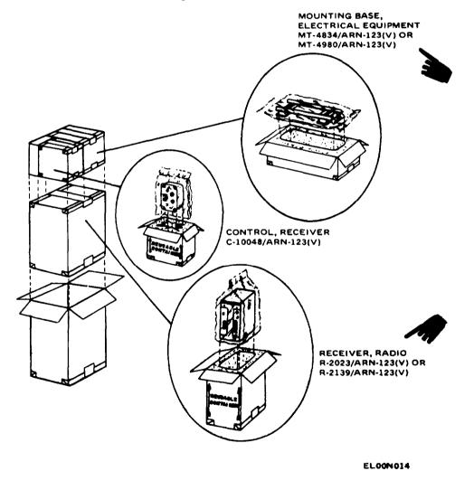
Figure 1-4. Interface conversion group packaging diagram, for receiving set, radio AN/ARN-123(V).
