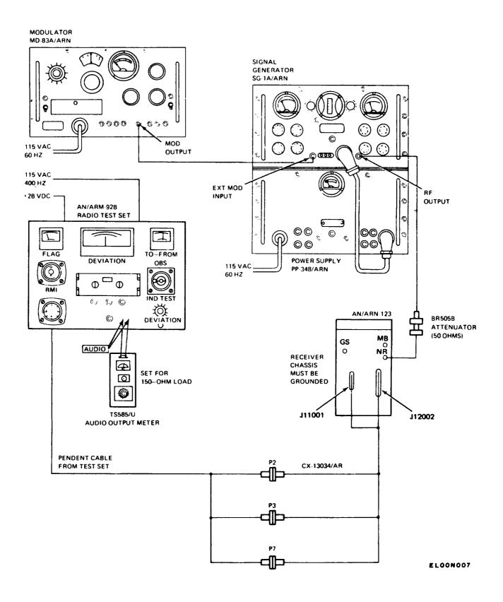
Figure 3-1. Bench Test Setup, VOR/LOC.
