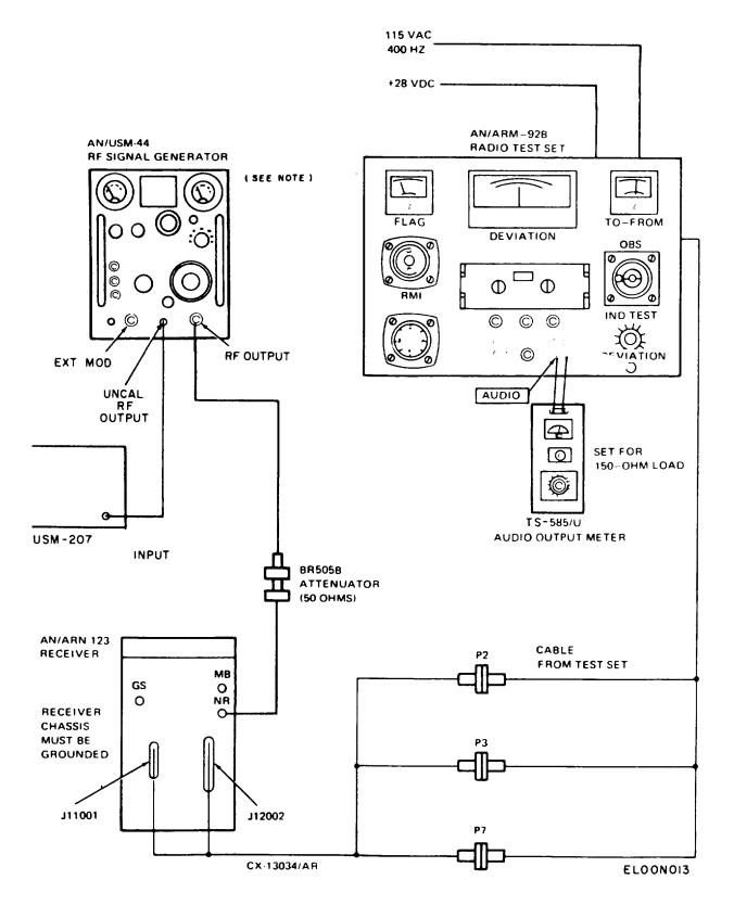
Figure 3-5. Bench Test Set, Alternate VOR/LOC Receiver Setsitivity Test.
