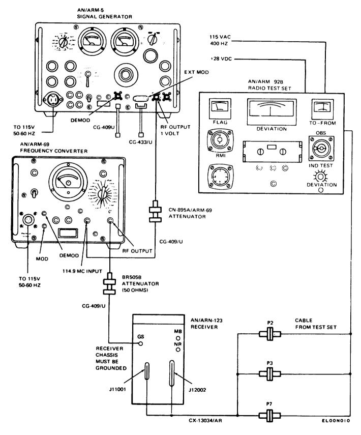
Figure 3-2. Bench Test Setup, Glideslope.
