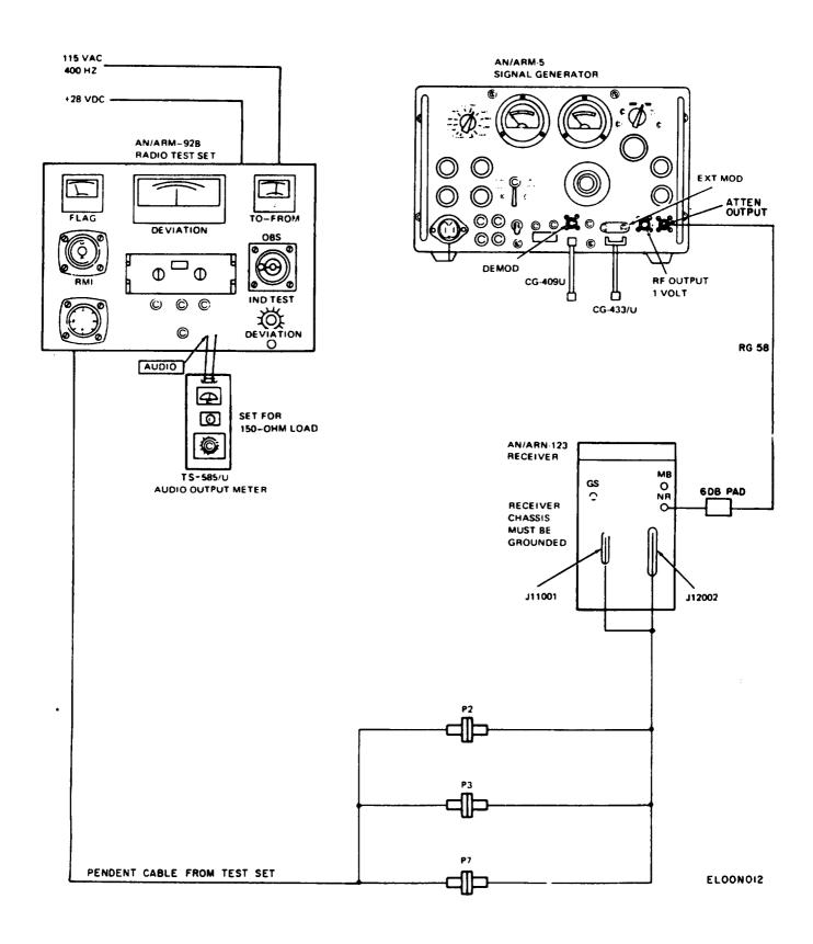
Figure 3-4. Bench Test Setup for VOR/LOC Tests usingAN/ARM-5A.
