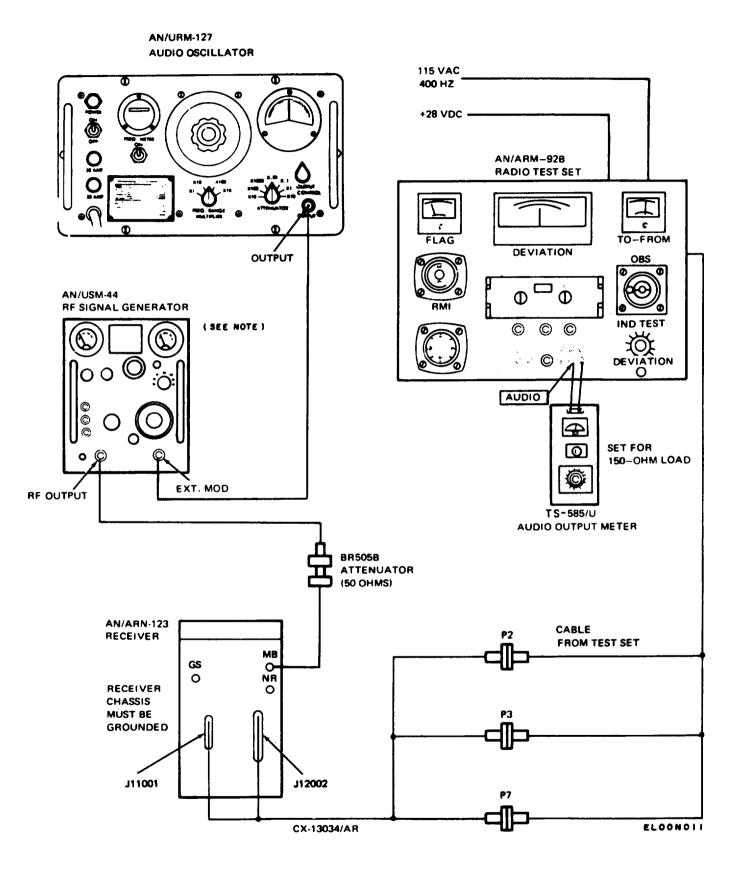
Figure 3-3. Bench Test Setup, Marker.
