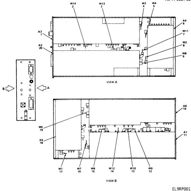
Figure 1. Receiver, Radio R924, 10-156287-1
