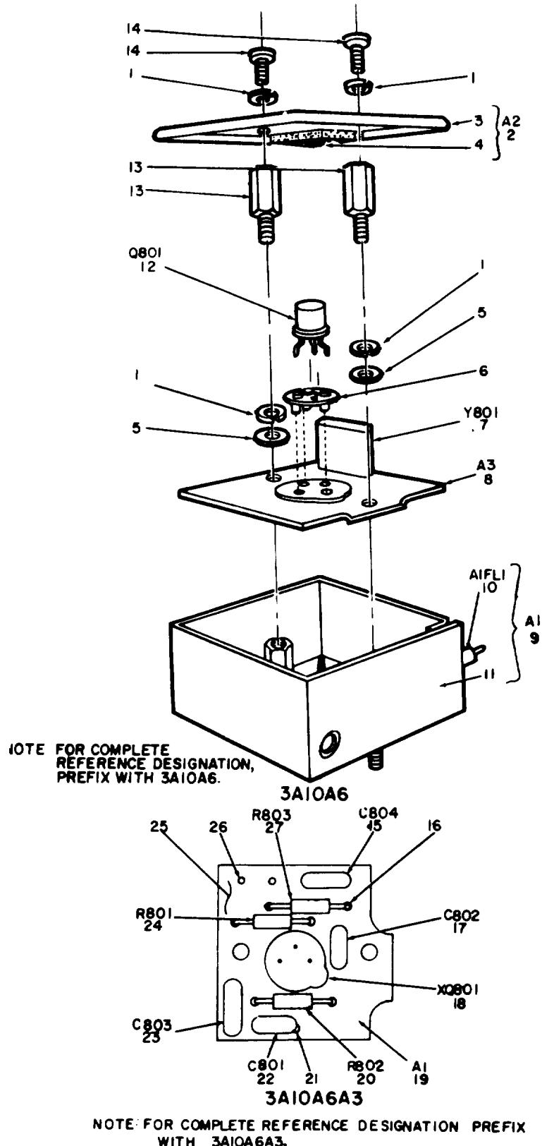
Figure 20. 3.045 MHz Oscillator Subassembly (3A10A6) and 3.045 MHz Oscillator Circuit Card Assembly (3A10A6A3).
