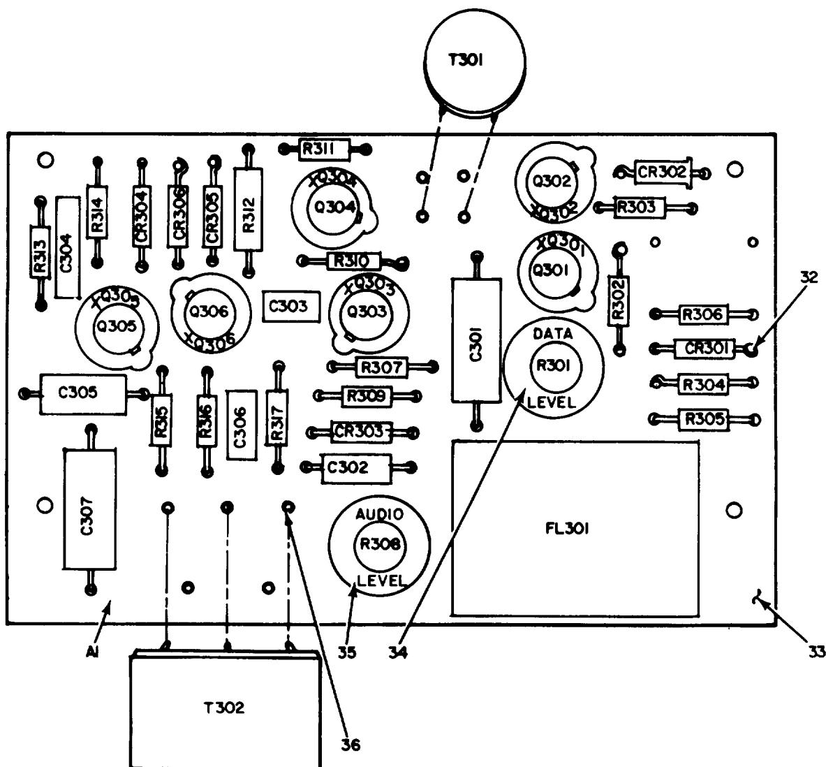
Figure 22. Squelch and Receiver Audio Subassembly (3A10A8) (Sheet 1 of 2).
