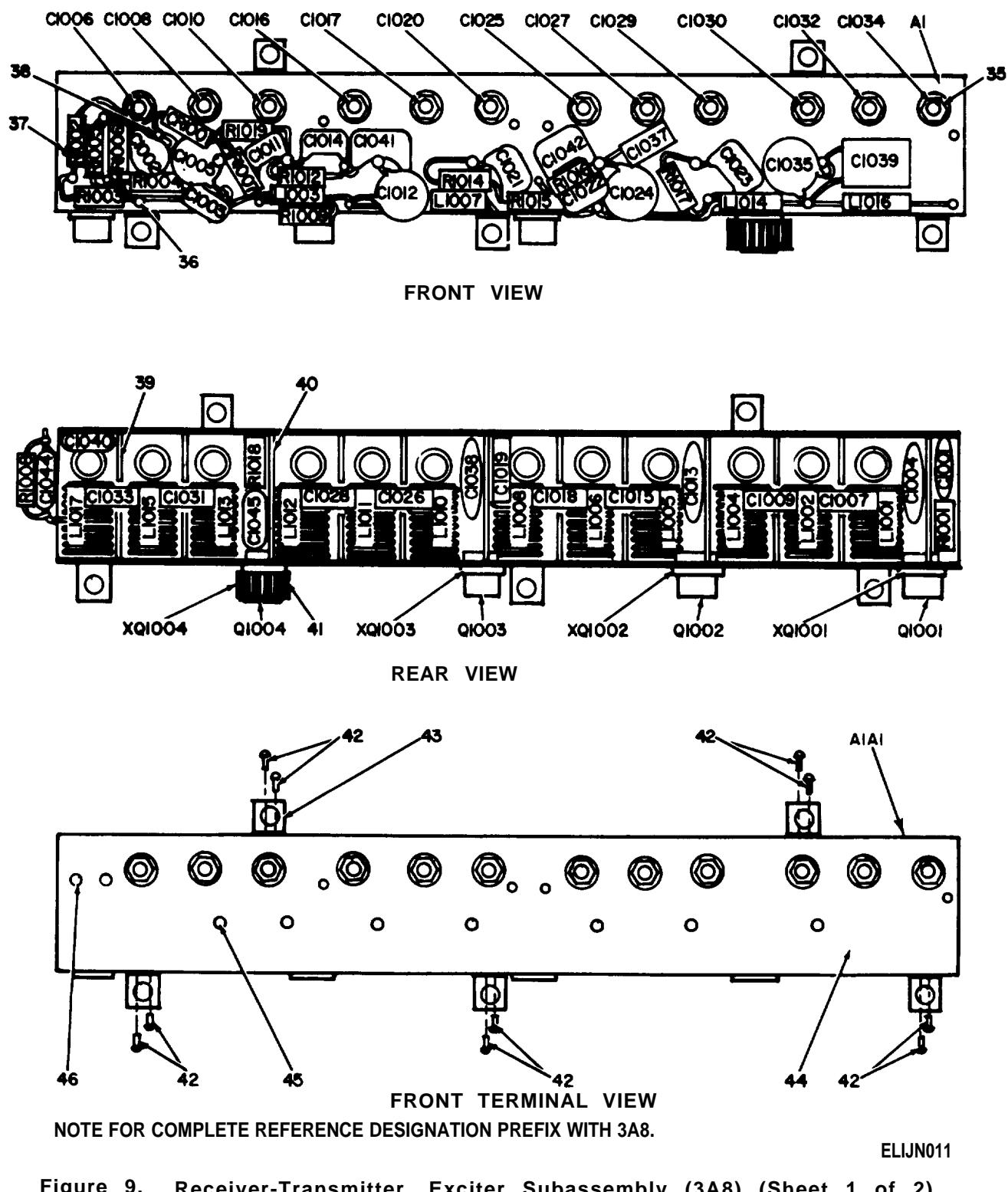
Figure 9. Receiver-Transmitter, Exciter Subassembly (3A8) (Sheet 1 of 2).
