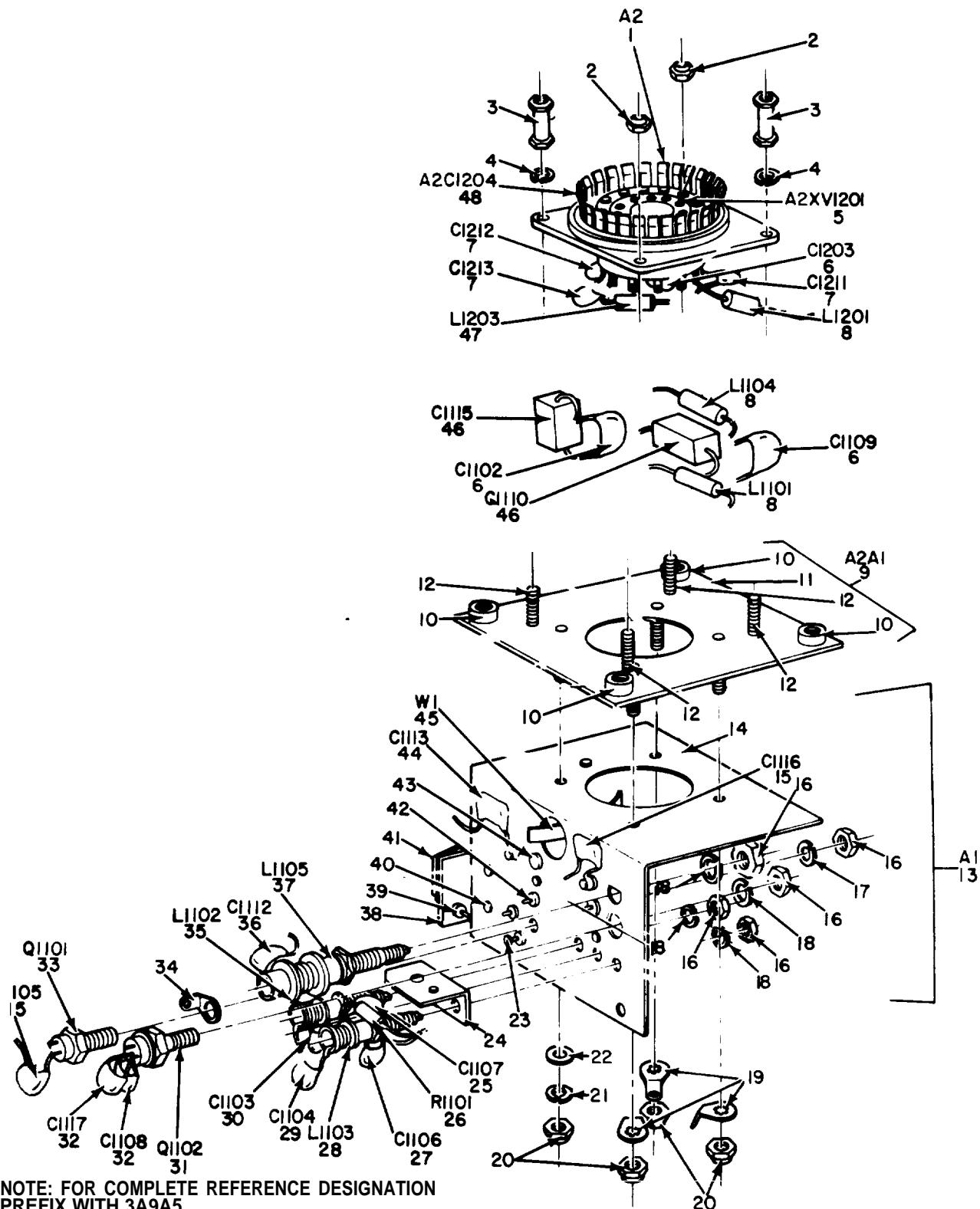
Figure 12. Driver Assembly (3A9A5).
