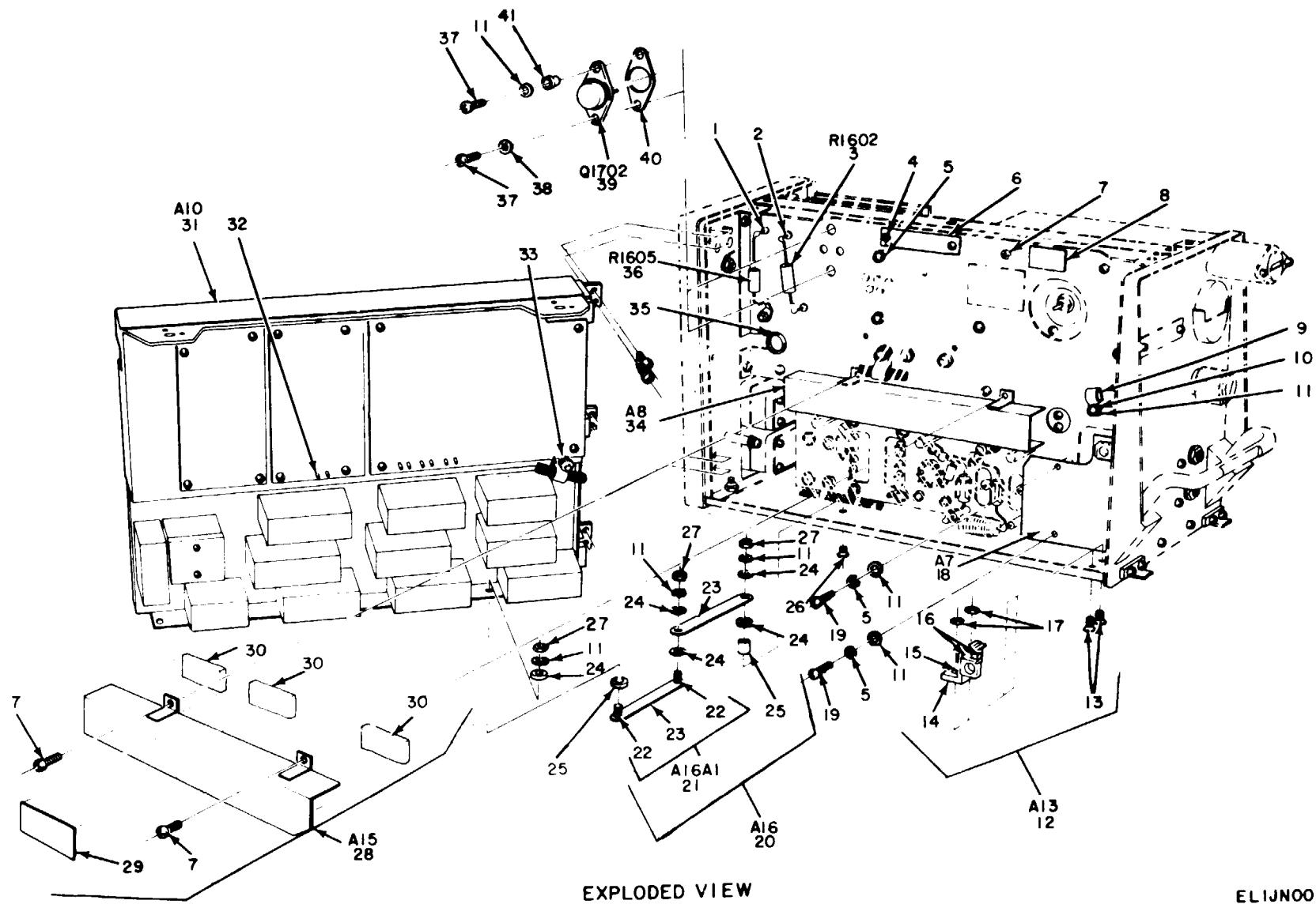
Figure 3. Receiver-Transmitter, Radio RT-857/ARC-134, Left Side View (Sheet 1 of 2).
