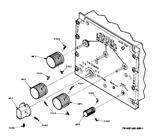
Figure 1. AN/ARC-116 Panel Assembly.
