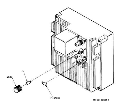
Figure 2. AN/A RC- 116 Rear Assembly
