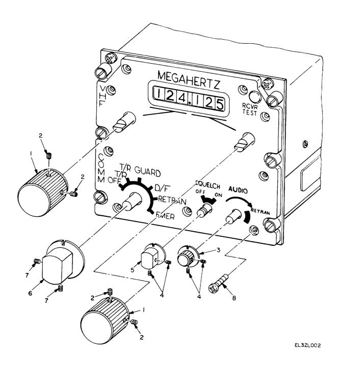
Figure 2. Panel Assembly, Radio Set AN/ARC-115A(V)l.
