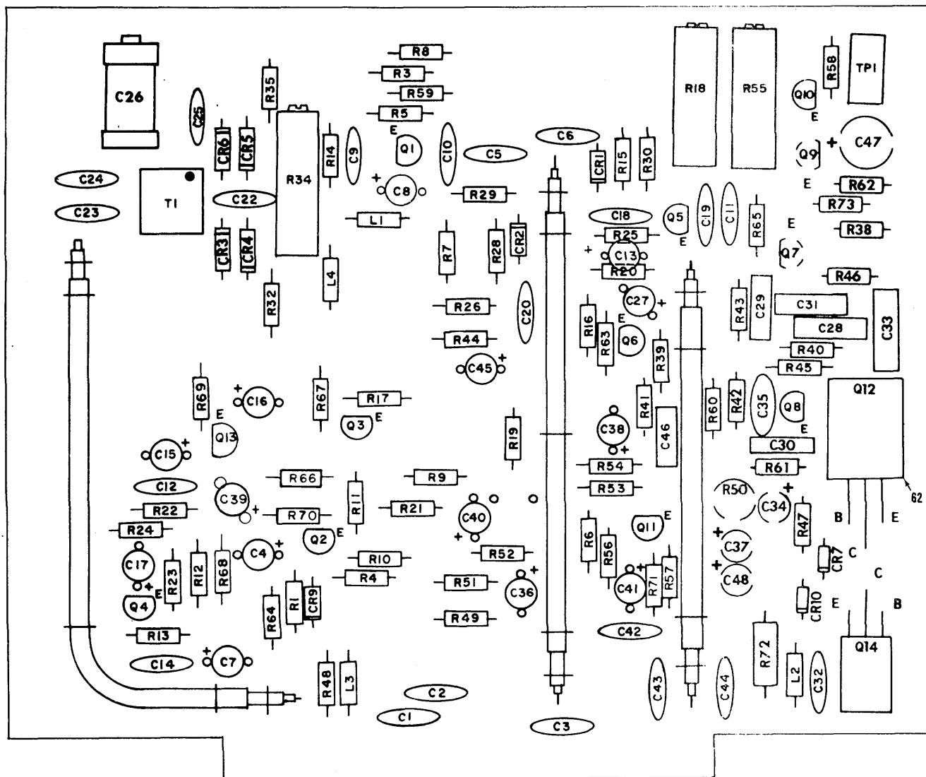
Figure 17. Sideband Generator Circuit Card Assembly (sheet 1 of 2).
