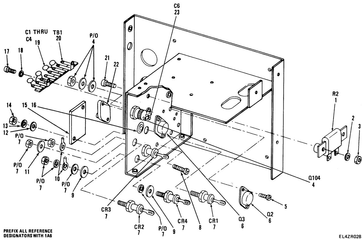
Figure 20. Power Supply Assembly, Chassis, Exploded View.
