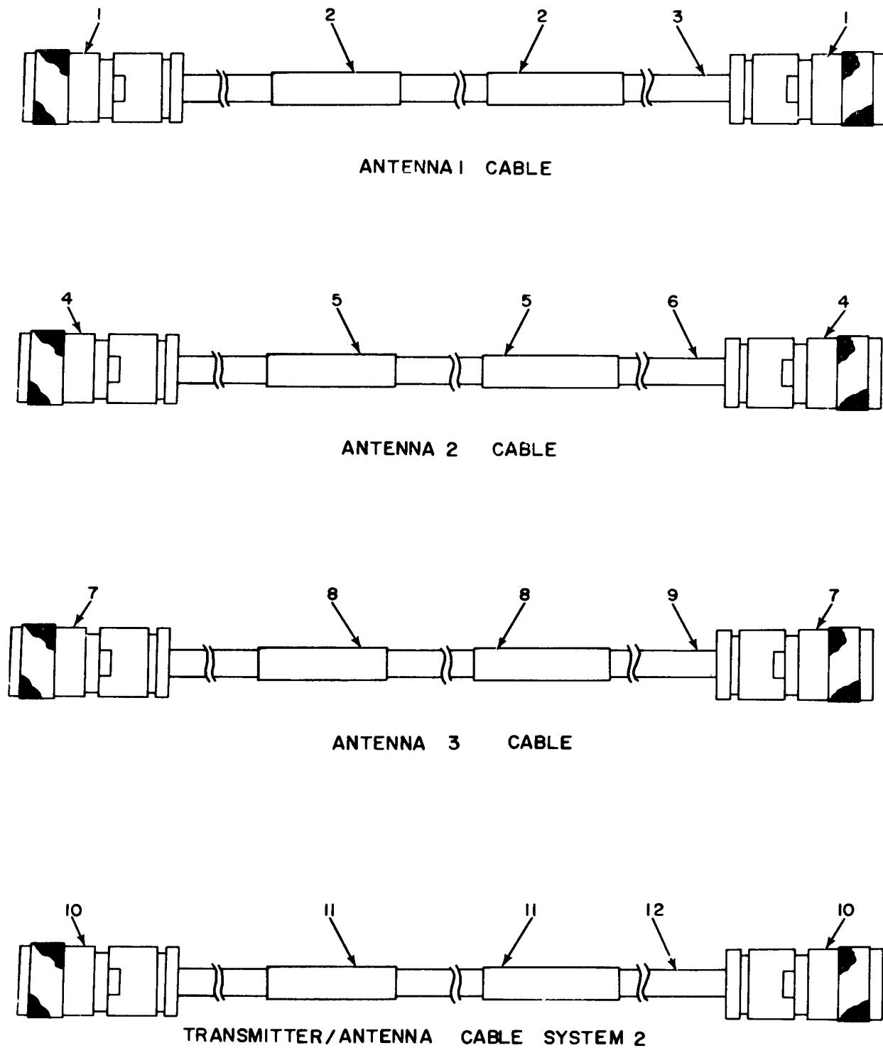
Figure 33. Cable Assemblies, Antenna GP1, GP2, GP3, and GP9.
