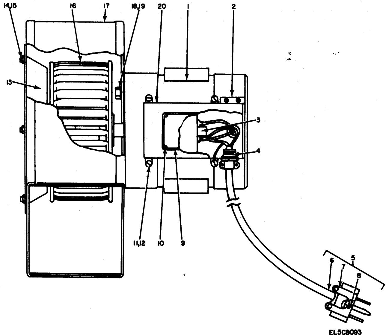
Figure 58. Blower Assembly, Curbside.
