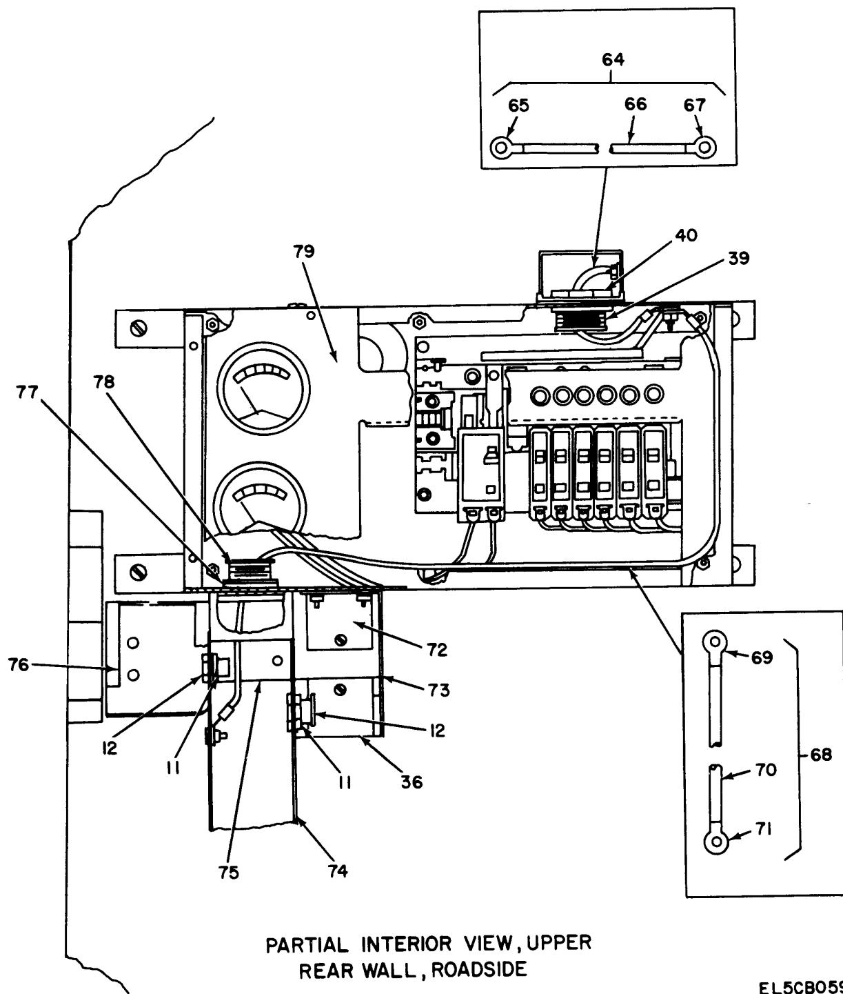
Figure 36. Utilities Installation, Raceway (Sheet 5 of 6).
