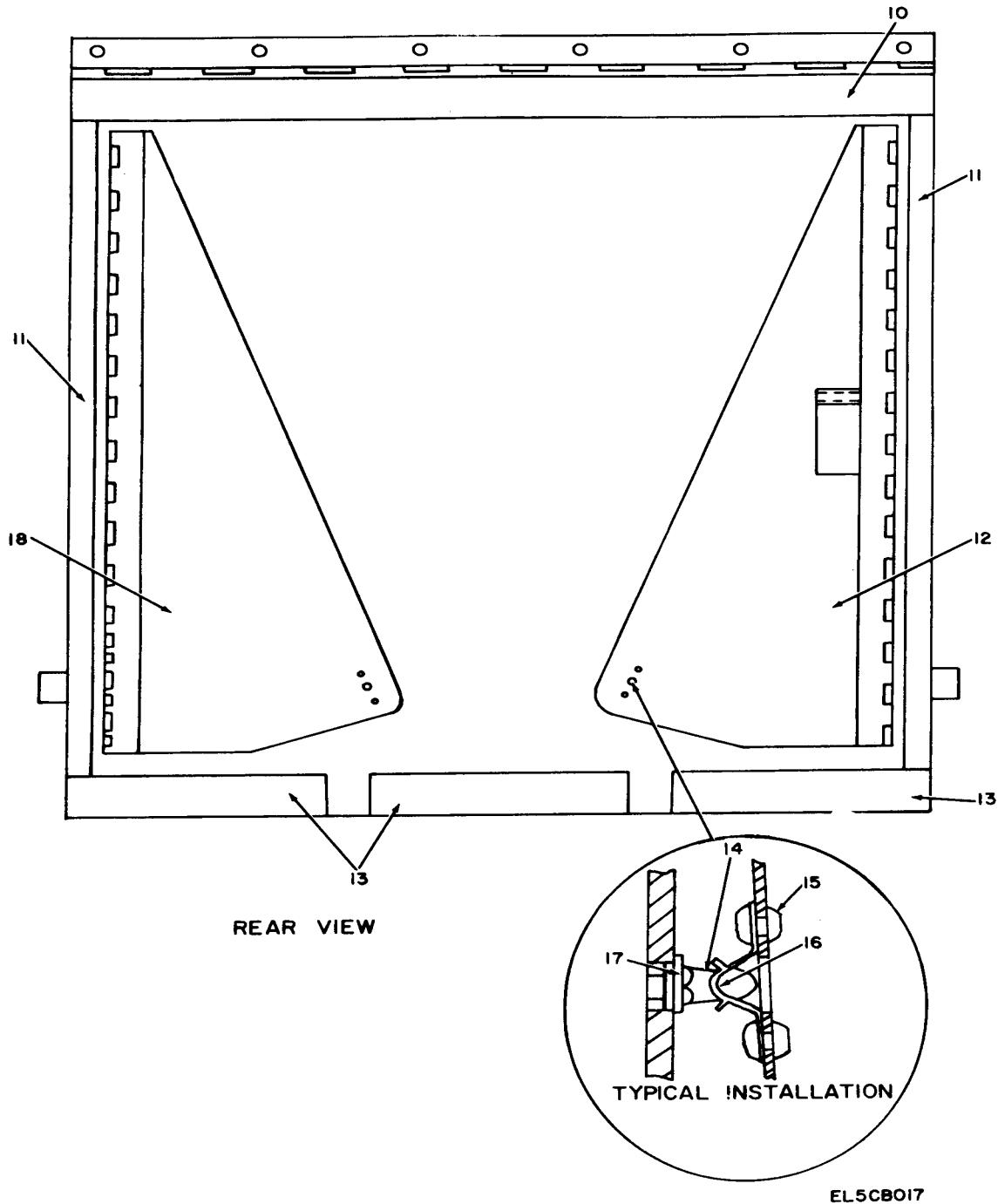
Figure 11. Shelter, Electrical Equipment S-298A/TRC-110(V), Cover, Power and Signal Entrance (Sheet 2 of 2).
