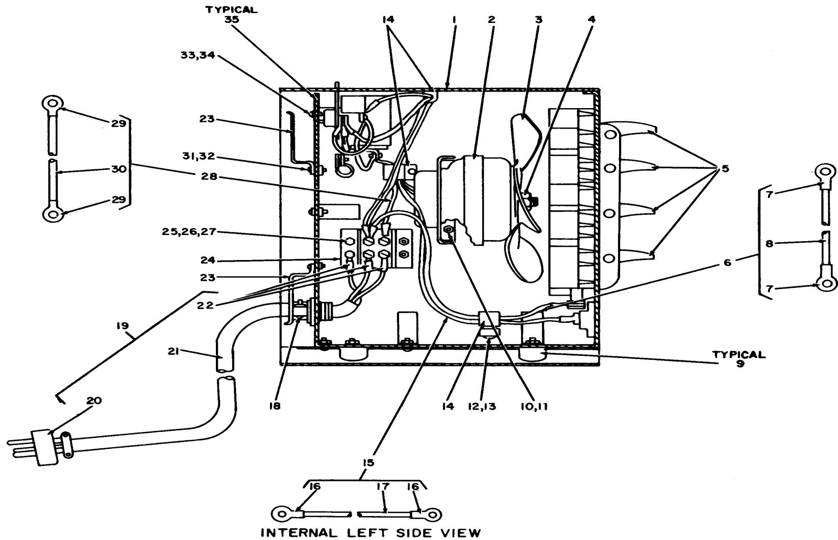
Figure 22. Heater, Space, Electrical (Sheet 1 of 3).
