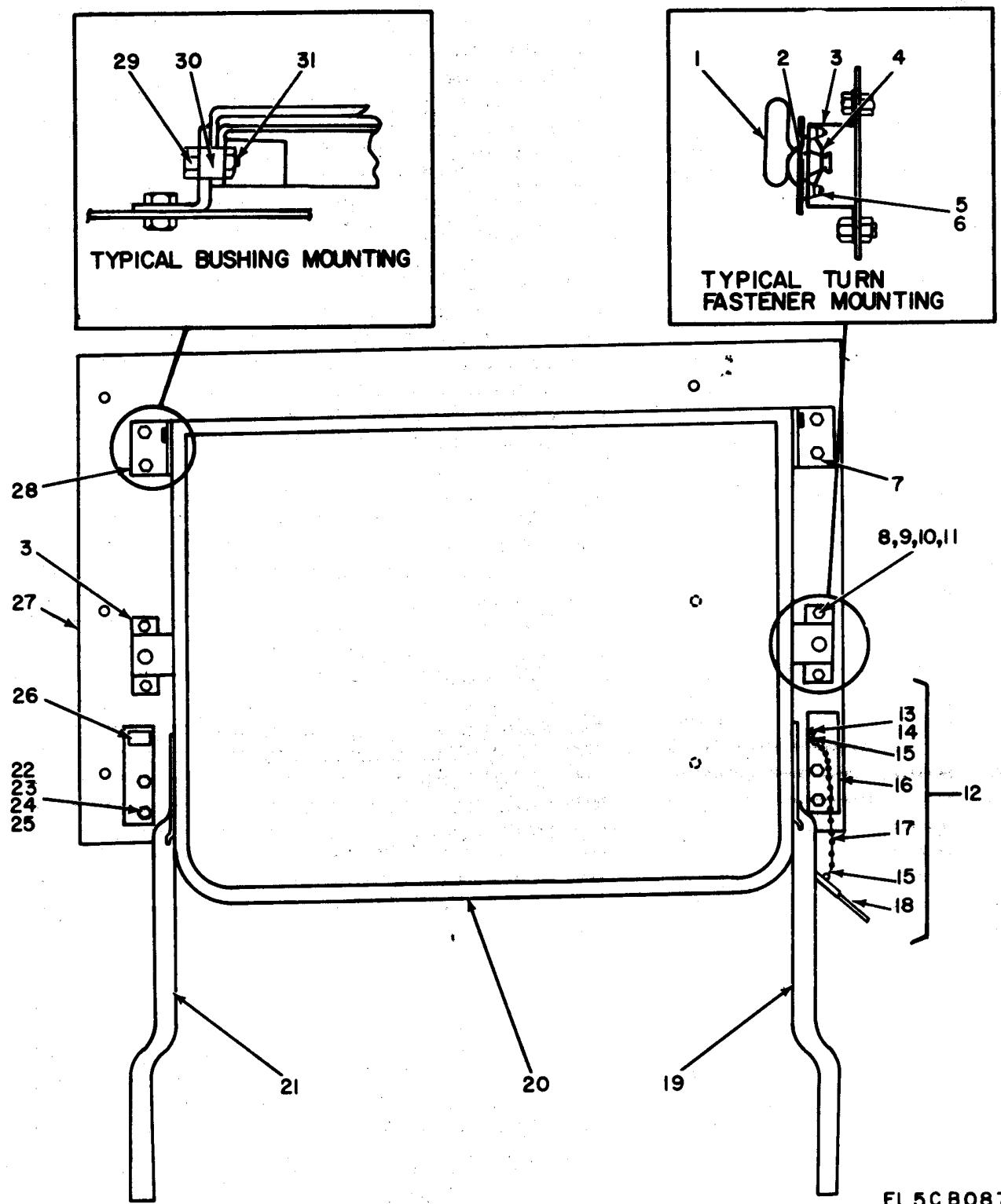
Figure 54. Bracket Installation, Table Assembly.
