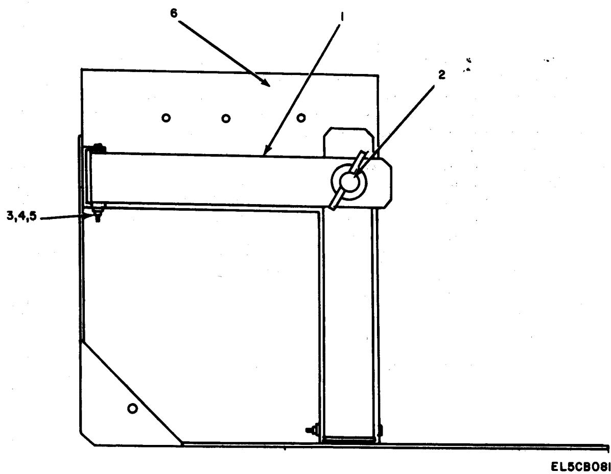
Figure 50. Bracket Installation, Cable Reel Hold-Down Assembly.
