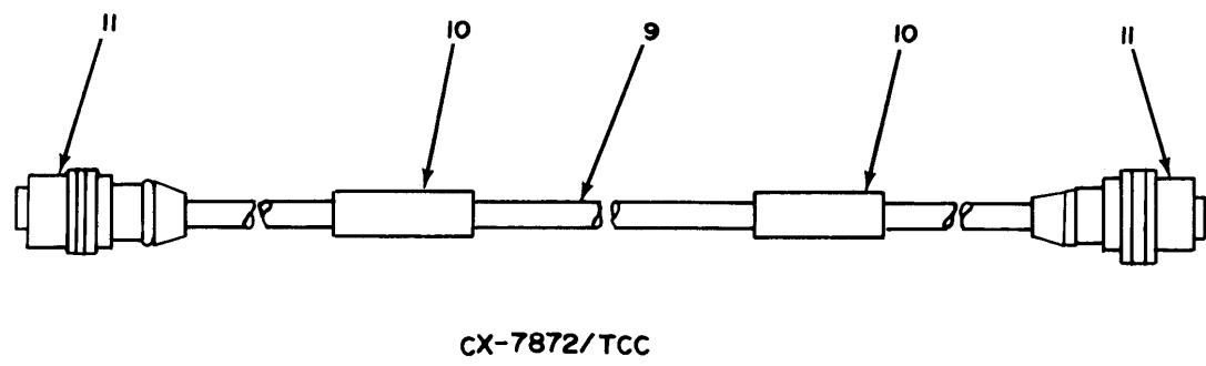
Figure 19. Cable Assembly, Radio Frequency CG-1040B/U (5 FT 0 IN), Cable Assemblies, Special Purpose, Electrical CX-7875/TCC (7 FT 0 IN) and CX-7872/TCC (5 FT 0 IN).
