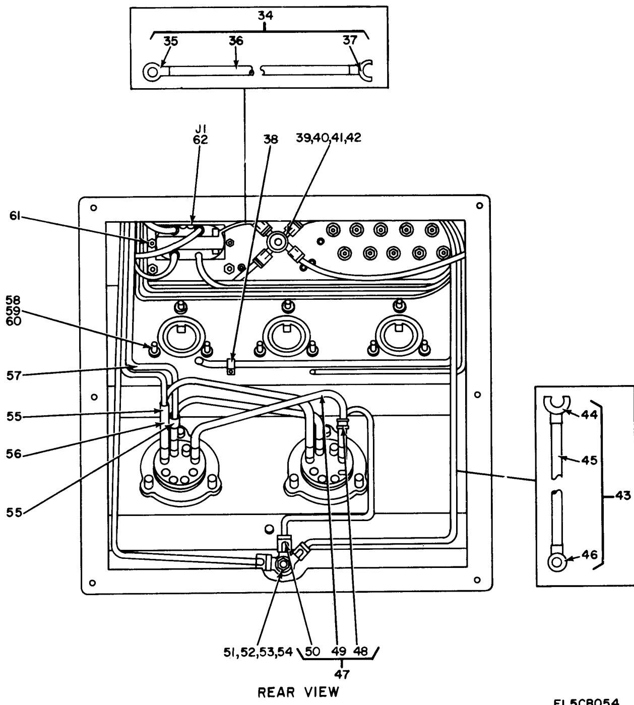
Figure 35. Power and Signal Entrance (Sheet 2 of 2).
