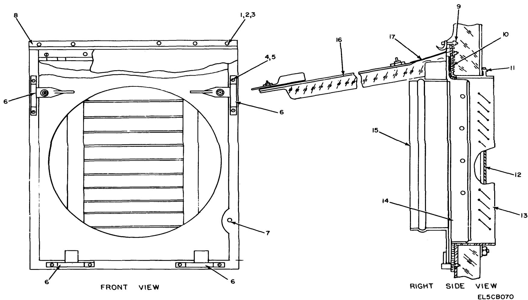
Figure 40. Bracket Installation, S-330(B) Shelter Air Conditioner Adapter Installation.
