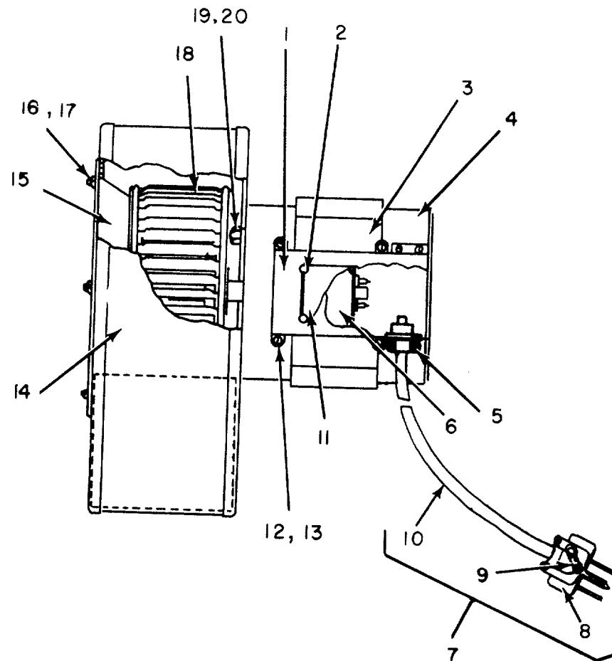
Figure 26. Exhaust Blower Installation, Blower Assembly (CCW), Roadside.
