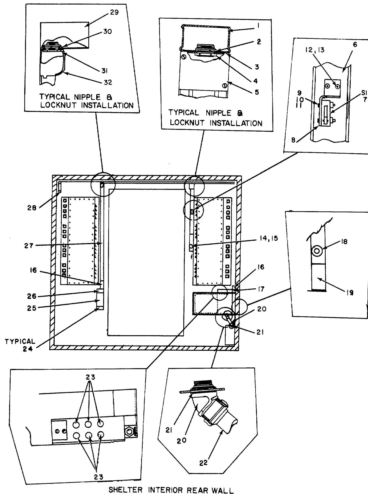
Figure 20. Utilities Installation, Raceway (Sheet 1 of 5).
