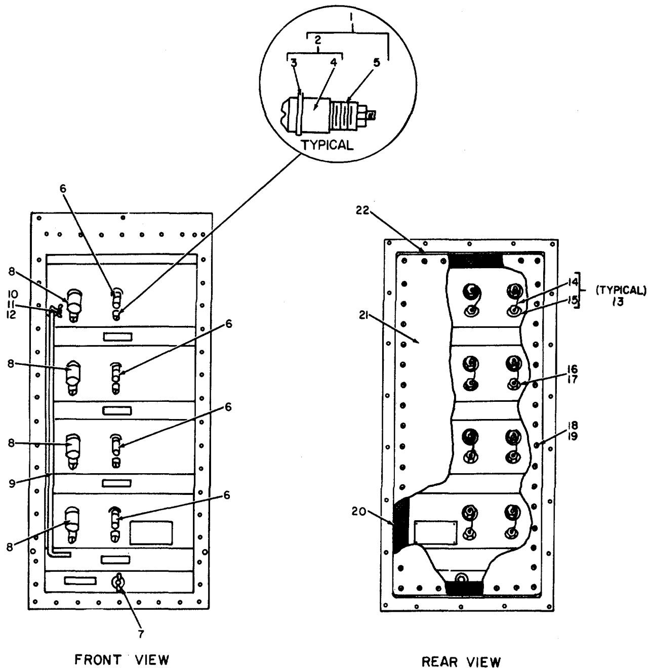
Figure 37, Video Entrance Box, Exterior Cover Removed.
