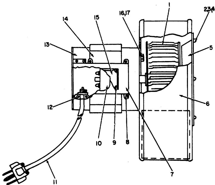
Figure 28. Exhaust Blower Installation, Blower Assembly (CW), Curbside.
