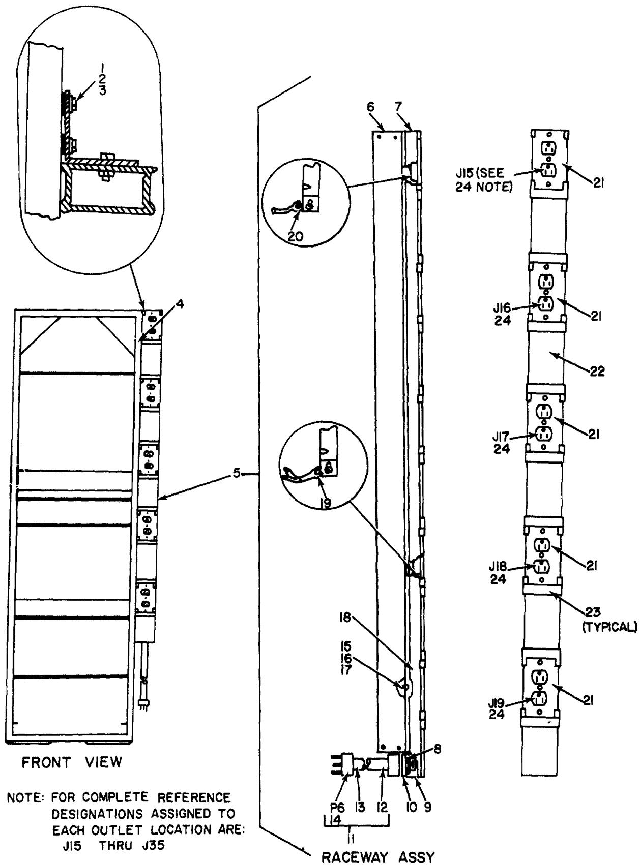
Figure 18. Utilities Installation, Electrical, Rack Assembly, System 3, 6 and 8.
