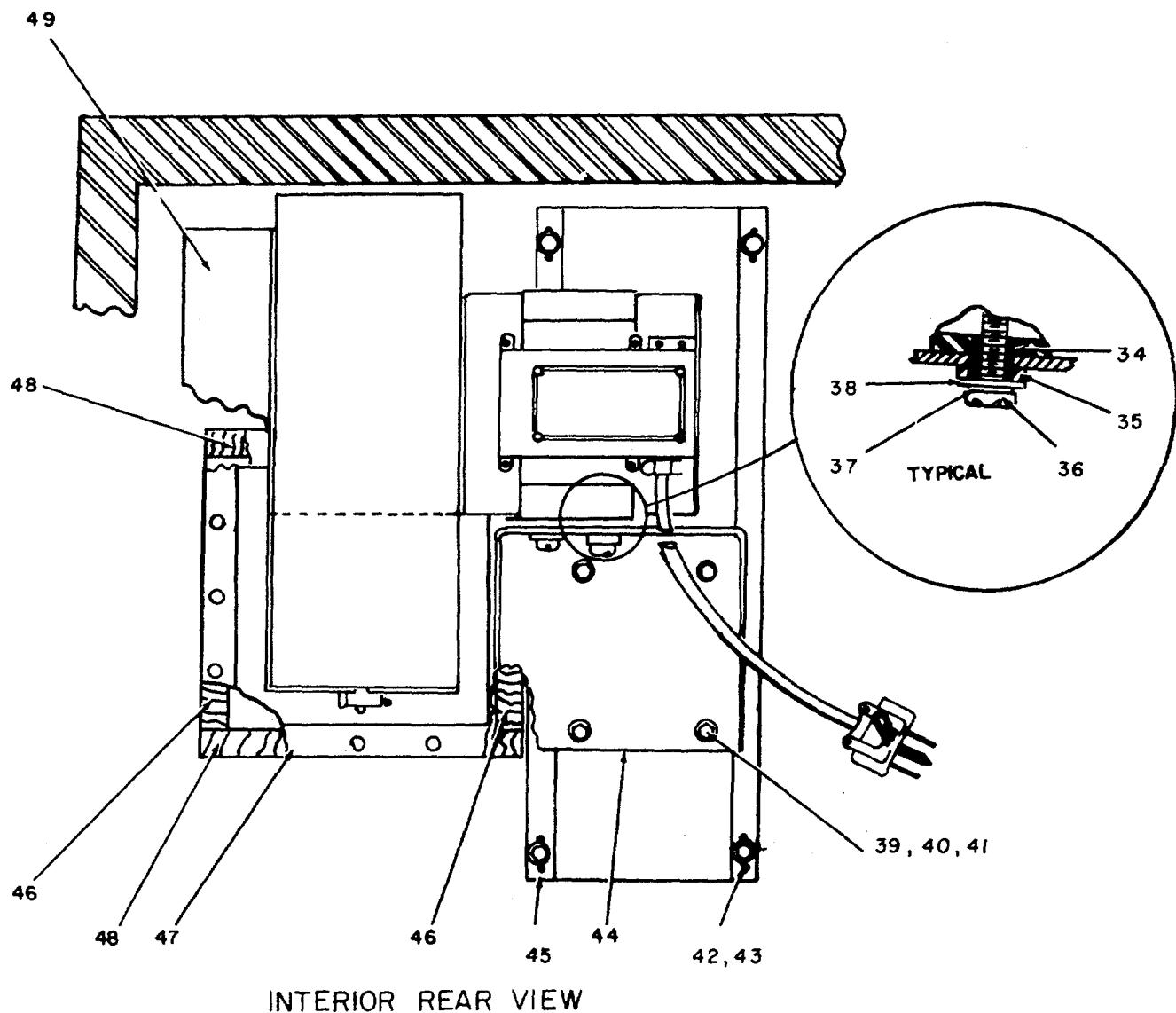
Figure 25. Exhaust Blower Installation, Roadside Wall (sheet 2 of 2).
