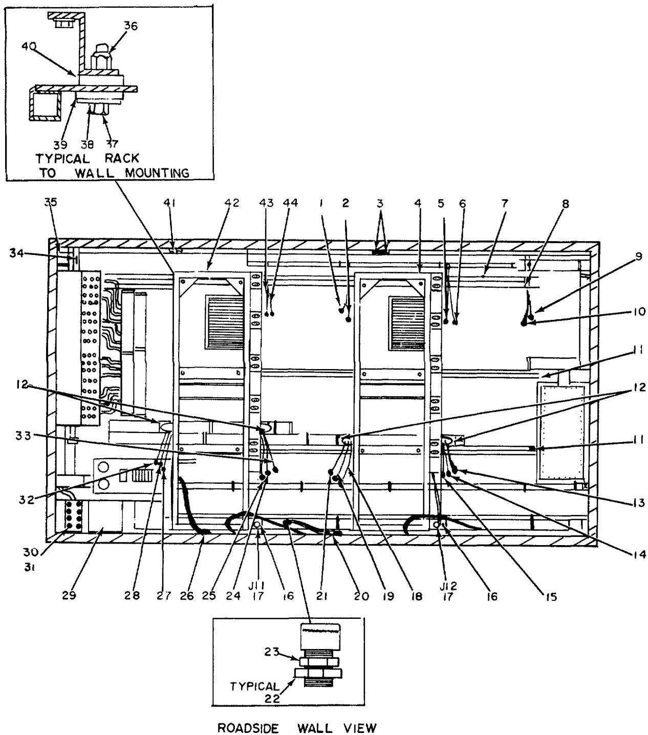
Figure 12. Utilities Installation, Electrical, Shelter, Interior Walls, (Sheet 1 of 2)
