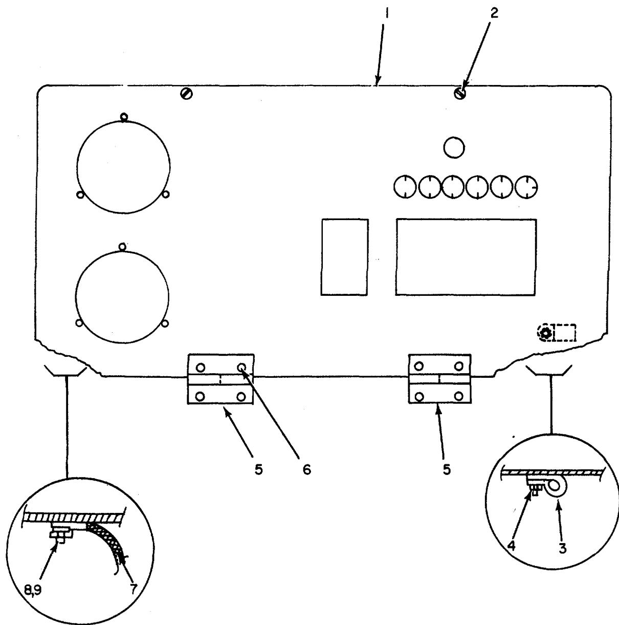
Figure 44. Power Distribution Panel, Cover Assembly.
