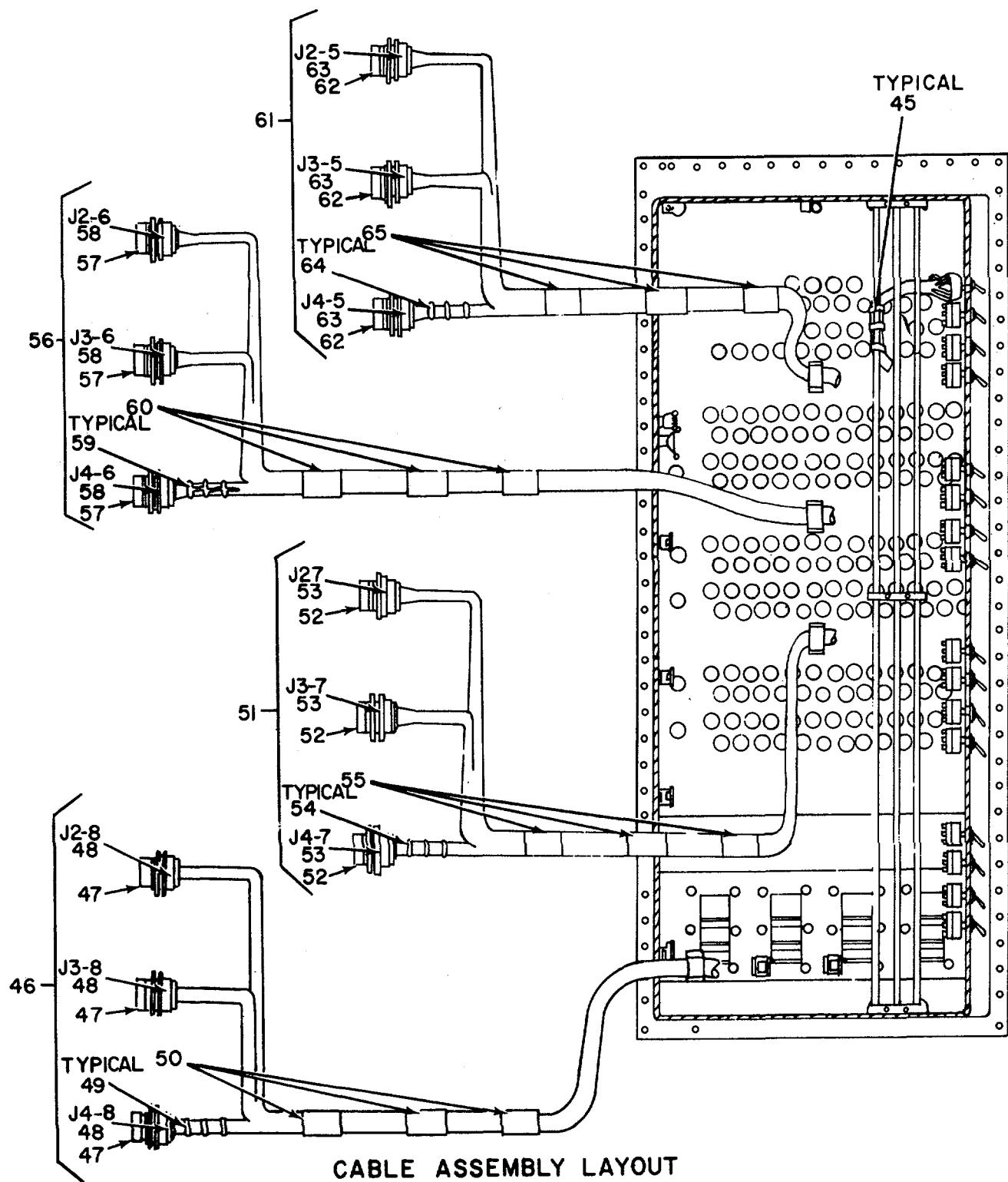
Figure 41. Signal Entrance Box, Curbside Installation (Sheet 4 of 4)
