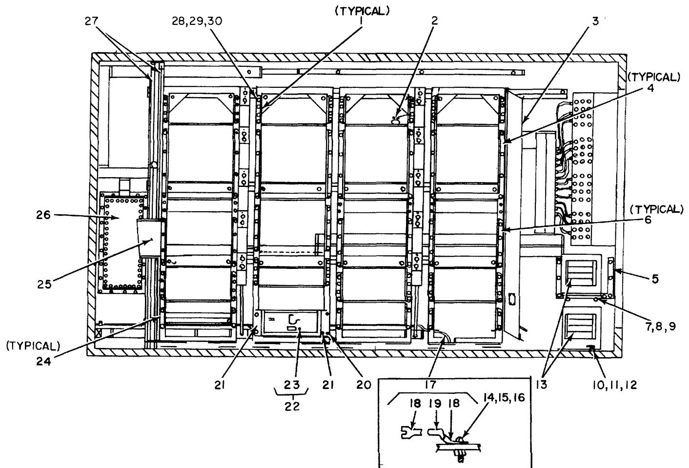
Figure 2. Shelter, Electrical Equipment S-301/TCC-61 (Sheet 1 of 2).
