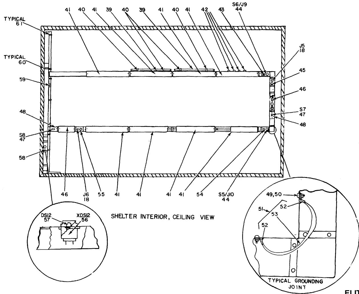
Figure 11. Utilities Installation, Electrical (Sheet 3 of 3).
