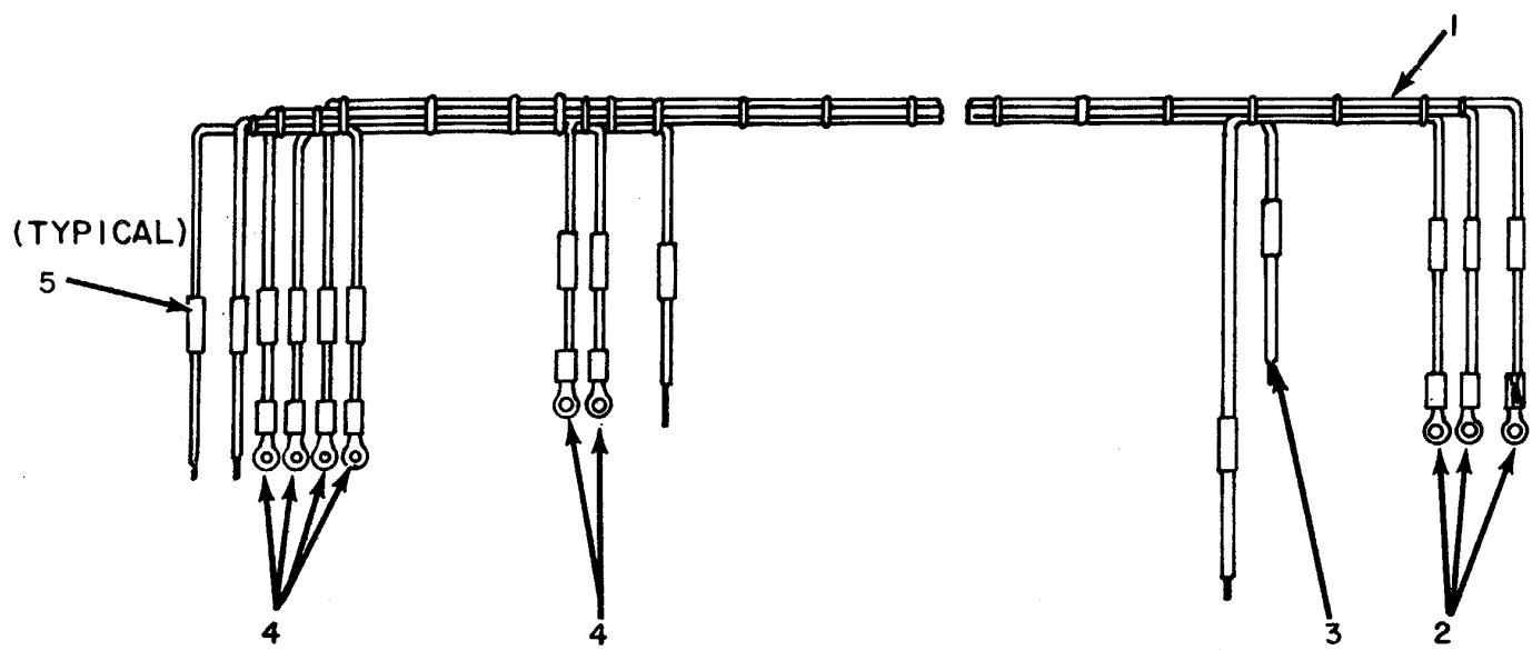
Figure 47. Overvoltage Protective Device, Harness Assembly.
