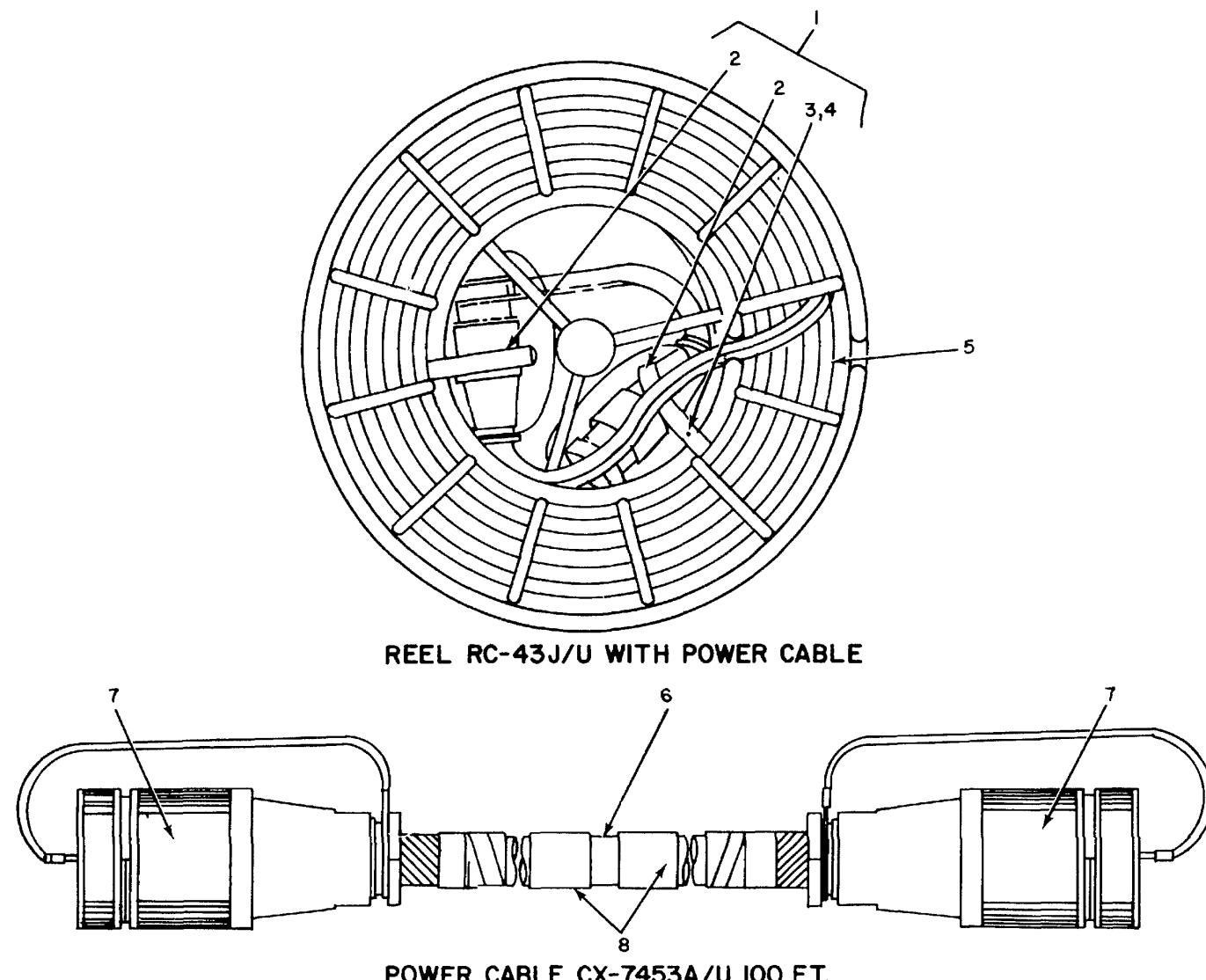
Figure 31. Cable Assembly, Power and Reel.
