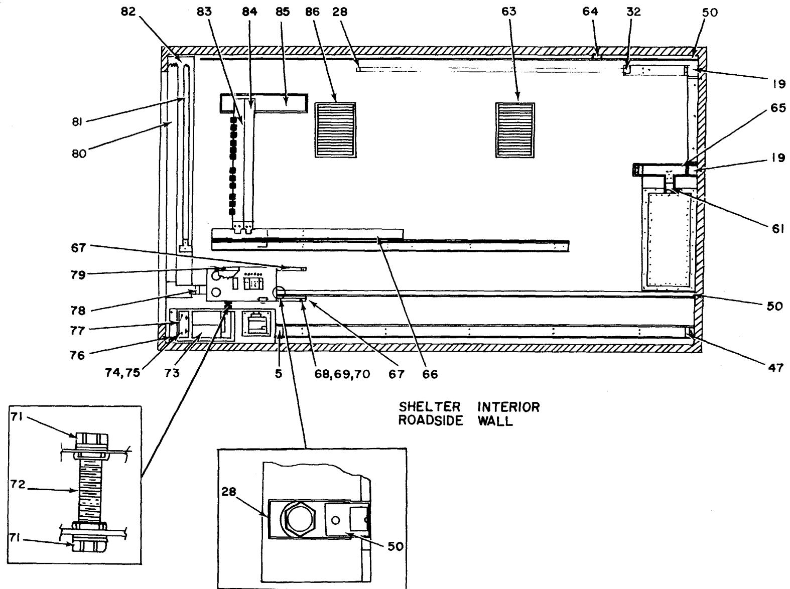
Figure 20. Utilities Installation, Raceway (sheet 5 of 5).
