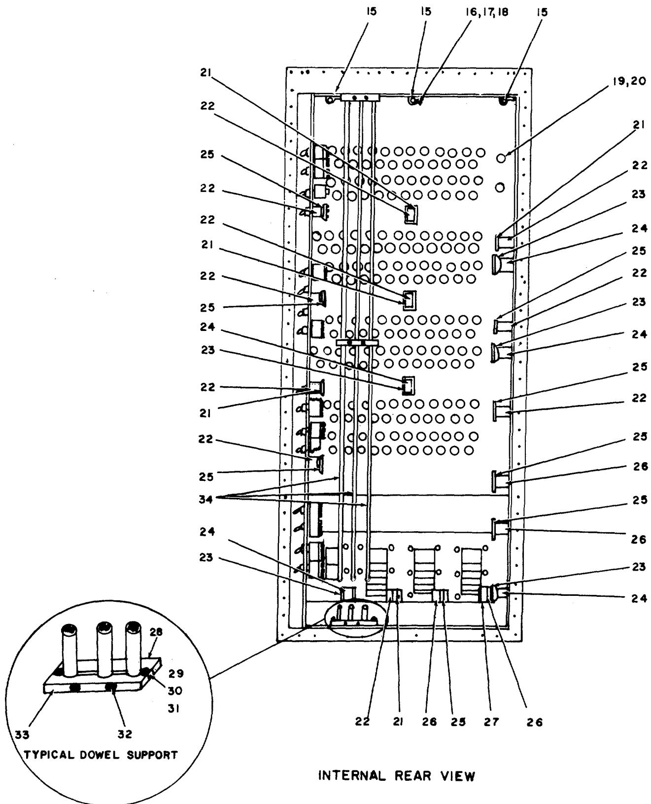
Figure 40. Signal Entrance Box, Roadside Installation (Sheet 2 of 4).
