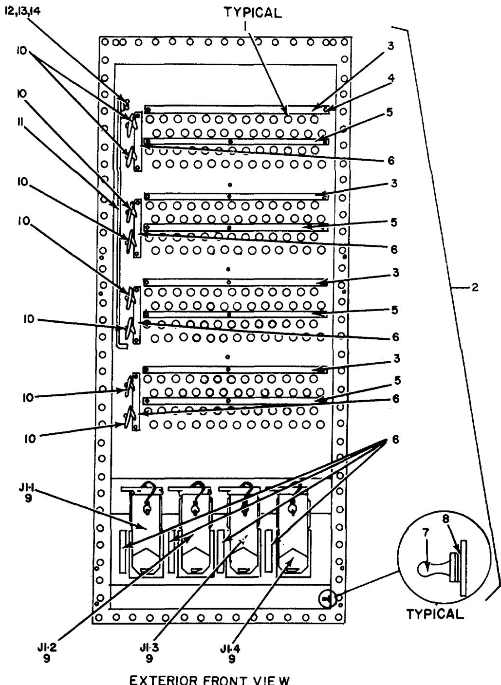
Figure 40. Signal Entrance Box, Roadside Installation (Sheet 1 of 4).
