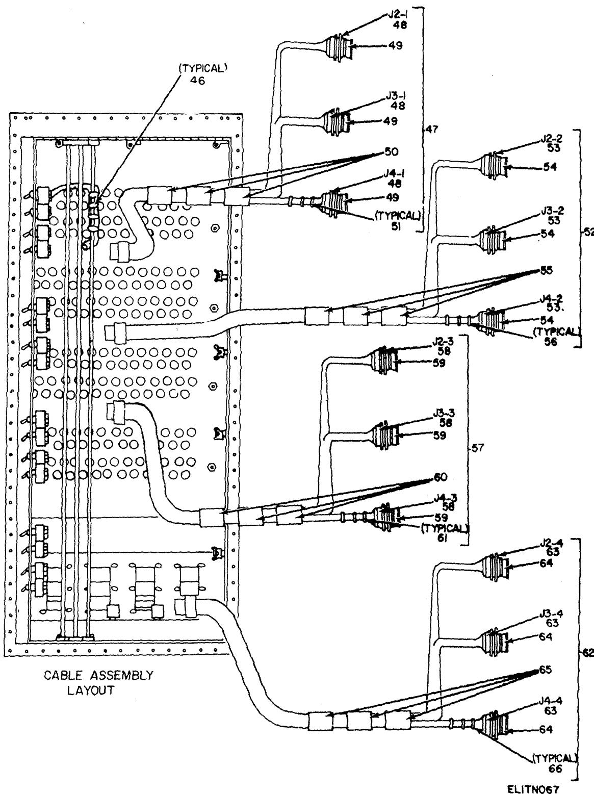
Figure 40. Signal Entrance Box, Roadside Installation (Sheet 4 of 4).
