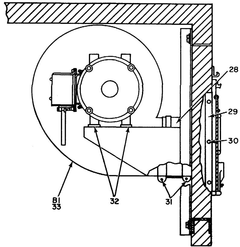
Figure 25. Exhaust Blower Installation, Roadside Wall (sheet 1 of 2).
