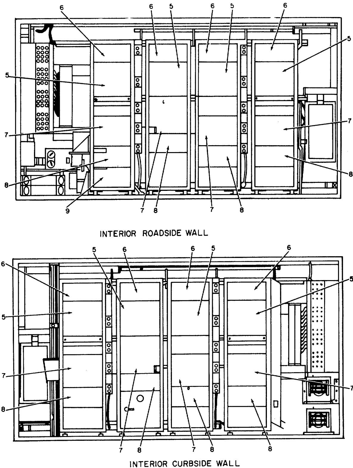
Figure 1. Terminal Set, Telephone AN/TCC-61 (Sheet 2 of 2).
