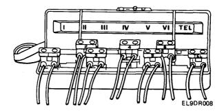
Connect the incoming lines to the adapters with the designation strip facing the operator.
