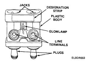
CONNECTOR ADAPTER. A combination jack and plug that fits into the jacks of other adapters, allowing for line-to-line or conference calls. The plugs, which are thumb-screws, secure telephone lines at the line terminal points through clamping force. A glow lamp seated inside the adapter's clear-plastic body will light when an incoming call is received. A designation strip painted on the body of the adapter allows the operator to designate terminal lines in writing.
