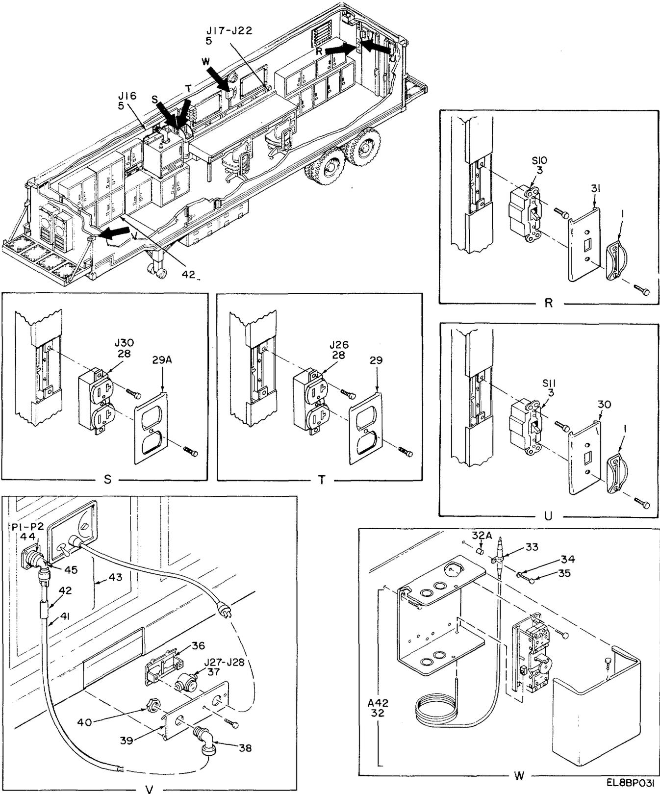
Figure 3. Electrical Installation (Sheet 3 of 6).
