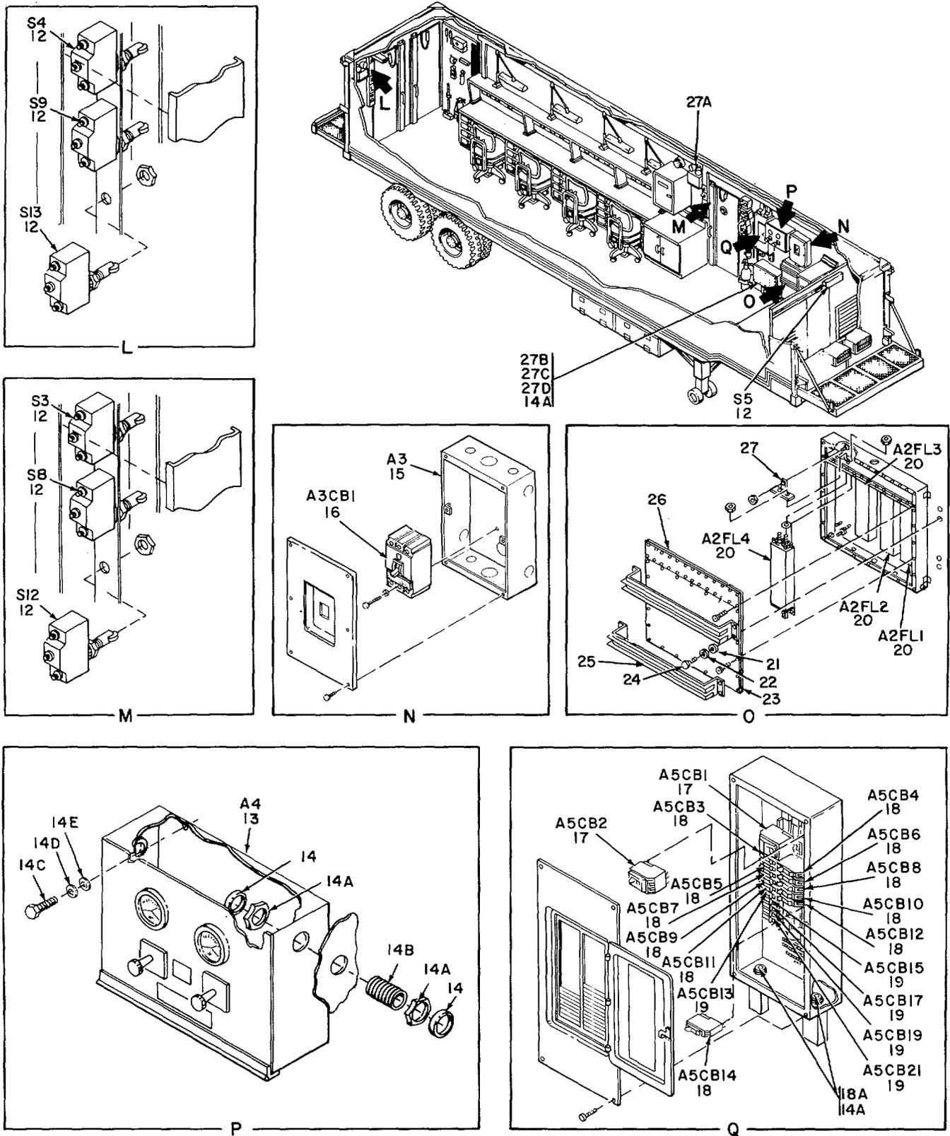
Figure 3. Electrical Installation (Sheet 2 of 6).
