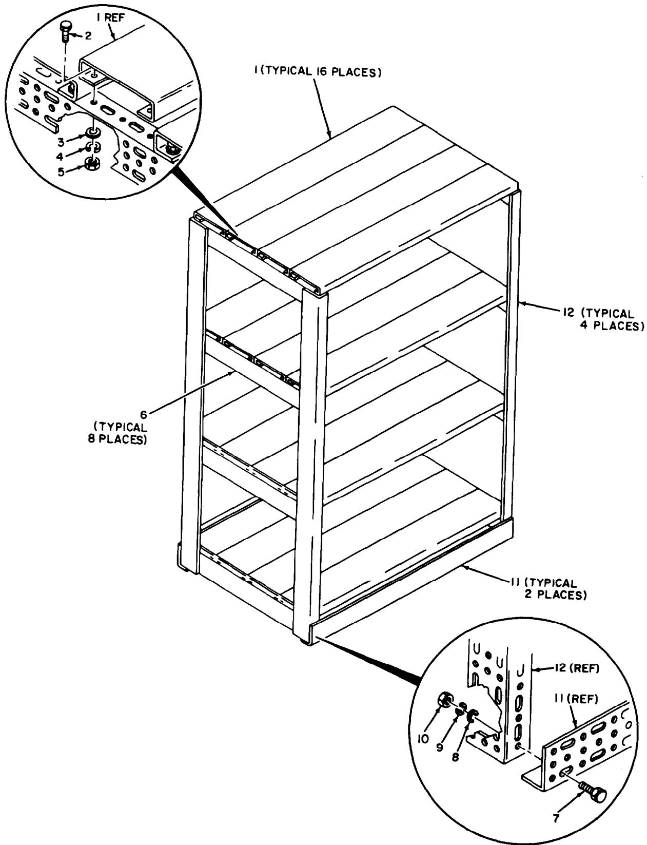
Figure 19. Single Storage Rack Assembly, P/N SMD593523-1.
