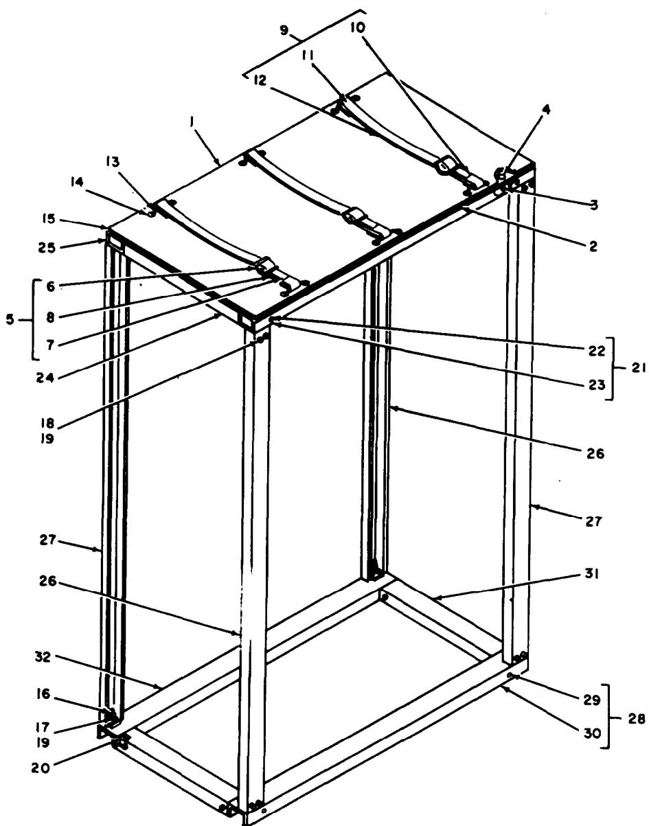
Figure 17. Cabinet Frame Assembly, P/N SMD593411-1.
