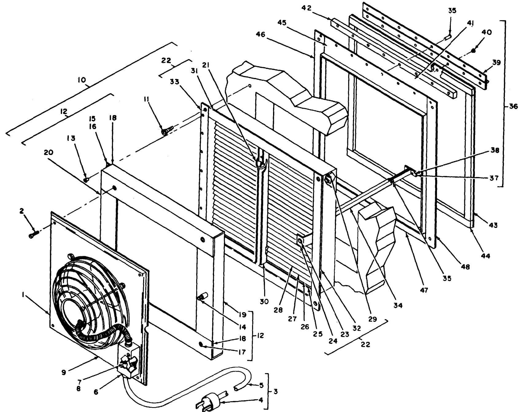
Figure 27. Exhaust Fan Assembly.
