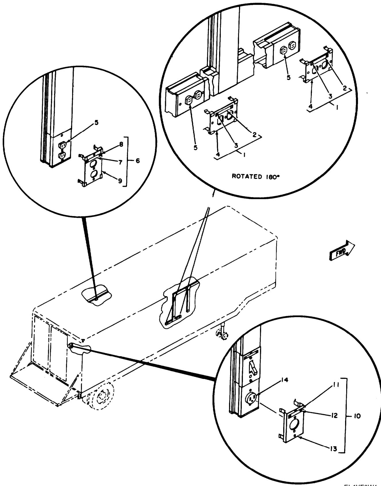
*Figure 32. Electrical Receptacle Installation*
