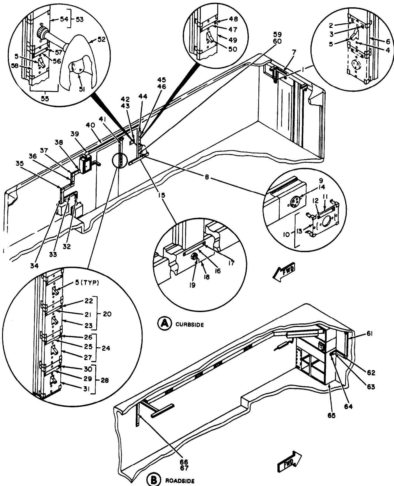
Figure 9. Electrical Components Installation.
