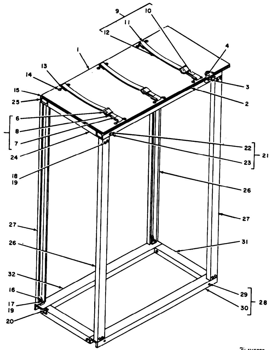
Figure 18. Cabinet Frame Assembly, P/N SMD593411-2.
