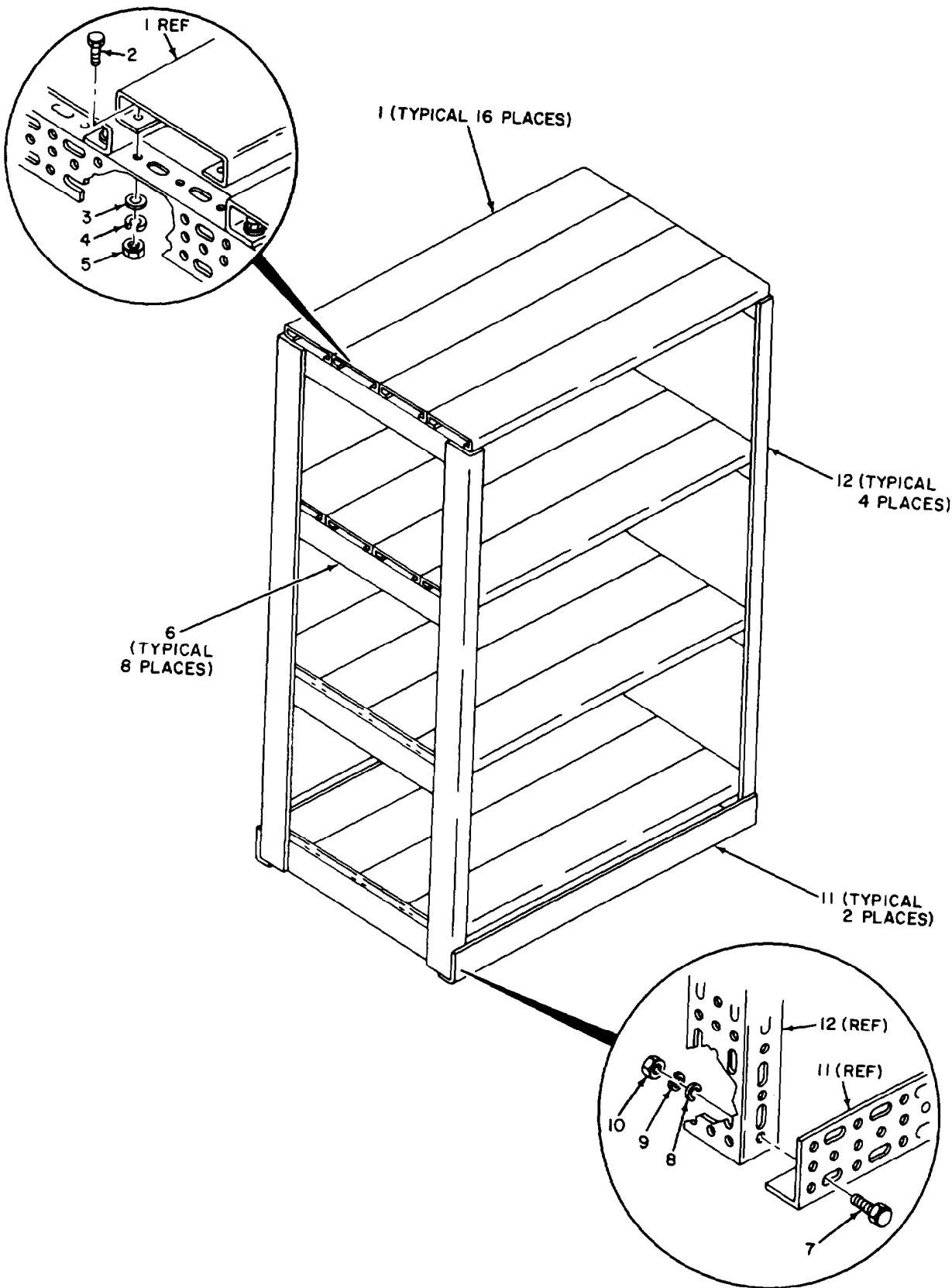
Figure 20. Single Storage Rack Assembly, P/N SMD593523-2.
