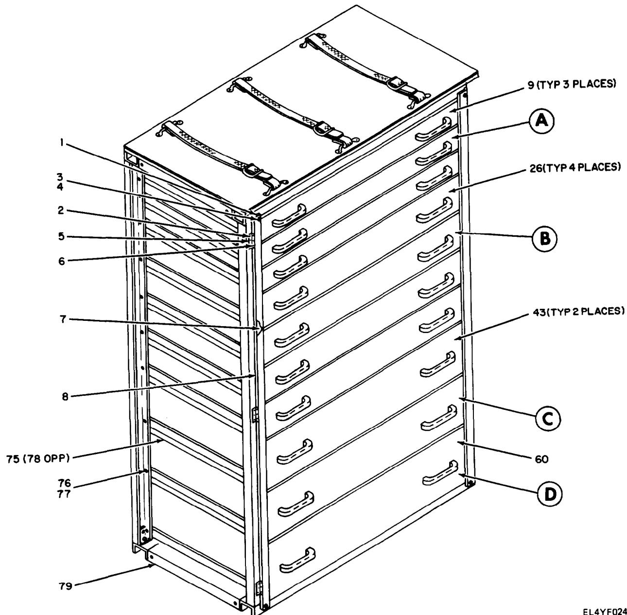
Figure 16. Small Parts Cabinet Assembly, P/N SMD593410-2 (Sheet 1 of 2).
