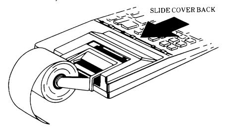
2. Remove the old ink roller by lifting it with the removal tab
