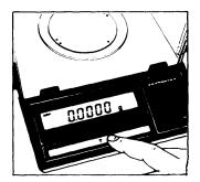
You must zero the display prior to weighing, if you are using a container or if the weight display does not read 0.0000 g (or the equivalent with the weight unit of your choice).
