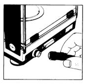
Make the power connection. Secure the connection with the threaded ring. Now connect the power supply unit to a line outlet.
