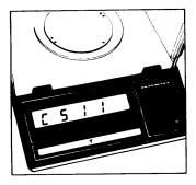
To make changes ("C" mode), press the tare bar when the appropriate code appears.
