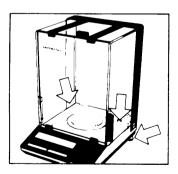
At the point of use, level the balance using the leveling screws (6) such that the air bubble is centered in the circle of the level indicator (5).
