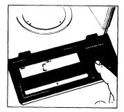
Clear the pan and zero the display. Once the display reads 0.0000 g, push the CAL button (8). The display now reads "C". If YOU get "CE", zero the display and push the CAL button again.
