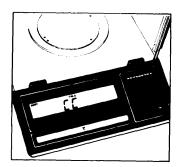
After a few seconds, the display will read "CC", followed by 0.0000 g. A beeper confirms successful completion of calibration.
