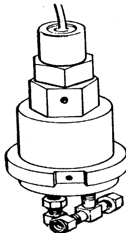
Model 23-4017: Remote mounting, weatherproof, explosion-proof, sample drawing
