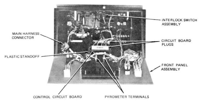
Figure 6. Temp-Master LA With Front Panel Removed (Temp-Master MA is similar)
