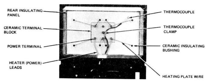
Figure 5. Temp-Master LA And LD (230V) With Upper Rear Panel Removed
