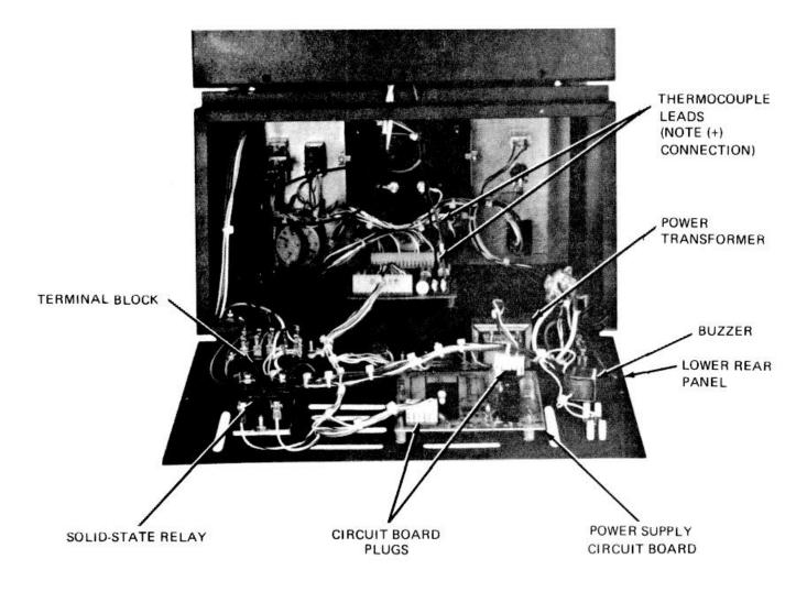
Figure 8. Temp-Master With Lower Rear Panel Removed
