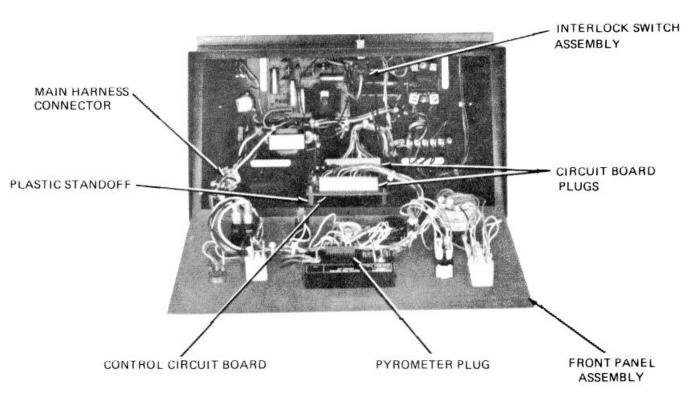
Figure 7. Temp-Master LD With Front Panel Removed (Temp-Master MD is similar)
