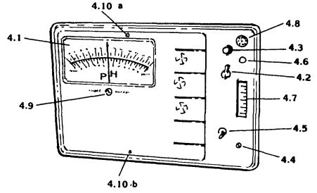
4.1 Analog face-6" mirror-backed analog display for pH and millivolt readings.
