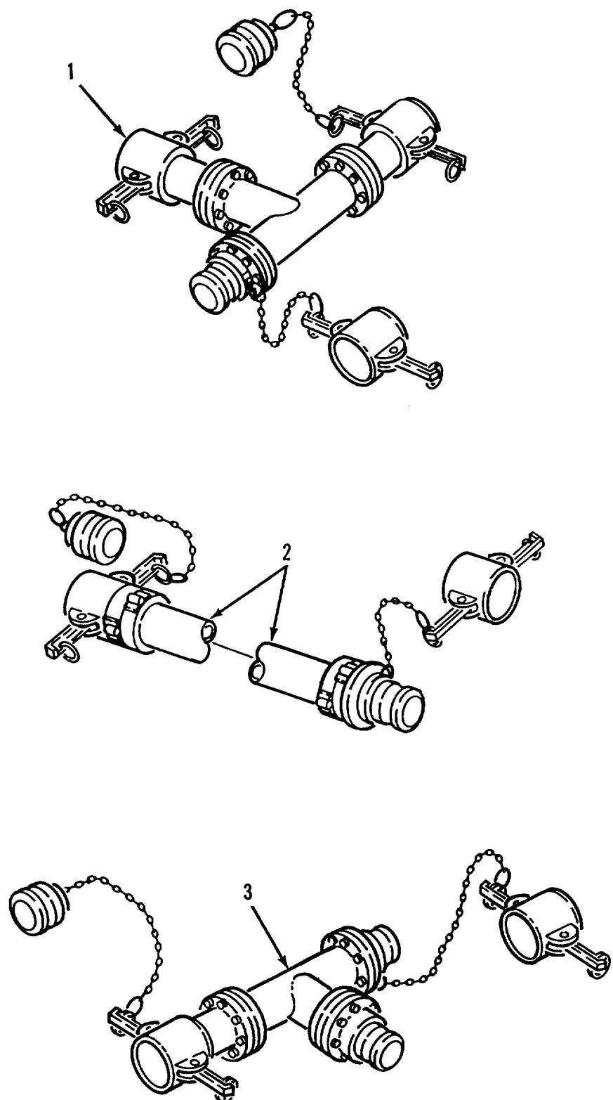
Figure 58. Discharge Hose Interconnection Kit, 4 Inch
