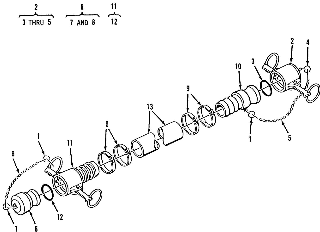
Figure 54. Hose Assembly, Suction, Potable Water, 4 Inch
