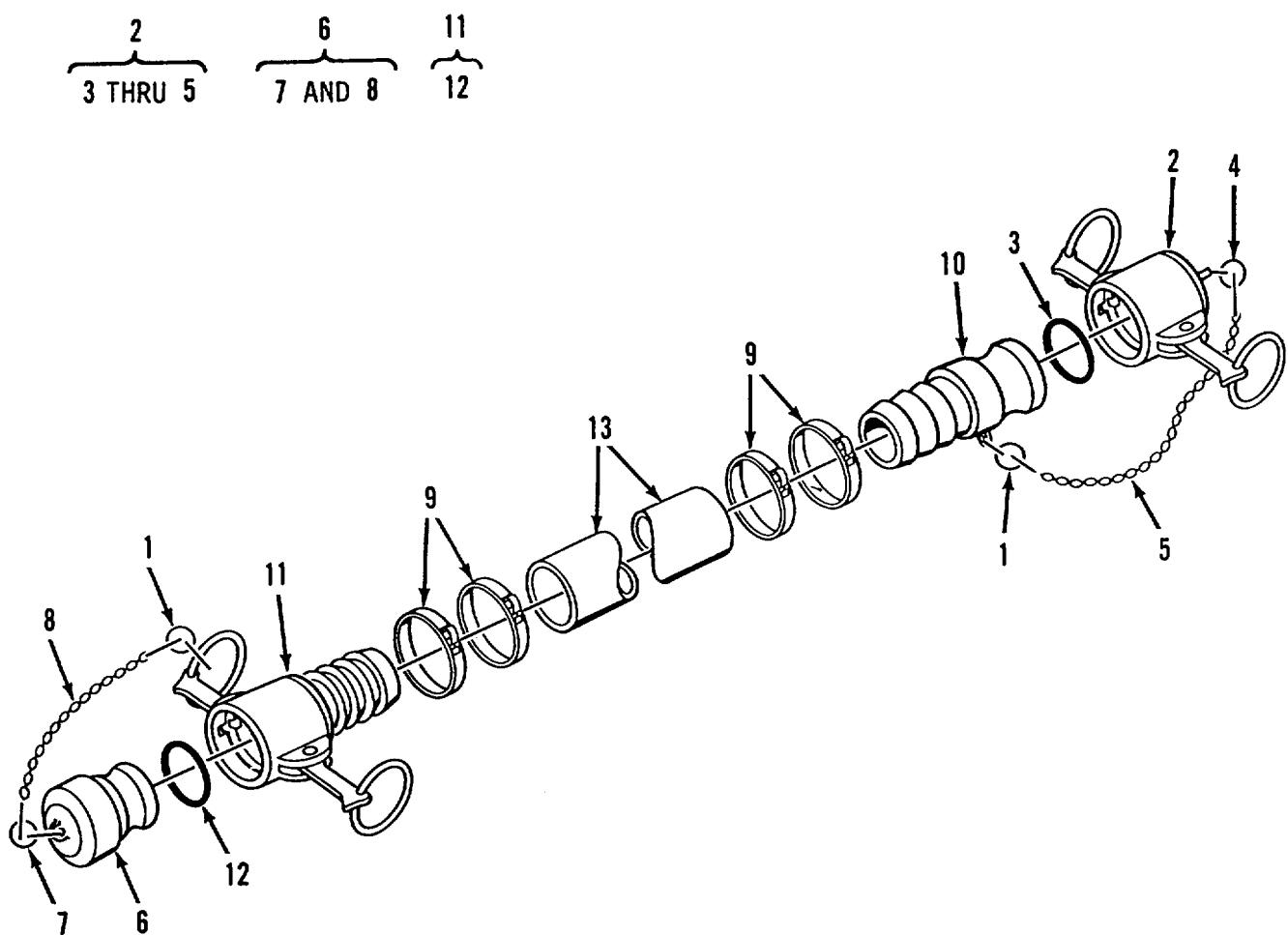
**Figure 47. Hose Assembly, Suction, Potable Water, 2 Inch**
