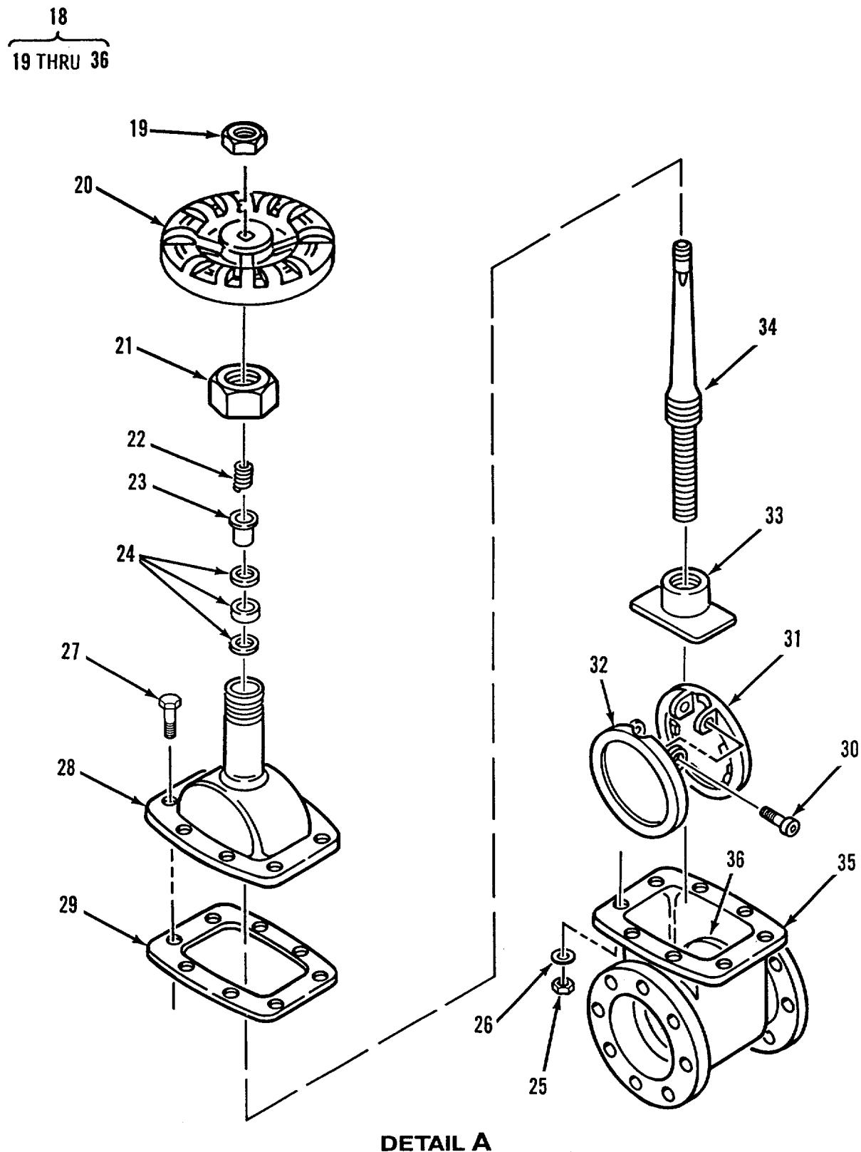
Figure 56. Gate Valve Assembly, 4 Inch (Sheet 2 of 2 )
