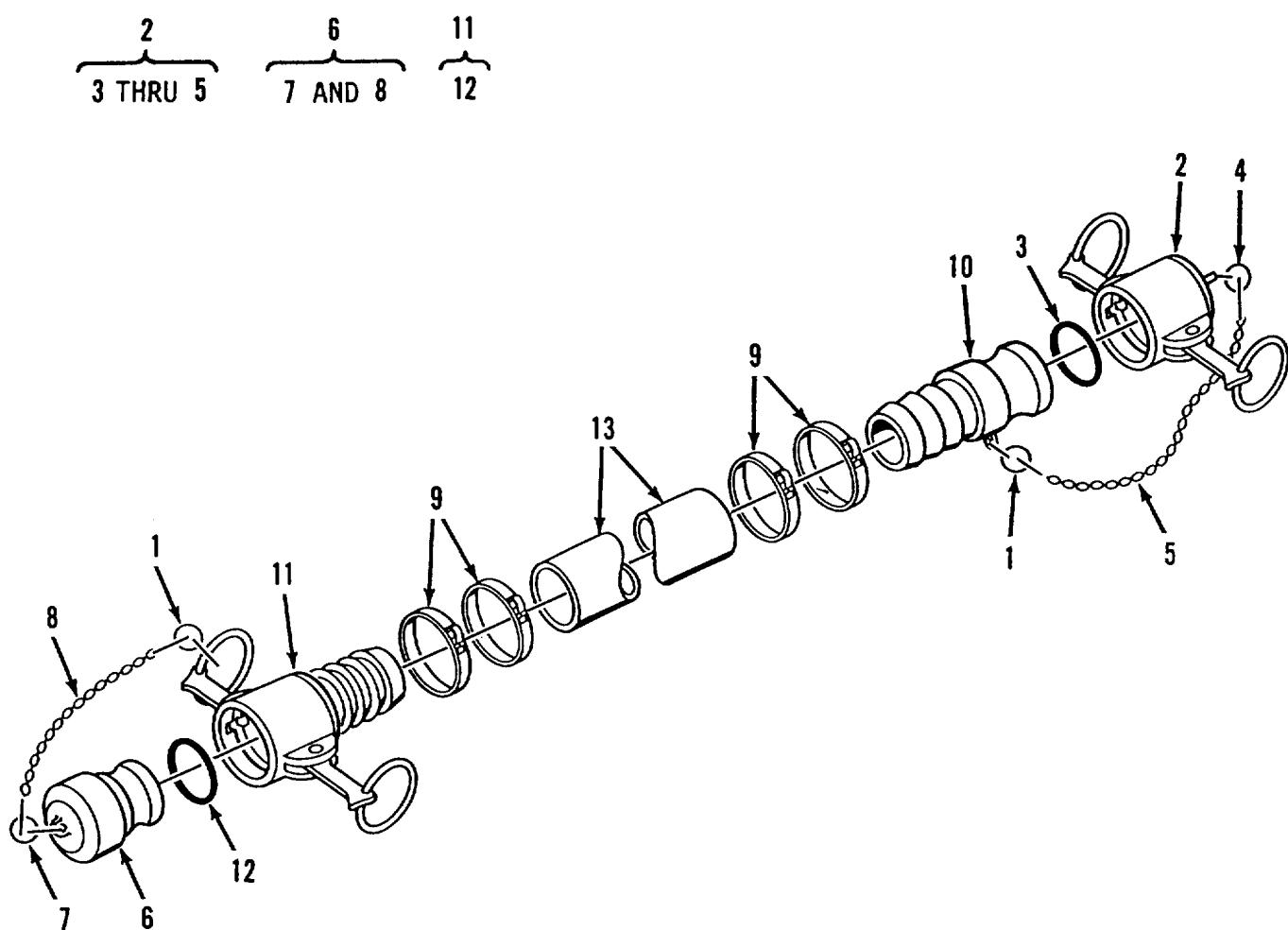
Figure 24. Hose Assembly, Discharge, Potable Water, 4 Inch
