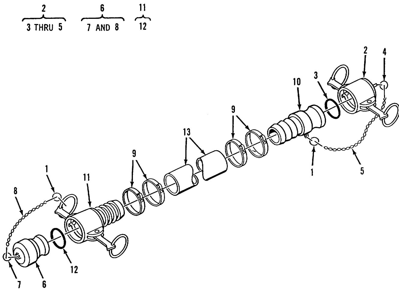
Figure 53. Hose Assembly, Suction, Potable Water, 4 Inch
