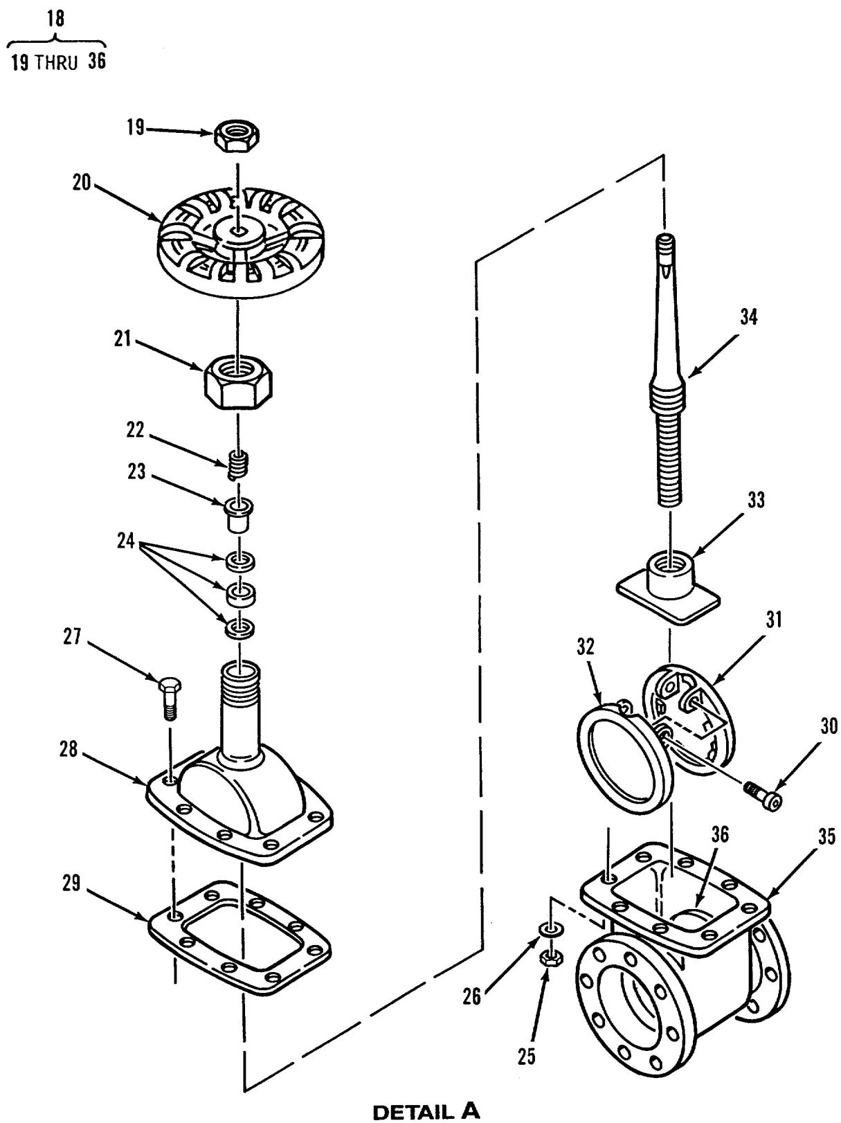
Figure 55. Gate Valve Assembly, 4 Inch (Sheet 2 of 2)
