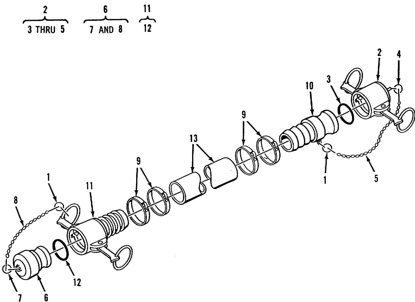
Figure 6. Hose Assembly, Discharge, Potable Water, 4 Inch
