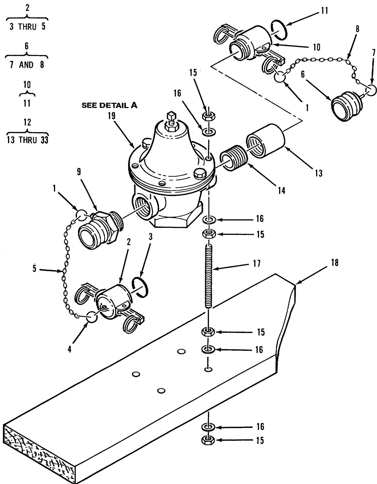
Figure 10. Regulator Assembly, Potable Water (Sheet 1 of 2)
