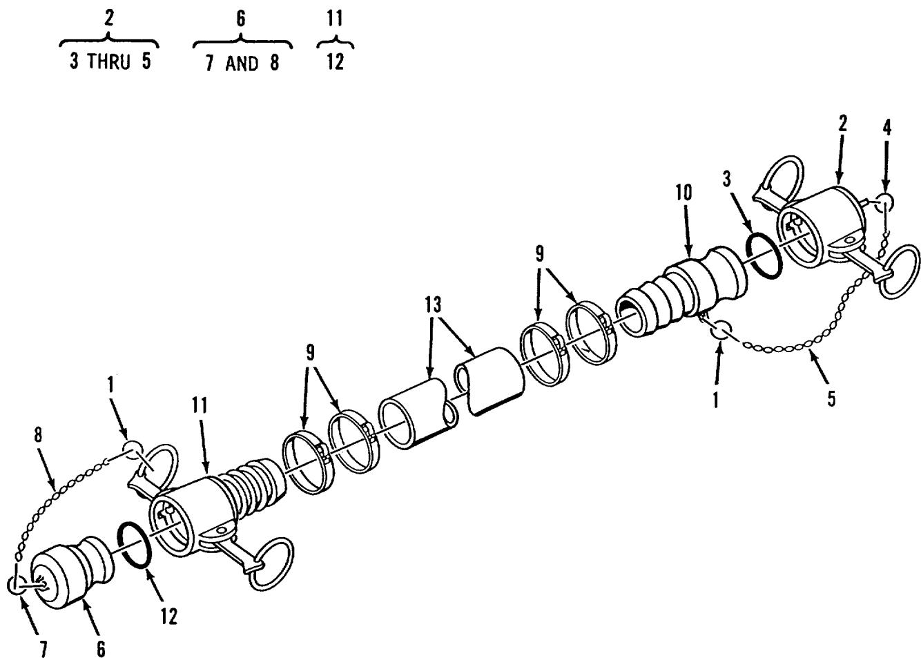
Figure 51. Hose Assembly, Discharge, Potable Water, 4 Inch
