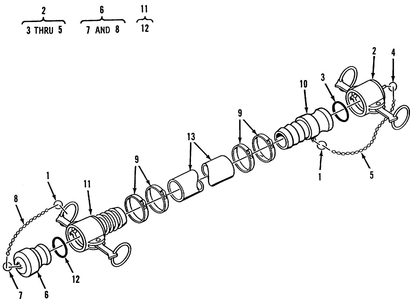
Figure 2. Hose Assembly, Discharge, Potable Water, 1 1/2 inch
