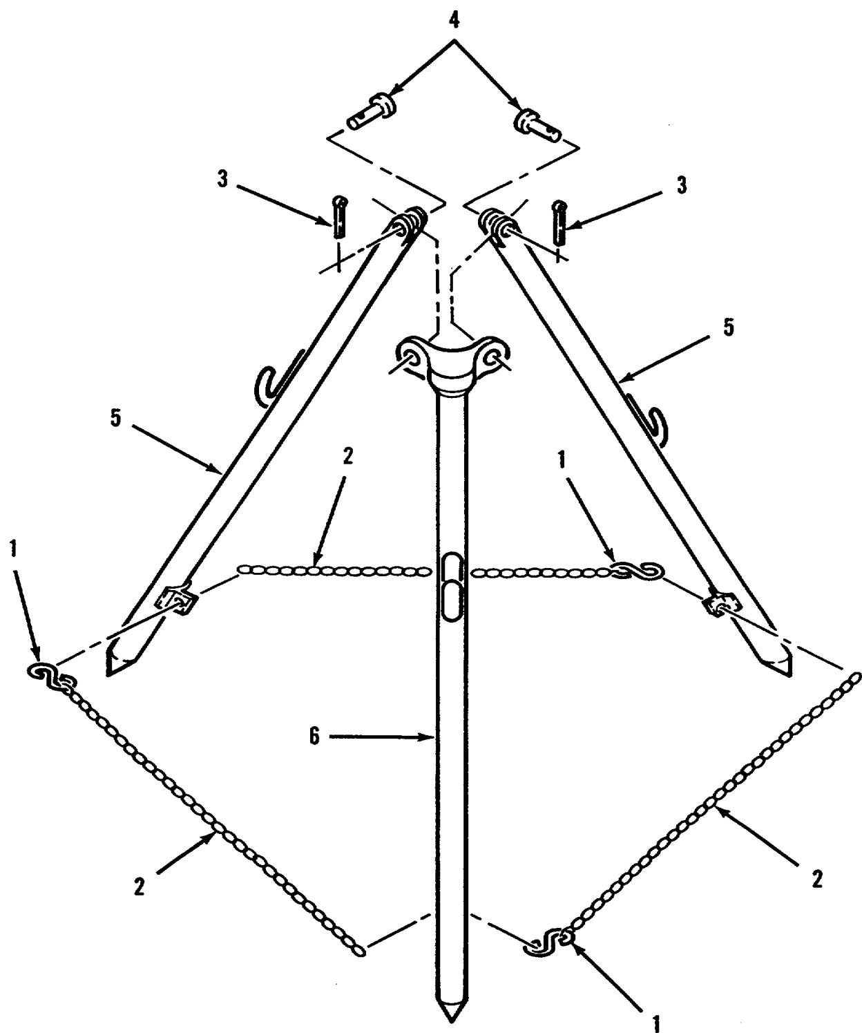
Figure 19. Stand Assembly, Nozzle
