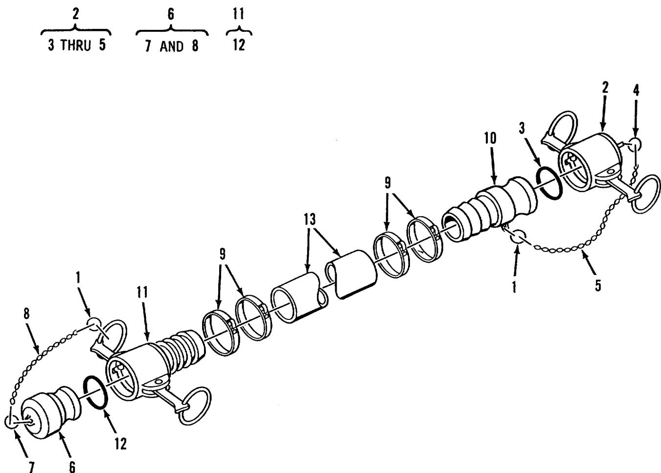
Figure 14. Hose Assembly, Discharge, Potable Water, 1 1/2 Inch
