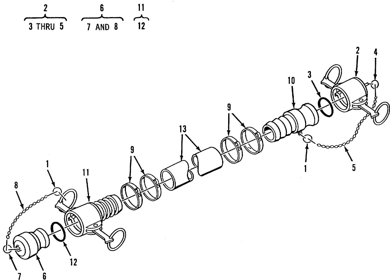
Figure 9. Hose Assembly, Discharge, Potable Water, 1 Inch
