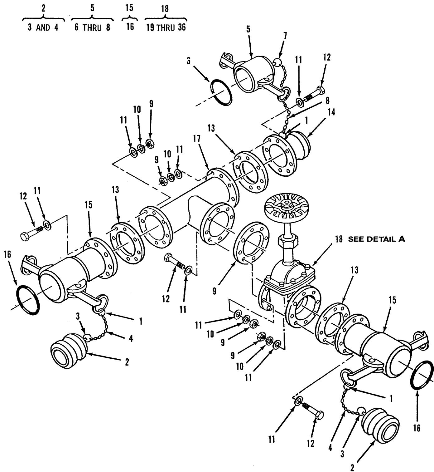
Figure 55. Gate Valve Assembly, 4 Inch (Sheet 1 of 2)
