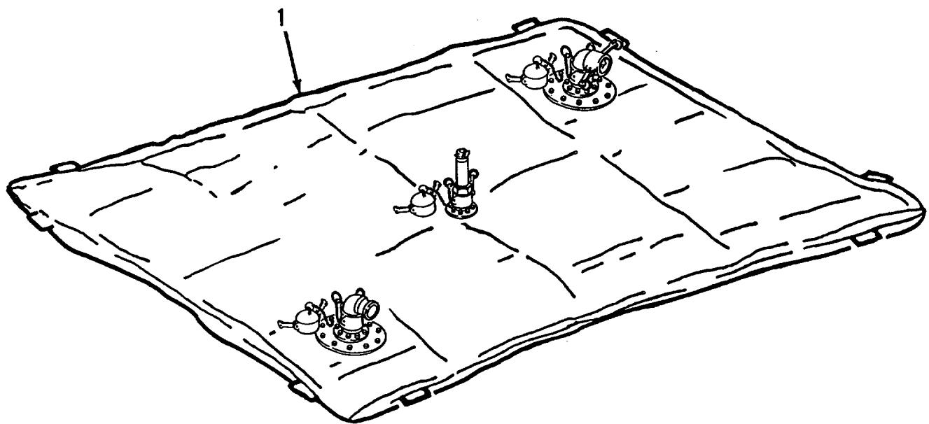
*Figure 62. Collapsible Fabric Tank. 20k Gallon*
