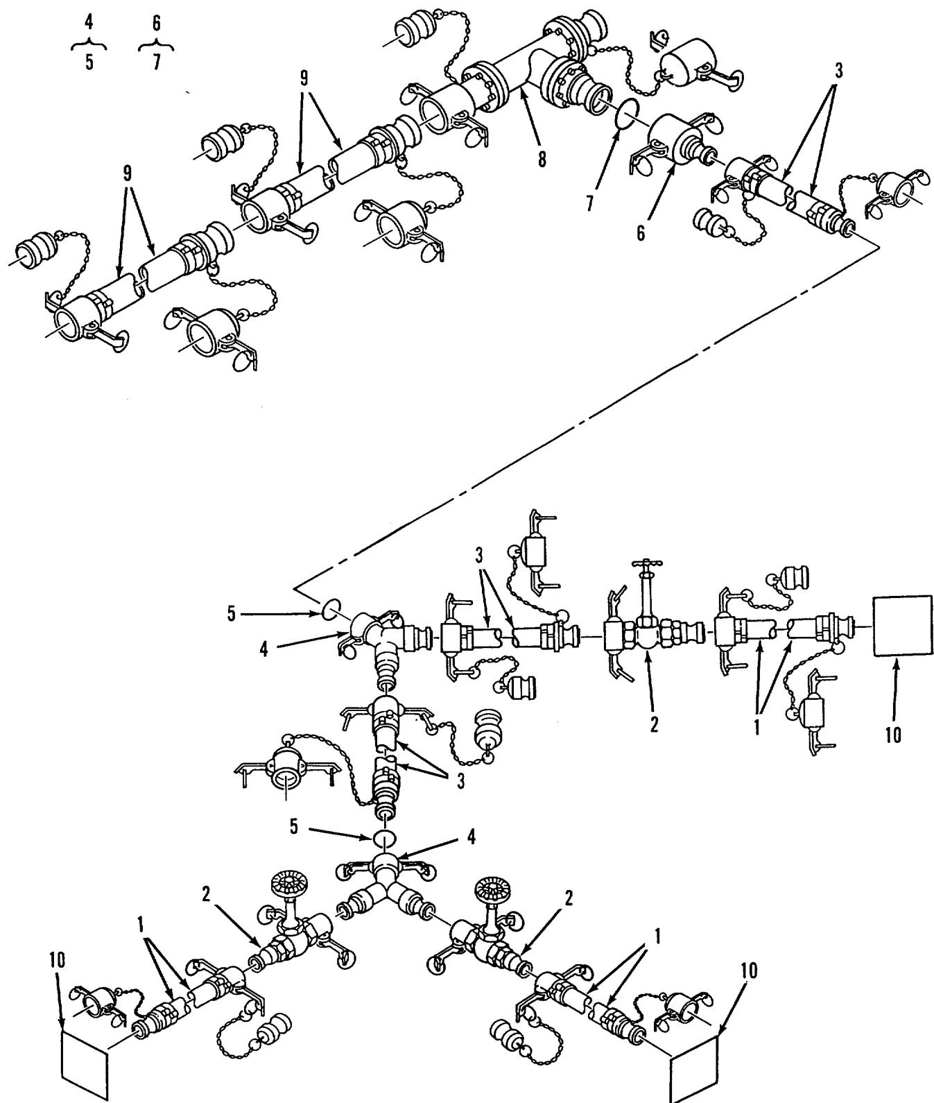
Figure 1. Bag Filler/Hose and Nozzle Connection Kits
