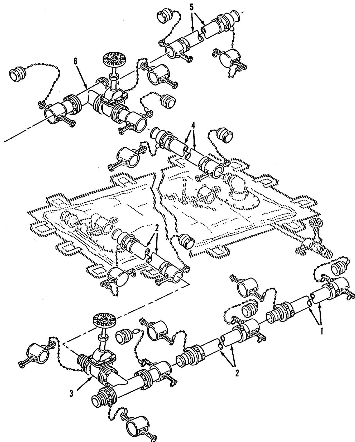
Figure 49. Dual Tank Connection Kit (Sheet 1 of 2)
