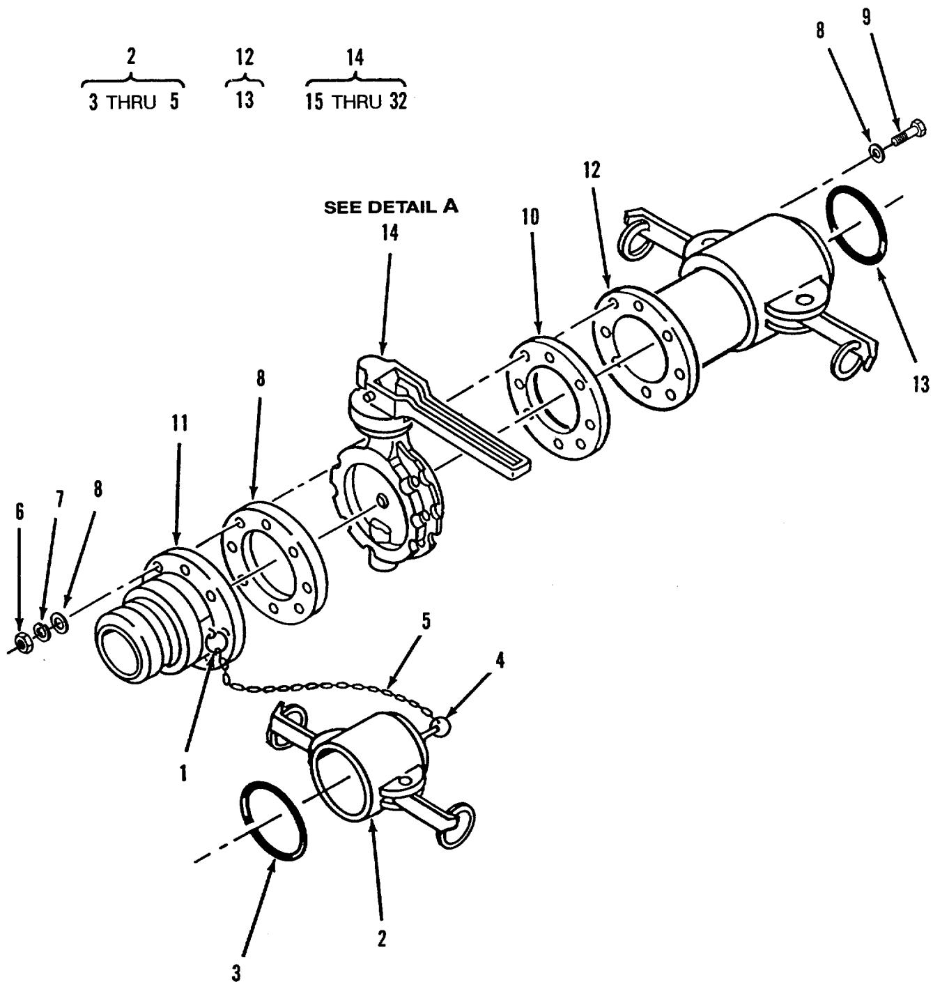
Figure 27. Butterfly Valve Assembly, 4 Inch (Sheet 1 of 2 )
