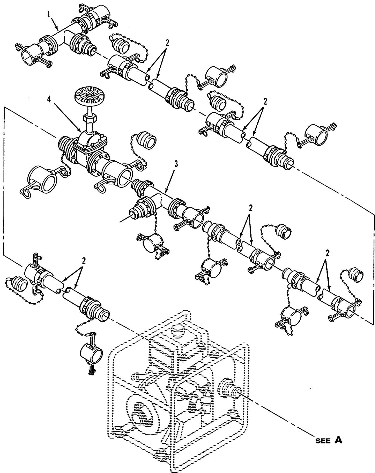
Figure 33. 350 GPM Pump Connection Kit (Sheet 1 of 2)
