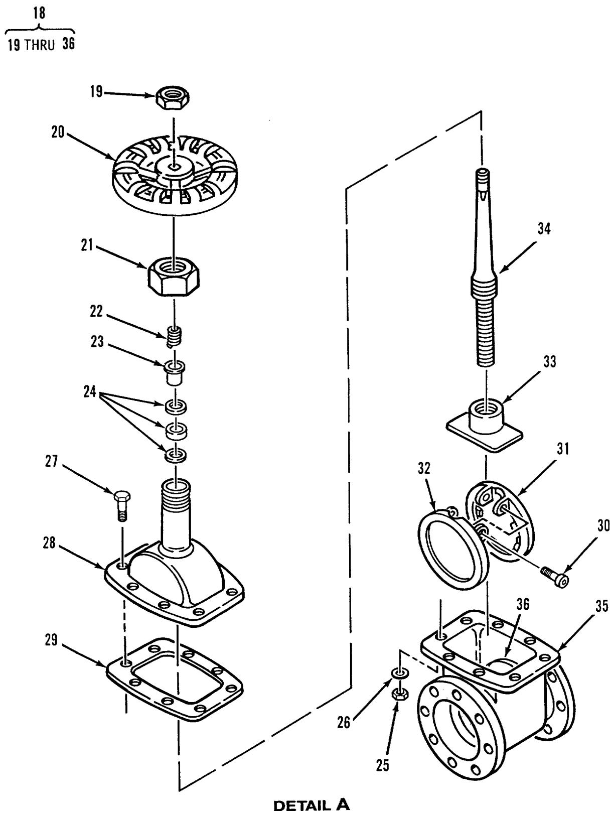
Figure 57. Gate Valve Assembly, 4 Inch (Sheet 2 of 2)
