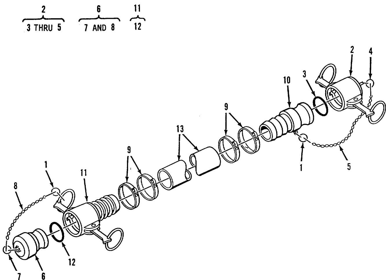
Figure 50. Hose Assembly, Discharge, Potable Water, 4 Inch
