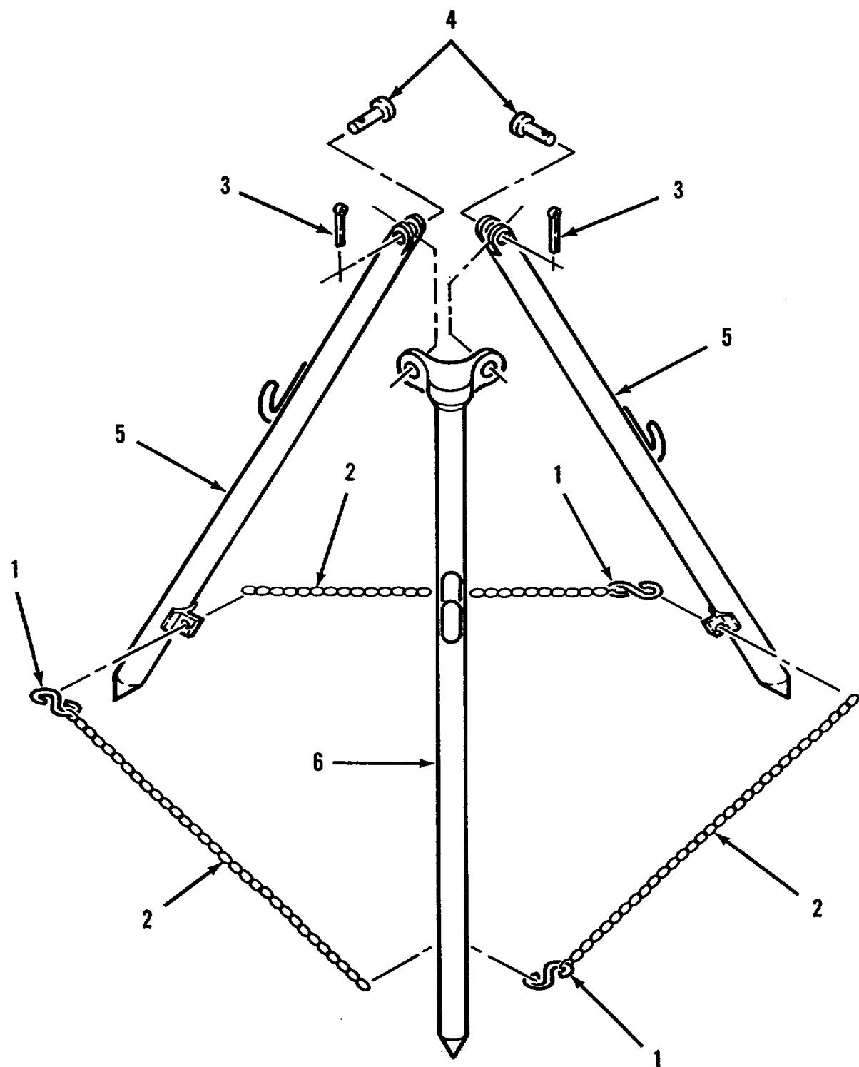
Figure 11. Stand Assembly, Nozzle
