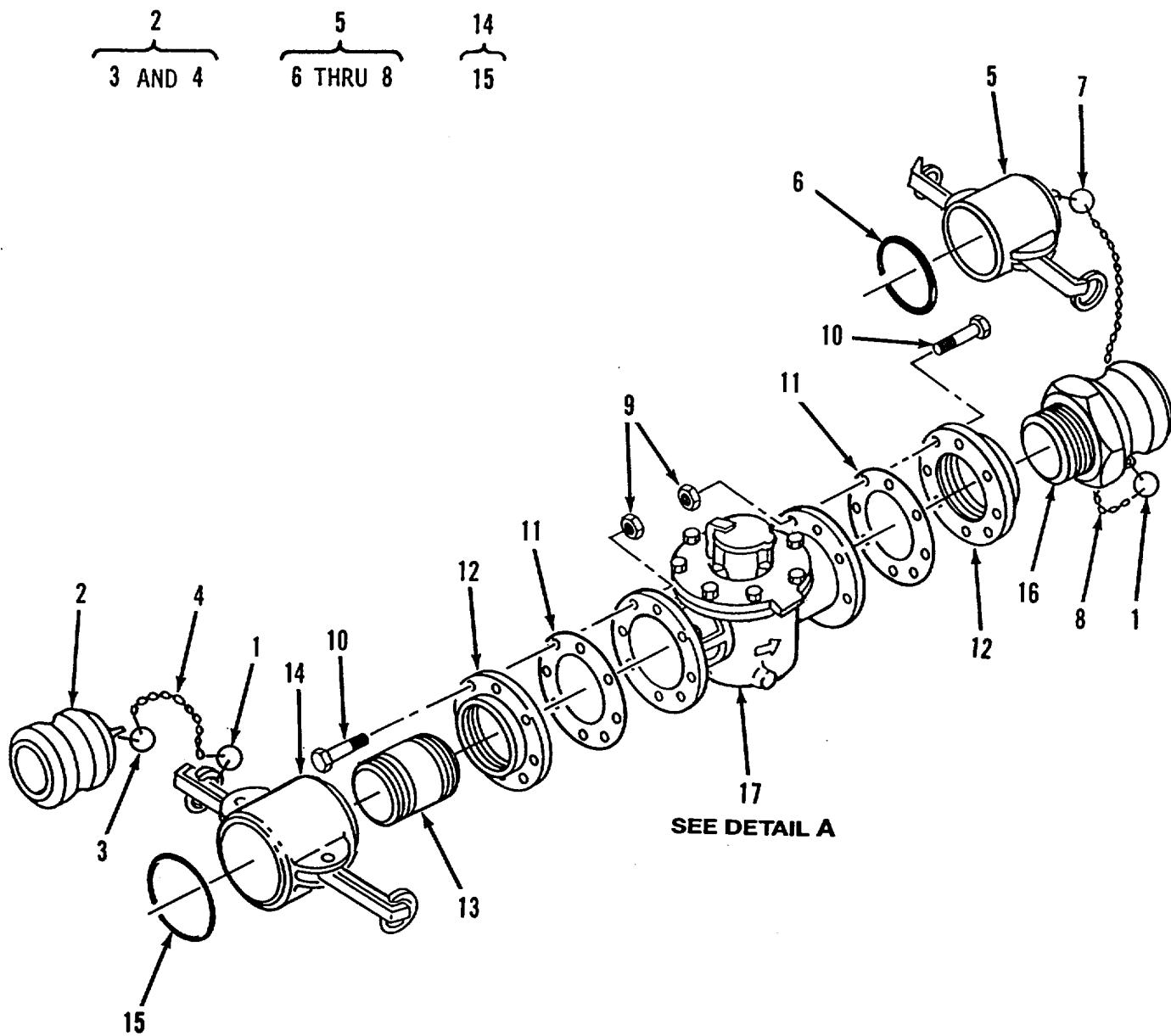
Figure 40. Water Meter Assembly, Fluid Flow Indicating (Sheet 1 of 2 )
