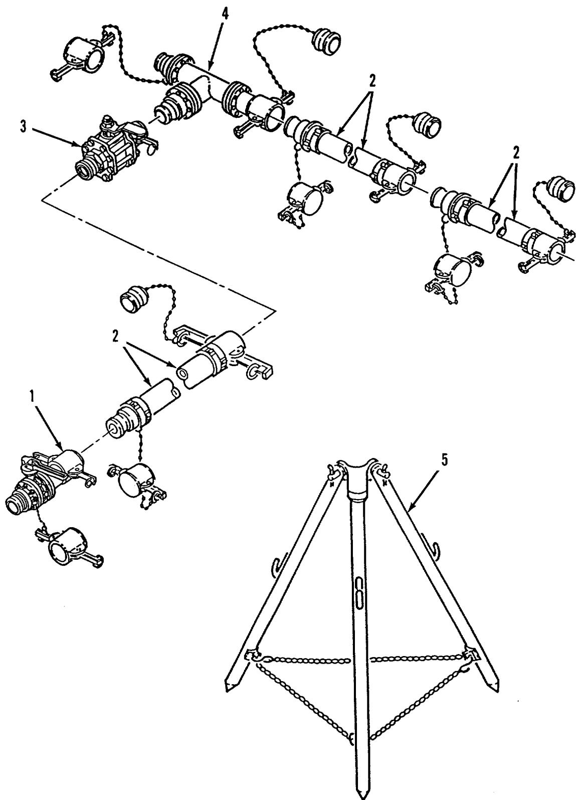
Figure 26. Hose Connection Kit, Potable Water, 4 Inch
