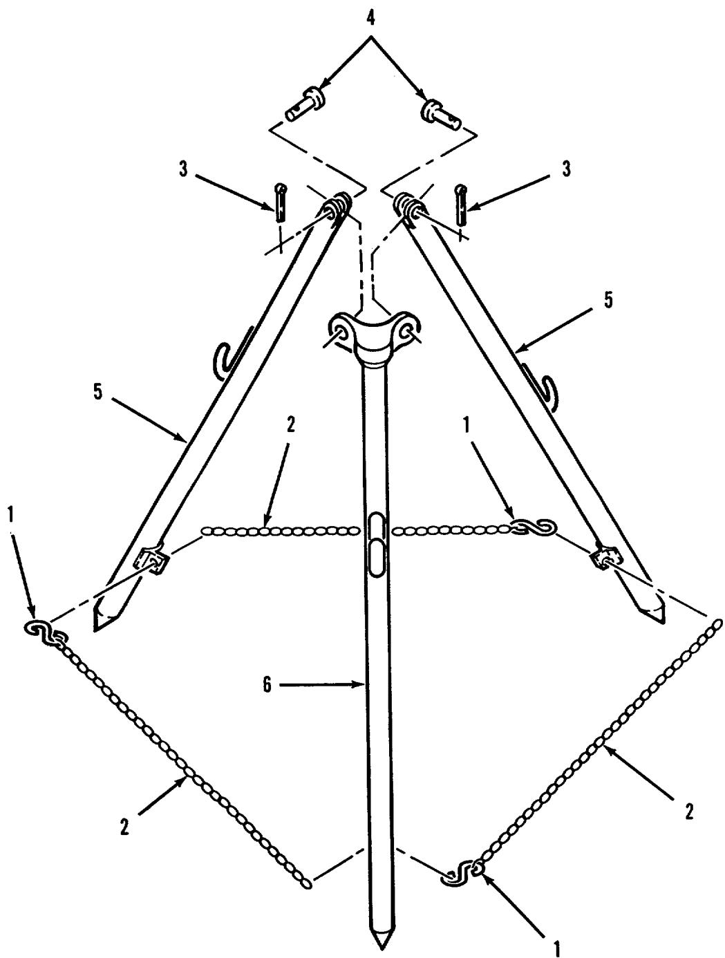
Figure 25. Stand Assembly, Nozzle
