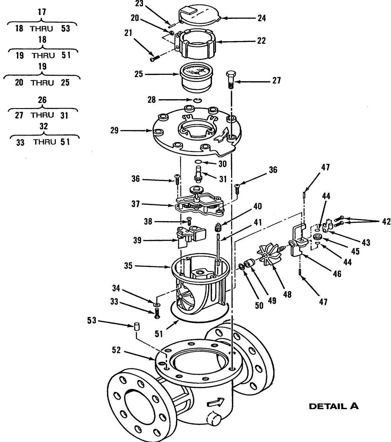
Figure 40. Water Meter Assembly, Fluid Flow Indicating (Sheet 2 of 2 )
