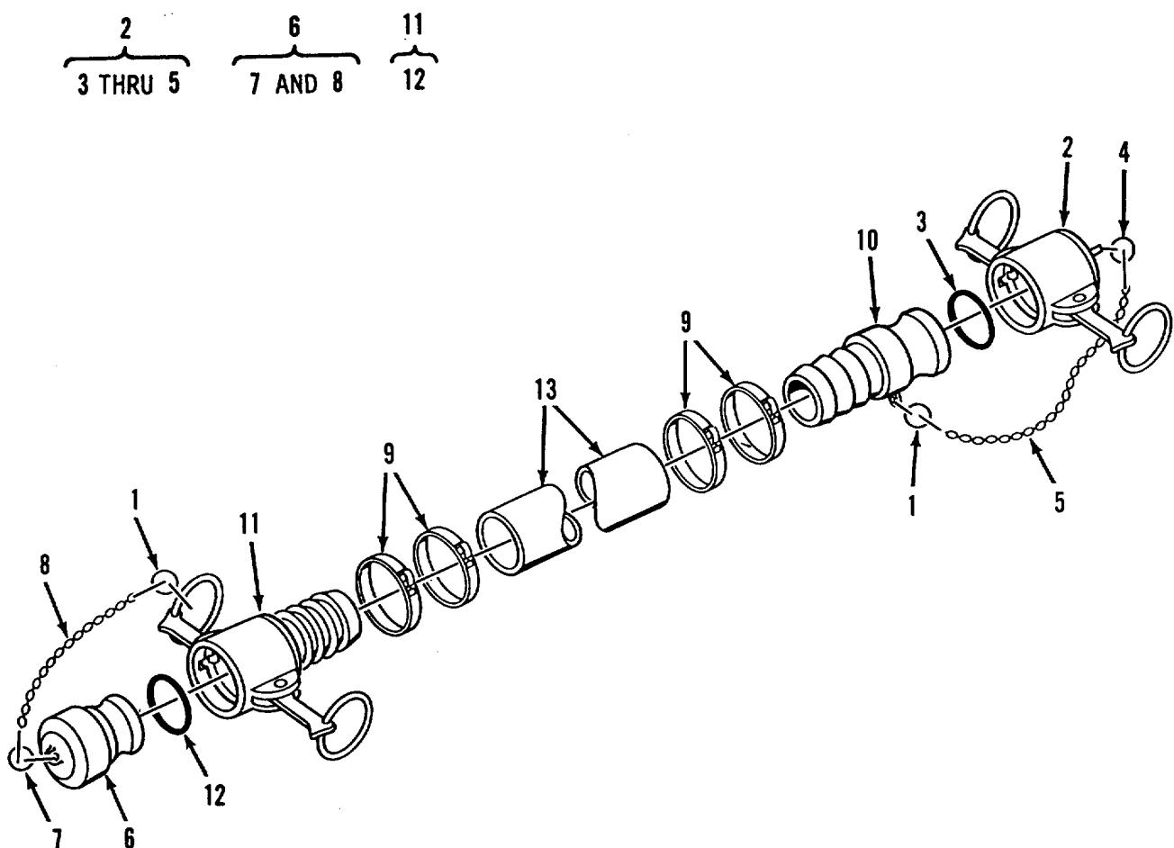
Figure 60. Hose Assembly, Discharge, Potable Water, 4 Inch
