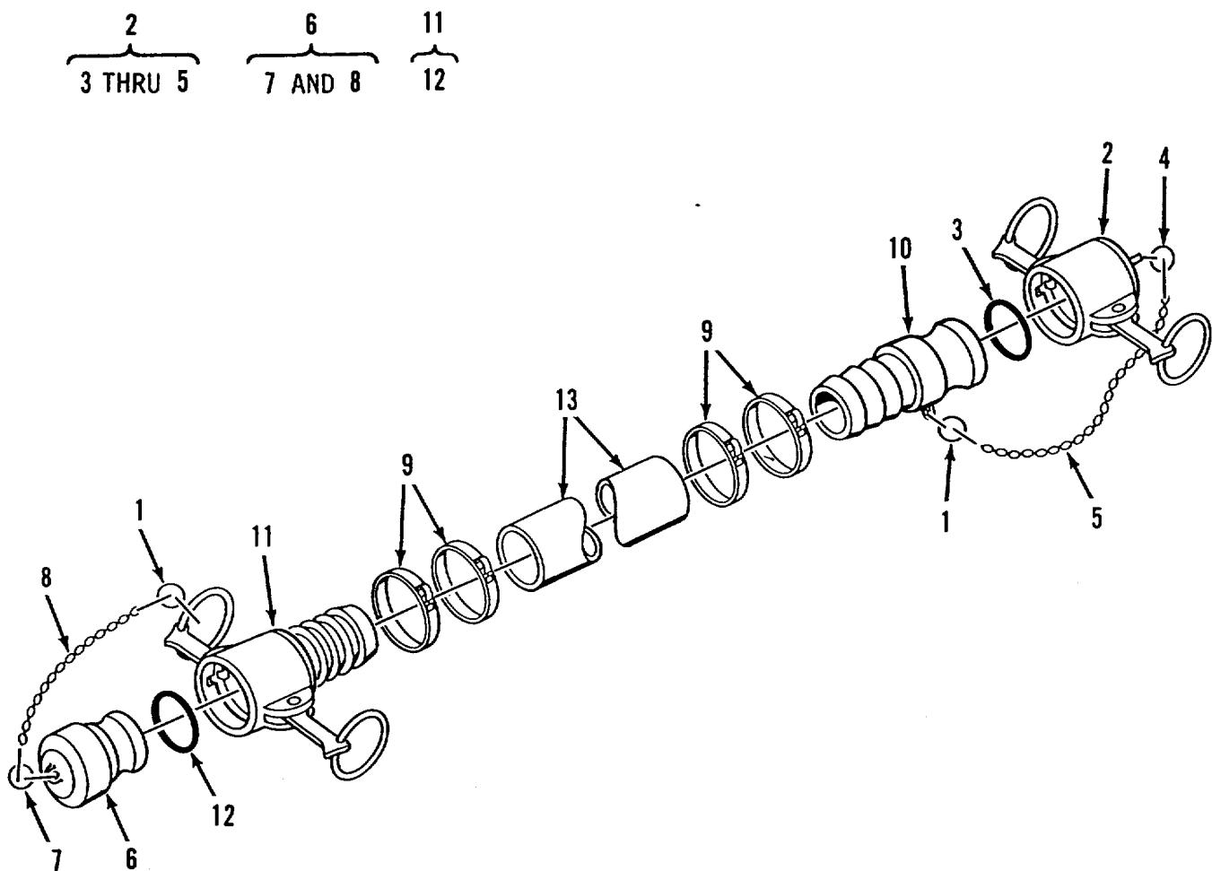
Figure 44. Hose Assembly, Discharge, Potable Water, 2 Inch
