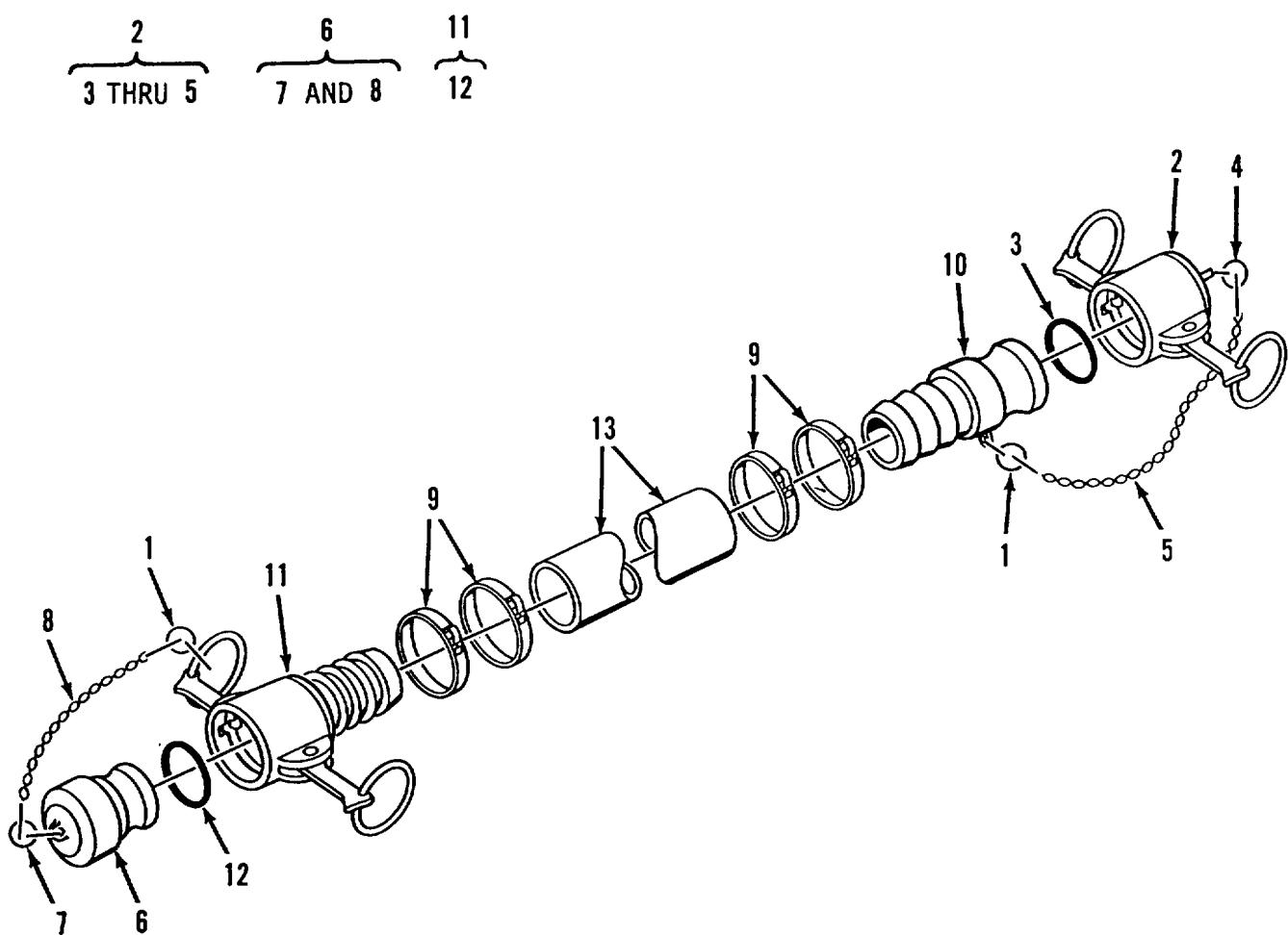
Figure 28. Hose Assembly, Discharge, Potable Water, 4 Inch
