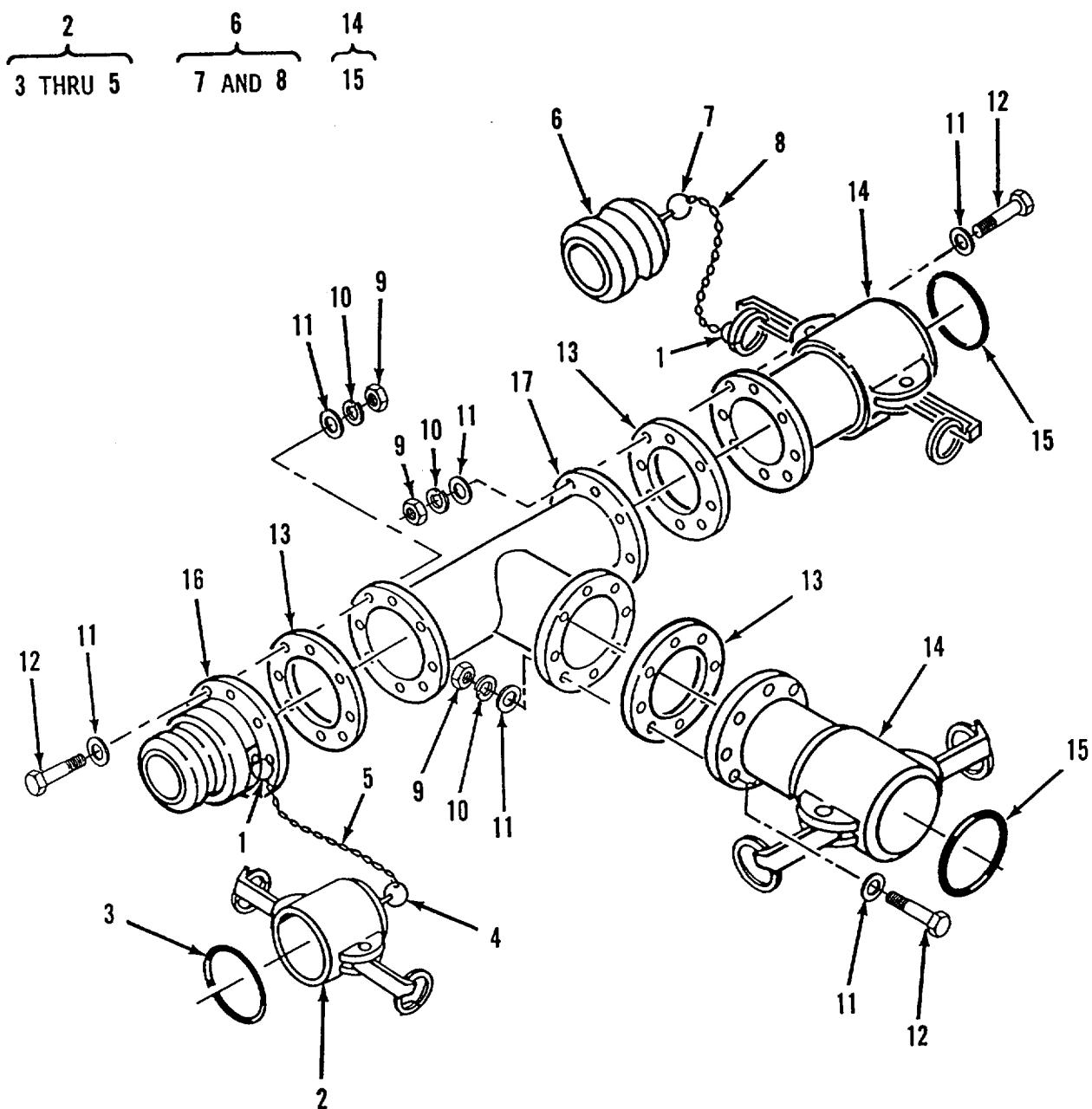
Figure 57. Gate Valve Assembly, 4 Inch (Sheet 1 of 2)
