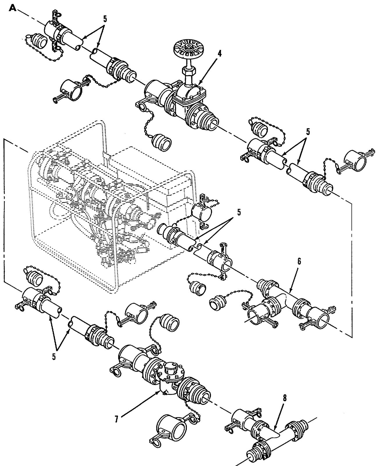
Figure 33. 350 GPM Pump Connection Kit (Sheet 2 of 2)
