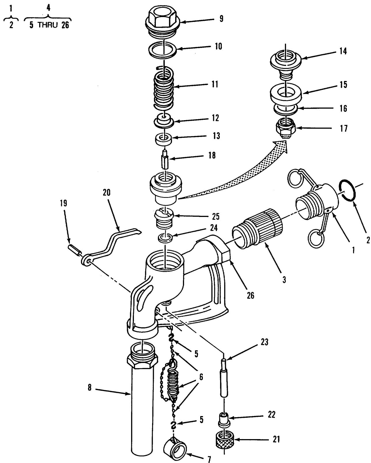
Figure 13. Nozzle Assembly, 1 1/2 Inch
