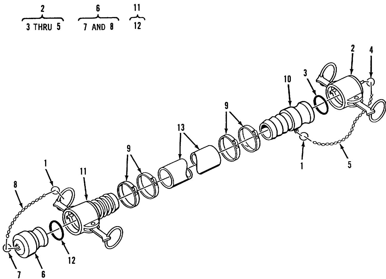
Figure 38. Hose Assembly, Discharge, Potable Water, 4 Inch
