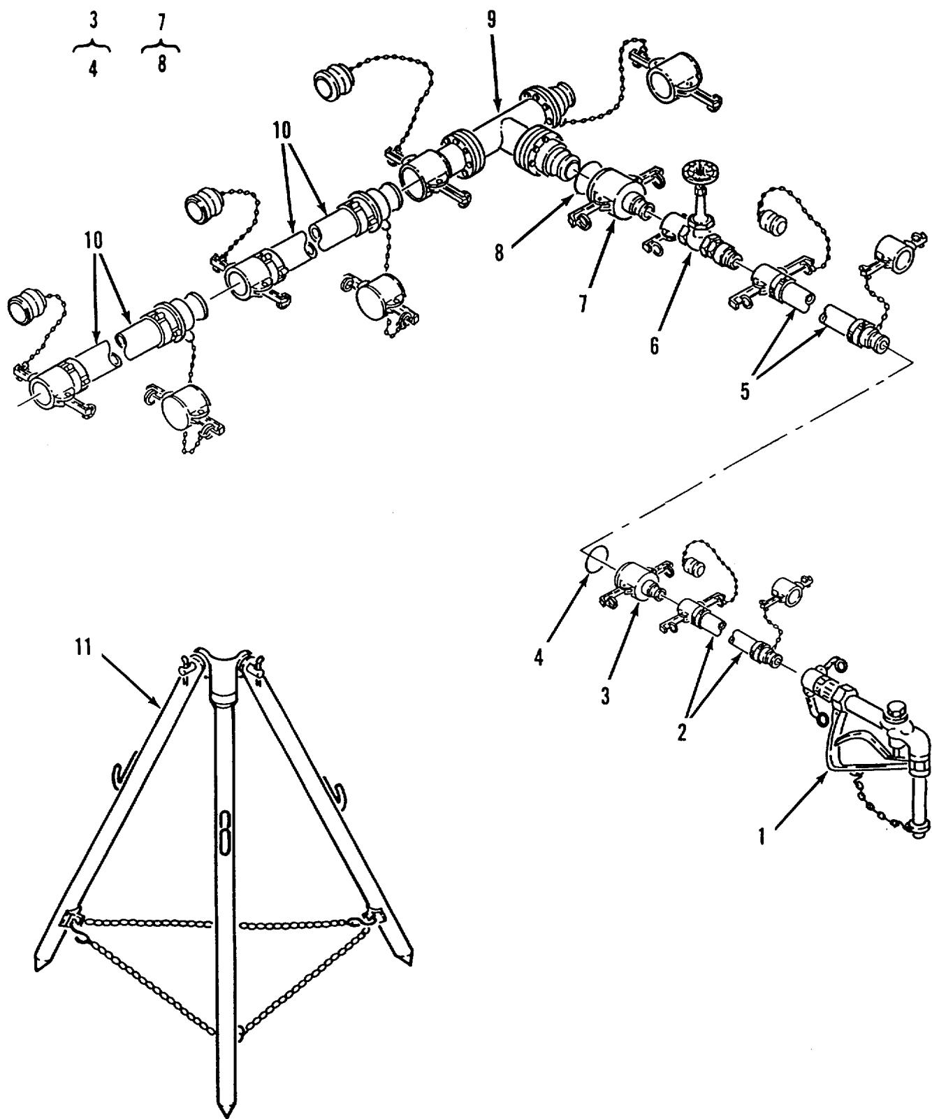
Figure 12. Hose Nozzle Connection Kit, Potable Water
