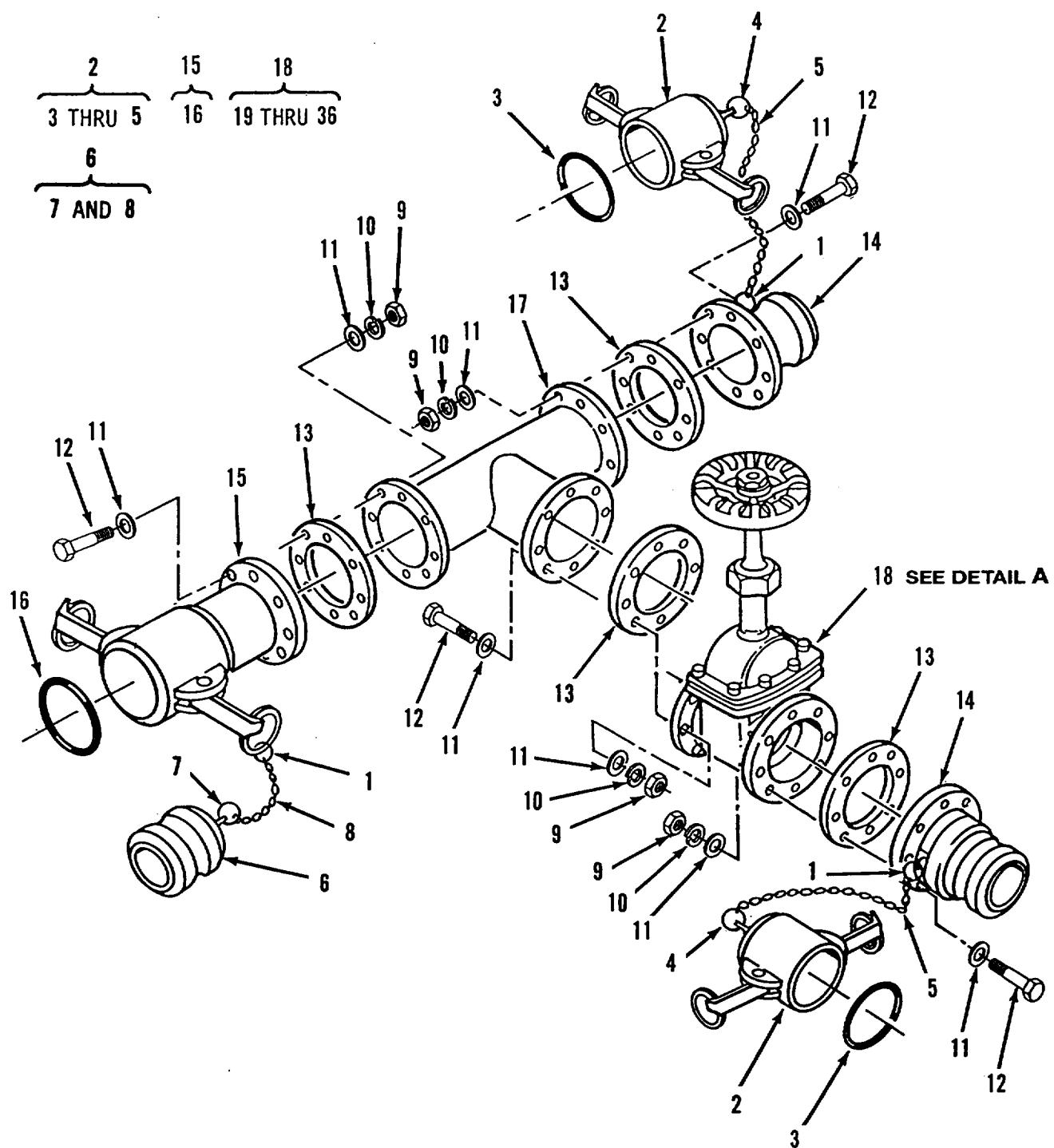
Figure 52. Gate Valve Assembly, 4 Inch (Sheet 1 of 2)
