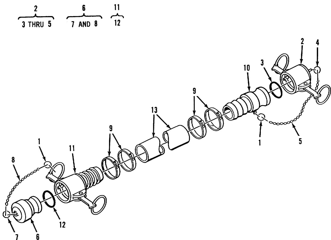
Figure 15. Hose Assembly, Discharge, Potable Water, 2 Inch
