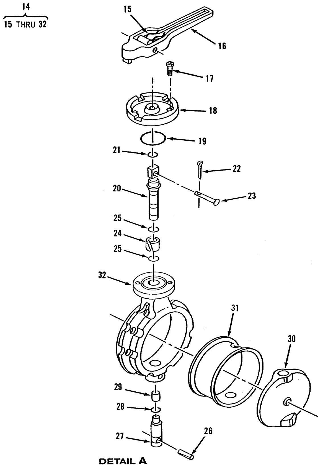
Figure 27. Butterfly Valve Assembly, 4 Inch (Sheet 2 of 2 )
