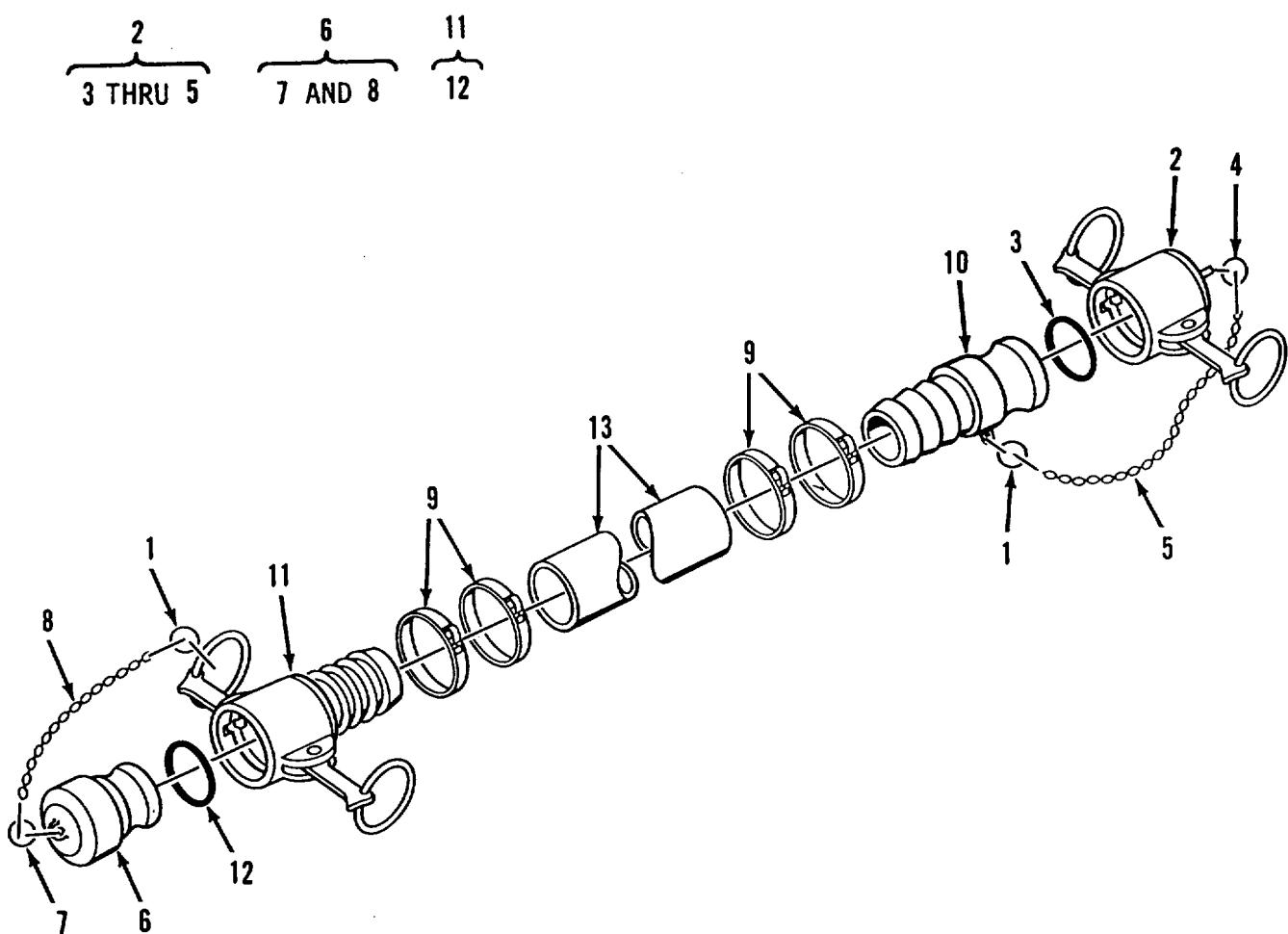
Figure 35. Hose Assembly, Suction, Potable Water, 4 Inch
