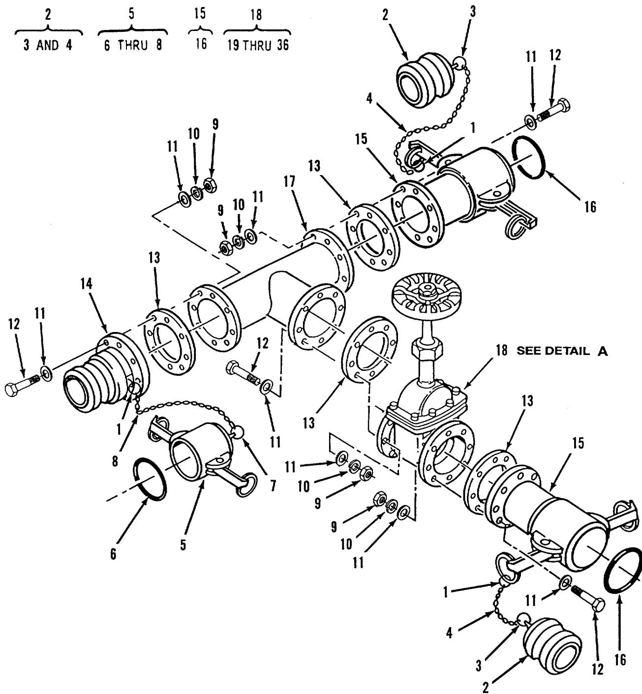
Figure 56. Gate Valve Assembly, 4 Inch (Sheet 1 of 2)
