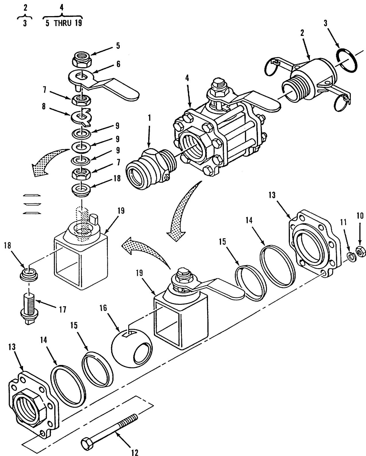
Figure 29. Quick Acting Valve Assembly, 4 Inch
