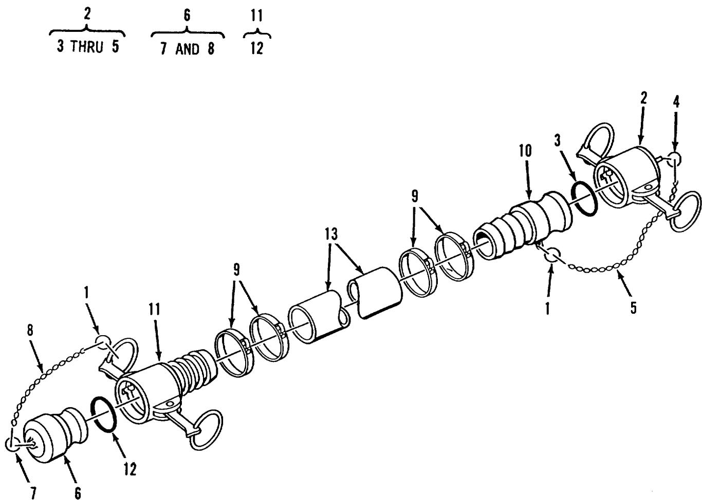
Figure 18. Hose Assembly, Discharge, Potable Water, 4 Inch
