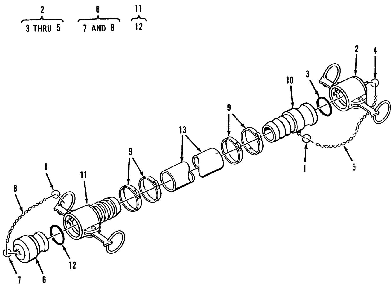
Figure 21. Hose Assembly, Discharge, Potable Water, 2 Inch
