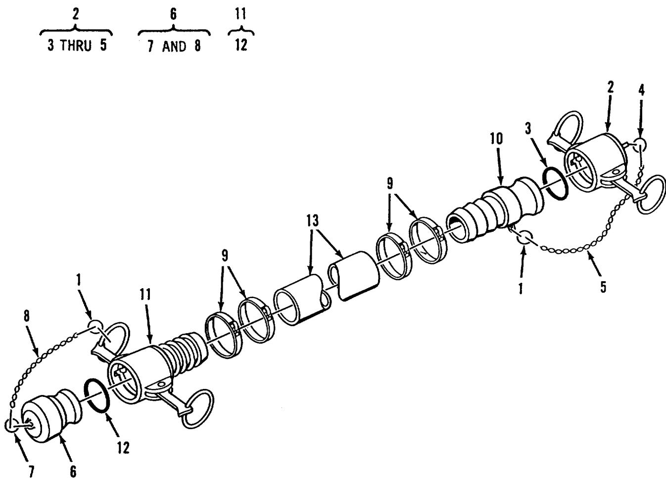
Figure 4. Hose Assembly, Discharge, Potable Water, 2 Inch
