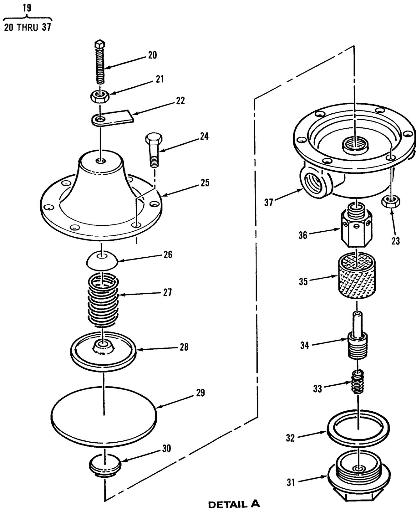
Figure 10. Regulator Assembly, Potable Water (Sheet 2 of 2)
