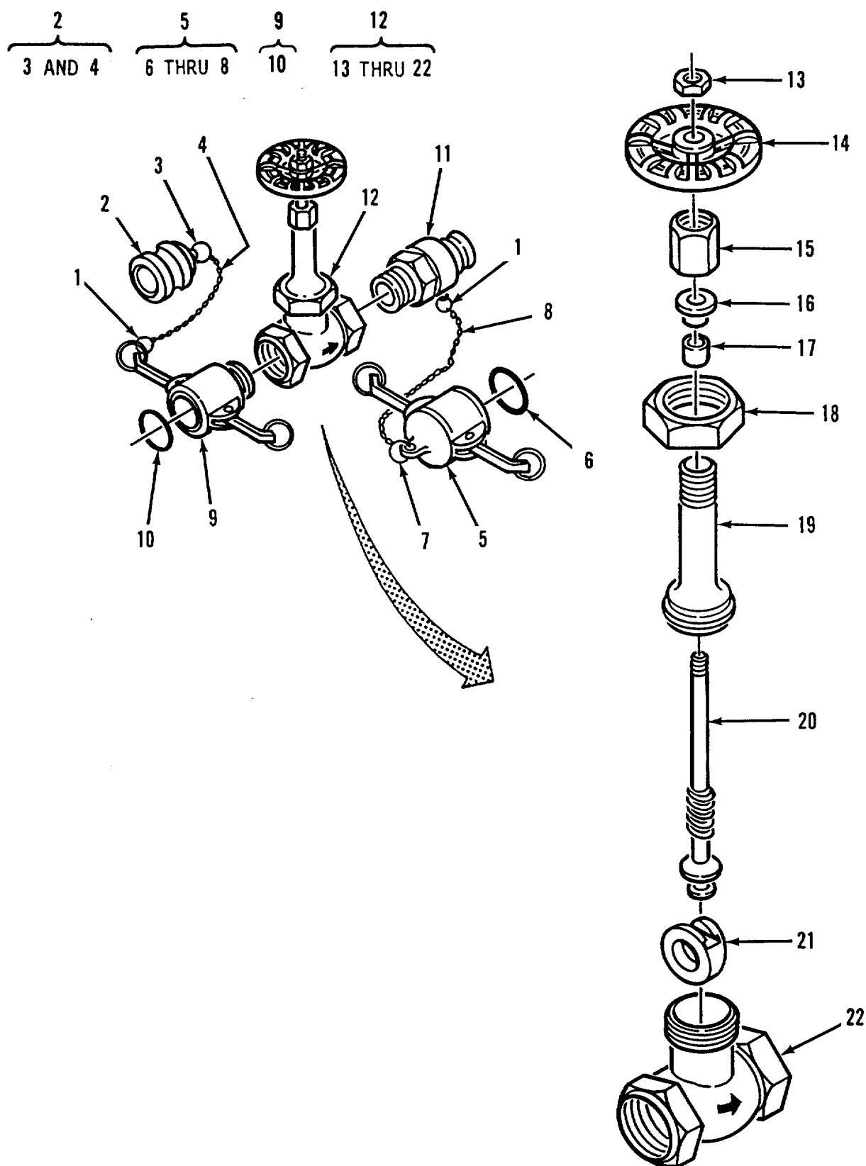
Figure 45. Gate Valve Assembly, 2 Inch
