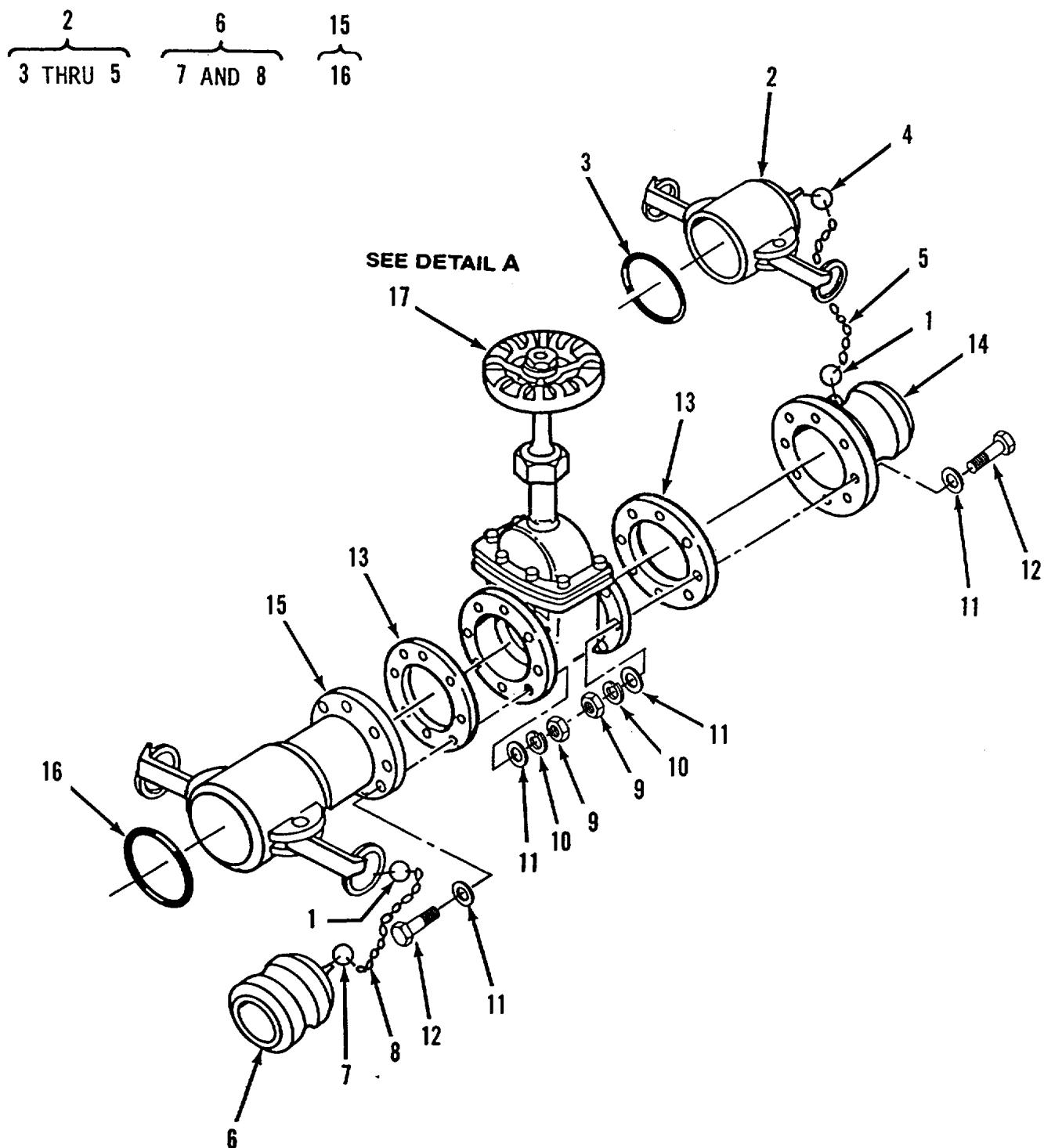
Figure 37. Gate Valve Assembly, 4 Inch (Sheet 1 of 2)
