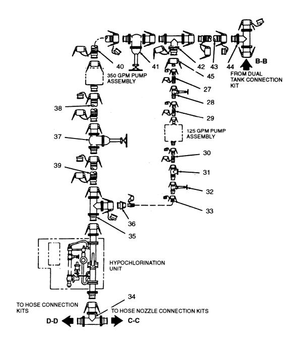
350 and 125 GPM Pump Connection Kits
