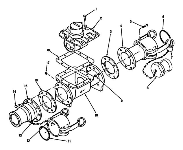
Water Meter Assembly (Model WSDS40K)
