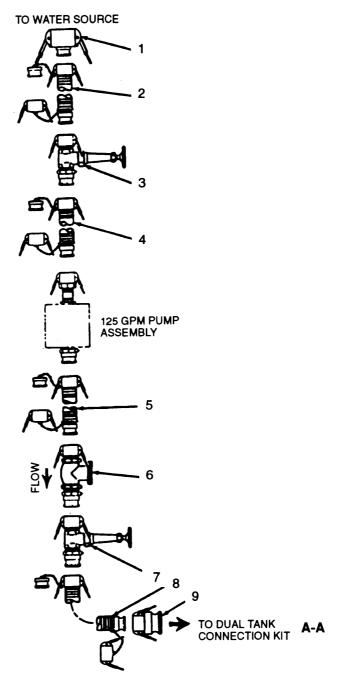
c. Dual Tank Connection Kit Assembly. Assemble dual tank connection kit as follows:
