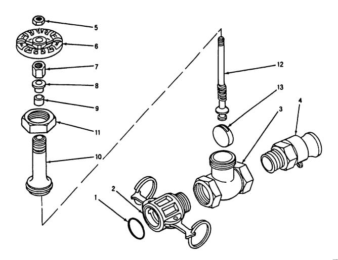
Gate Valve Assembly (2-inch) (Models WSDS40K & 40KWSDS)
