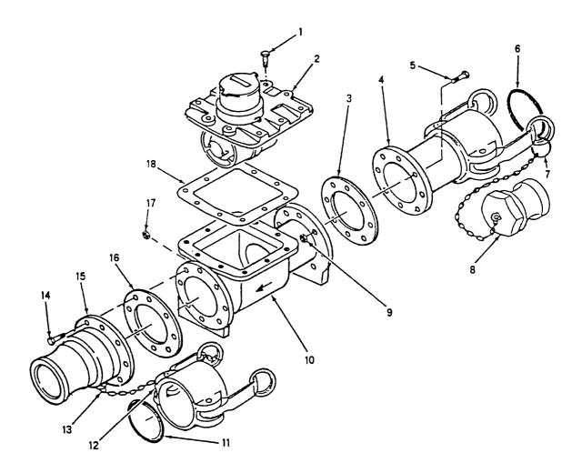
Water Meter Assembly (Model WSDS40K)
