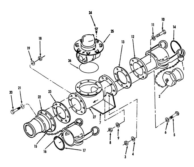
Water Meter Assembly (Model 40KWSDS)
